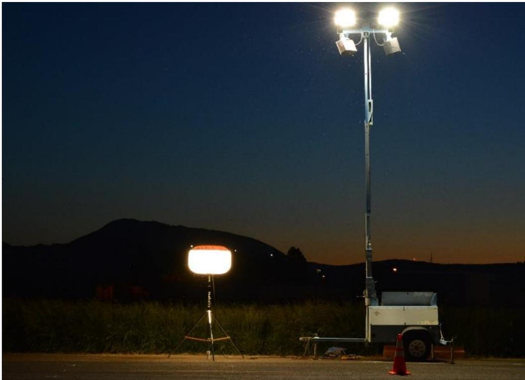
*Figure 3.1 Lighting equipment tested: balloon light (left) and light tower (right).*
