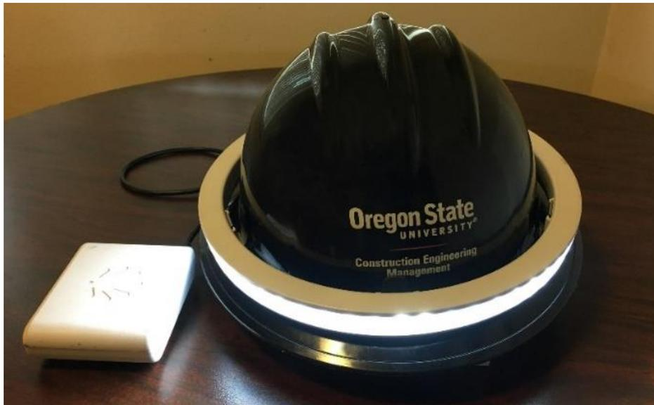
*Figure 3.2 Personal wearable light (Halo Light by Illumagear) attached to hardhat.*
