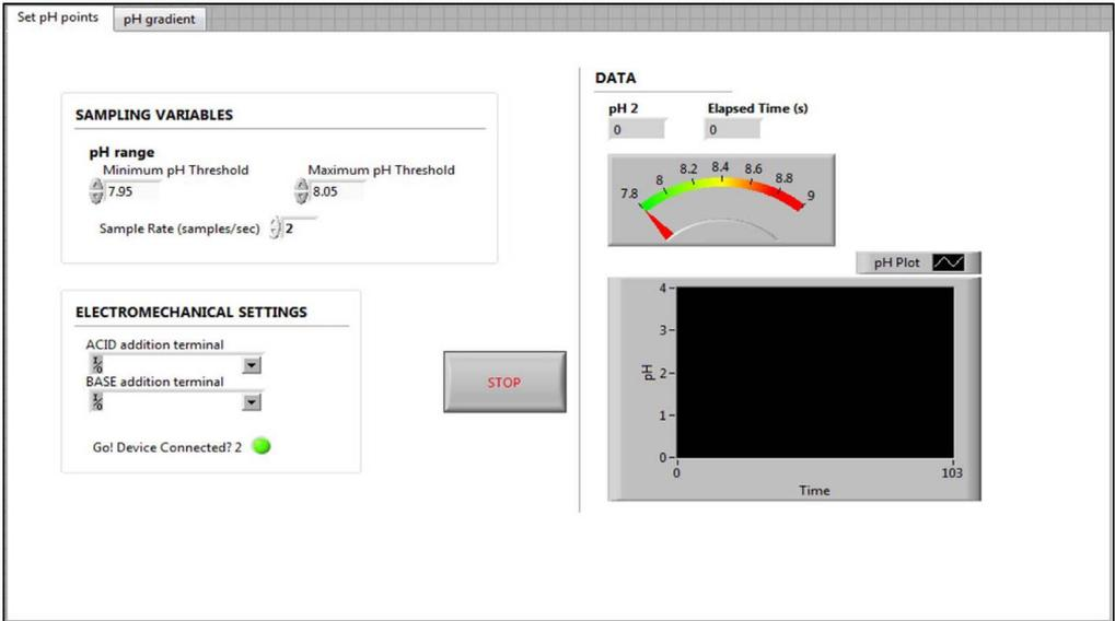
Fig. 1. Front panel of virtual instrument (VI) for producing a steady state pH environment.
