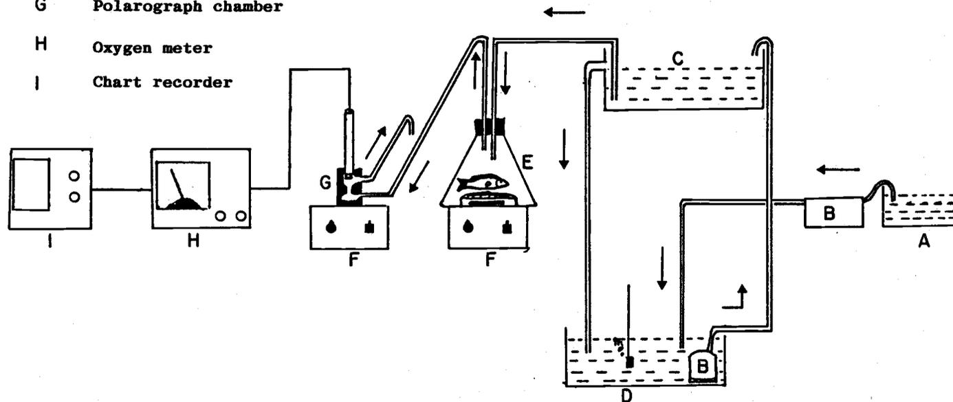
Figure 2. Diagram of the respirometry system. Arrows indicate the direction of water flow.
