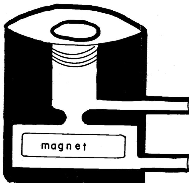
Figure 3. Polarograph chamber
