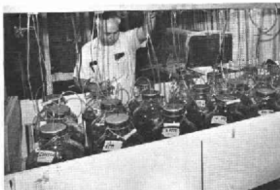
Static water bioassay set up for determining lethal concentrations of 2,4-D to young salmon.
