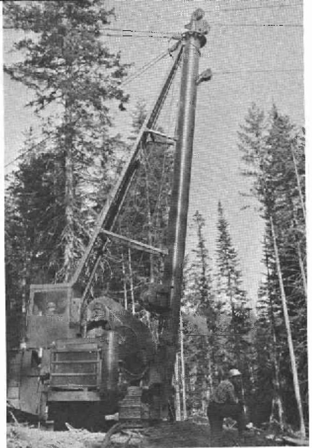
A new mobile running skyline yarder developed from Station Engineering Research.
