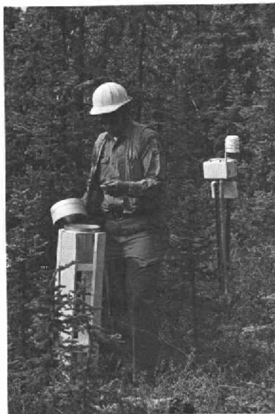
A rain gage in foreground and an automatic soil temperature recorder produce data used in analyzing environmental influences on spruce productivity.
