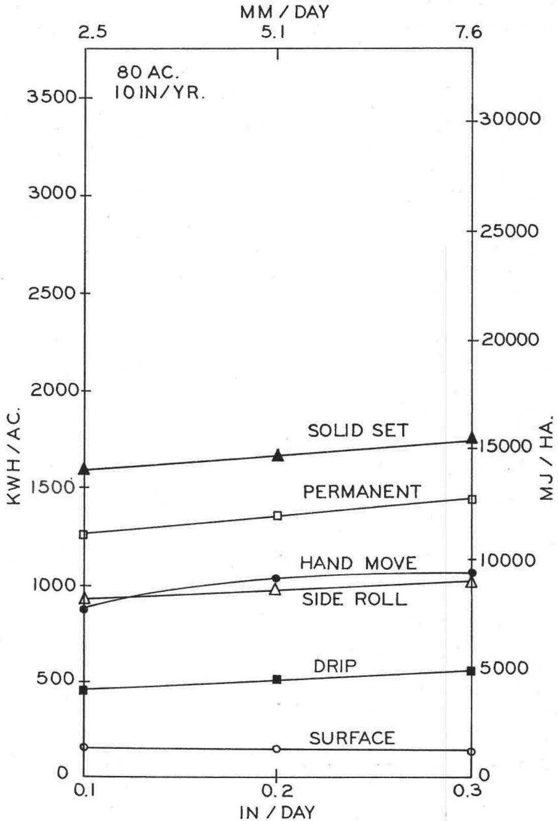
Figure 5. Plot of total seasonal energy as a function of consumptive use rate for a 10 inch (254 mm) seasonal application on a 80 acre (32.4 ha.) field.
