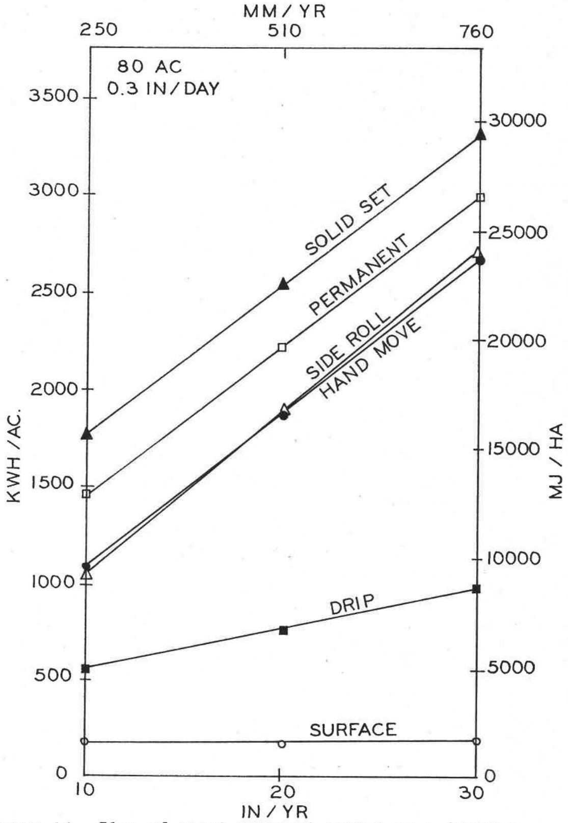
Figure 16. Plot of total seasonal energy as a function of seasonal application on a 80 acre (32.4 ha.) field with a consumptive use rate of 0.3 inch (7.6 mm) per day.
