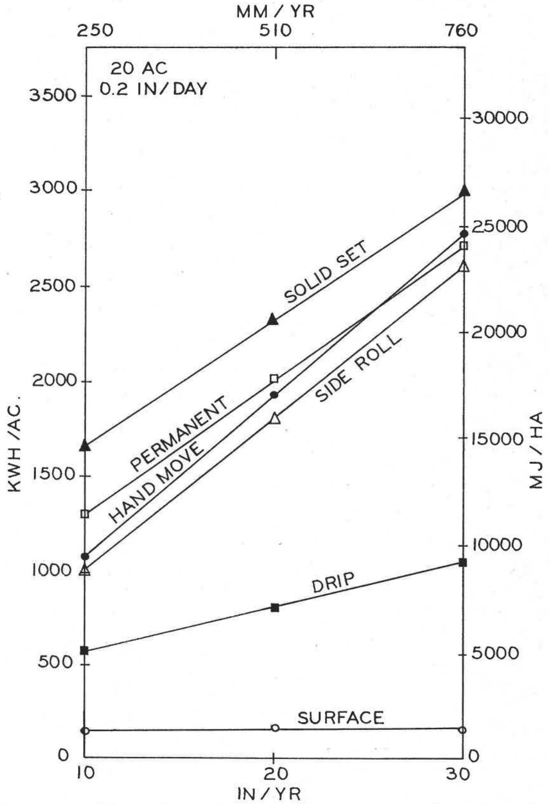
Figure 12. Plot of total seasonal energy as a function of seasonal application on a 20 acre (8.1 ha.) field with a consumptive use rate of 0.2 inch (5.1 mm) per day.
