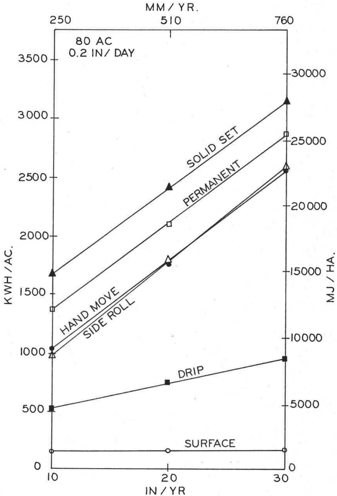
Figure 15. Plot of total seasonal energy as a function of seasonal application on a 80 acre (32.4 ha.) field with a consumptive use rate of 0.2 inch (5.1 mm) per day.
