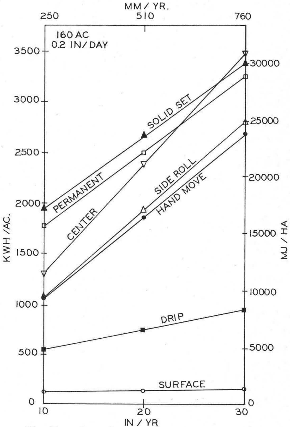
Figure 18. Plot of total seasonal energy as a function of seasonal application on a 160 acre (64.8 ha.) field with a consumptive use rate of 0.2 inch (5.1 mm) per day.
