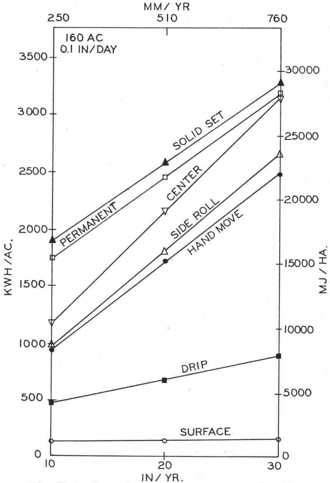
Figure 17. Plot of total seasonal energy as a function of seasonal application on a 160 acre (64.8 ha.) field with a consumptive use rate of 0.1 inch (2.5 mm) per day.
