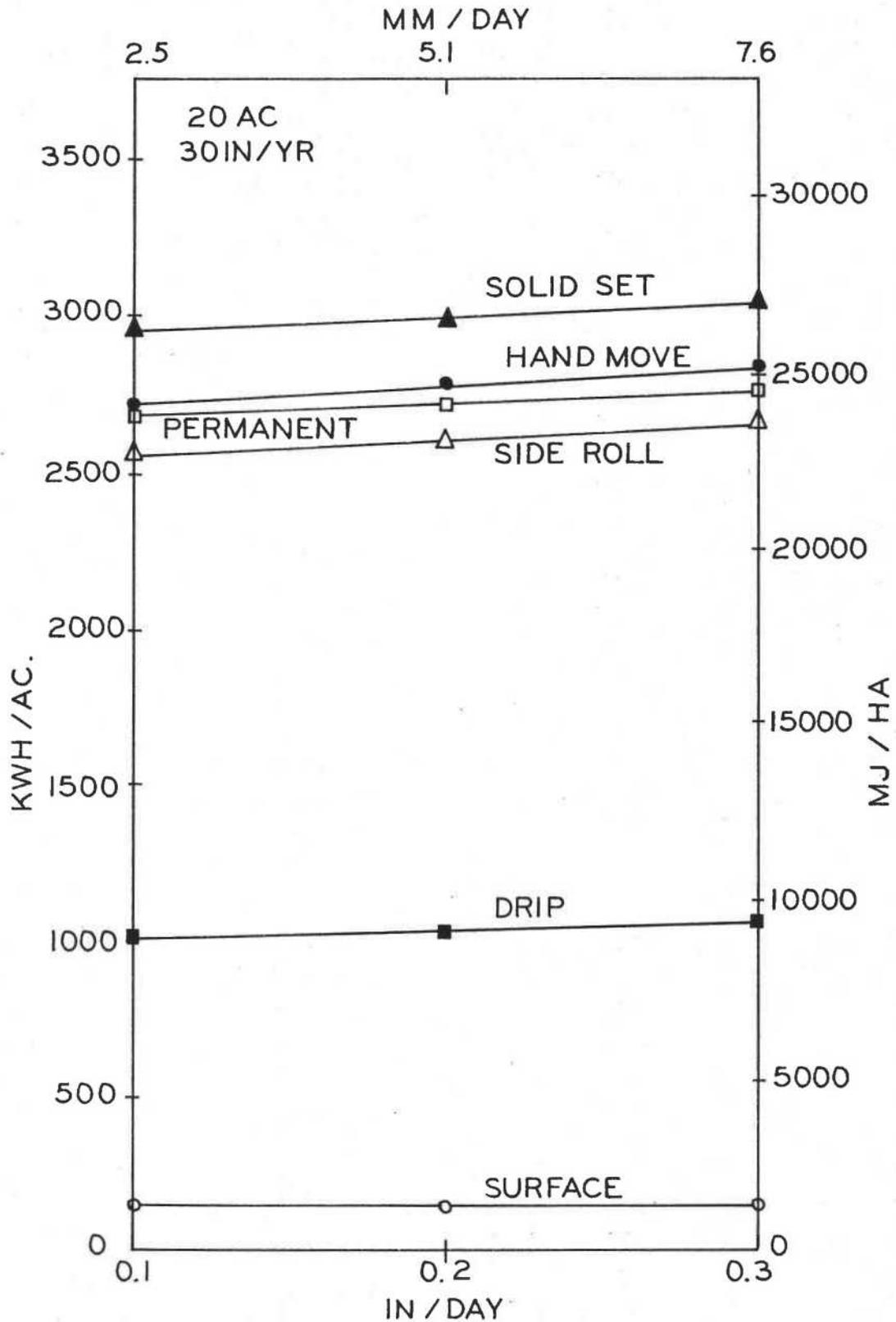
Figure 4. Plot of total seasonal energy as a function of consumptive use rate for a 30 inch (762 mm) seasonal application on a 20 acre (8.1 ha.) field.
