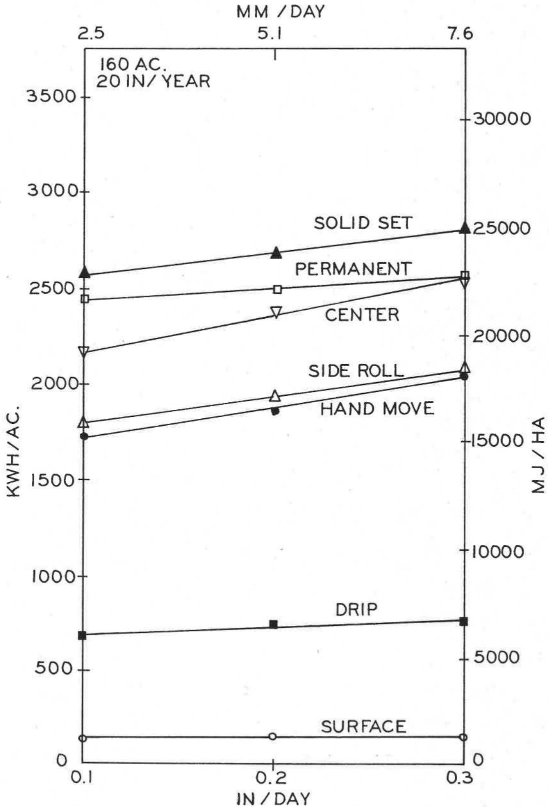
Figure 9. Plot of total seasonal energy as a function of consumptive use rate for a 20 inch (508 mm) seasonal application on a 160 acre (64.8 ha.) field.
