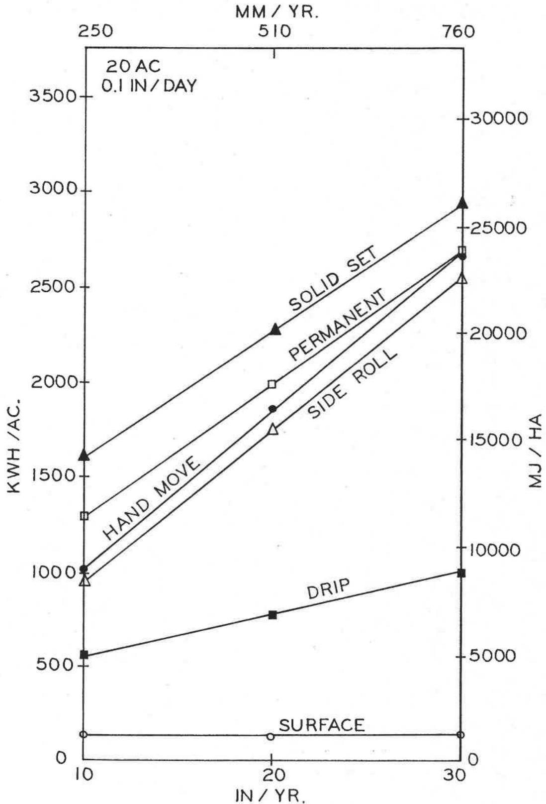
Figure 11. Plot of total seasonal energy as a function of seasonal application on a 20 acre (8.1 ha.) field with a consumptive use rate of 0.1 inch (2.5 mm) per day.
