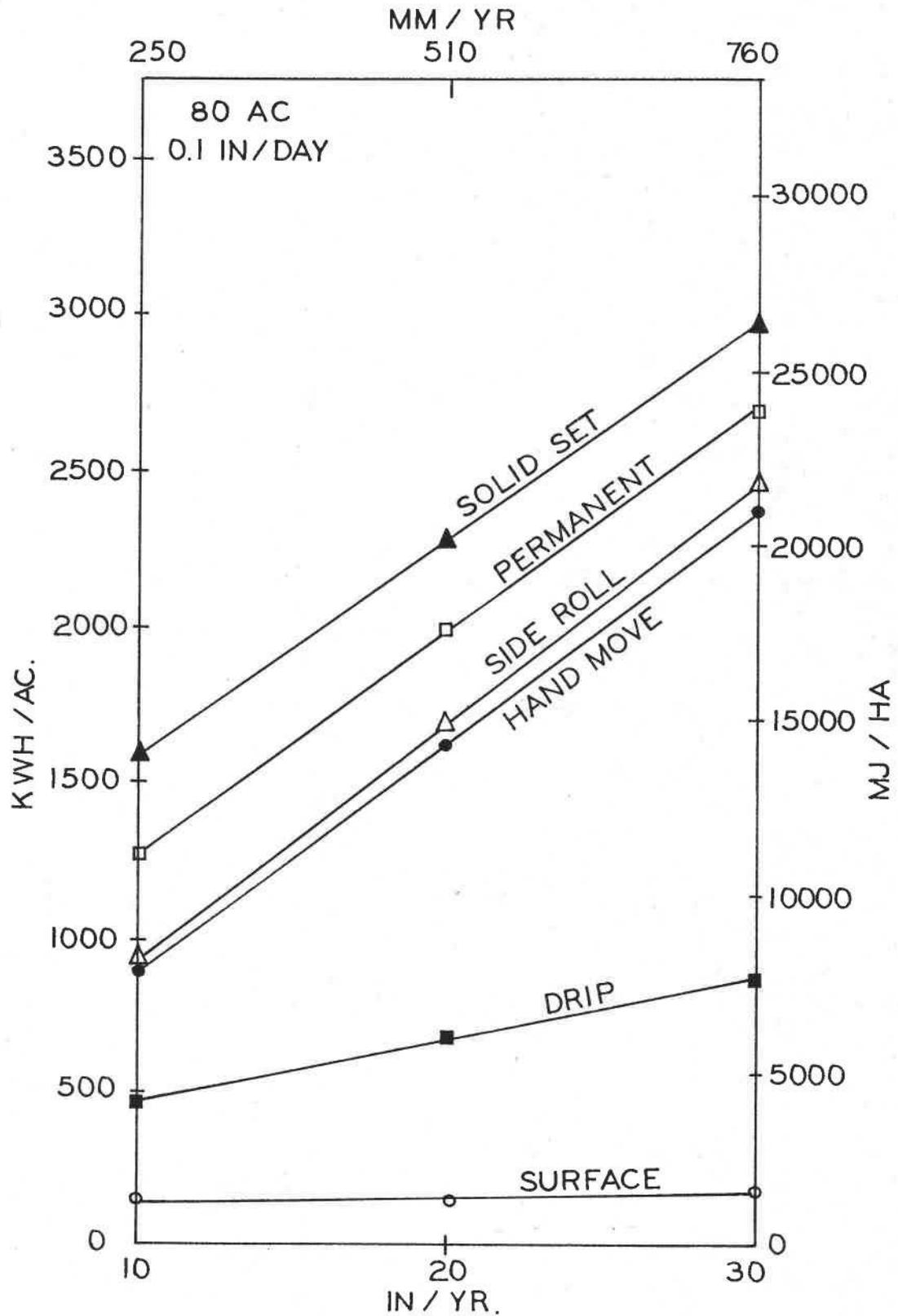
Figure 14. Plot of total seasonal energy as a function of seasonal application on a 80 acre (32.4 ha.) field with a consumptive use rate of 0.1 inch (2.5 mm) per day.
