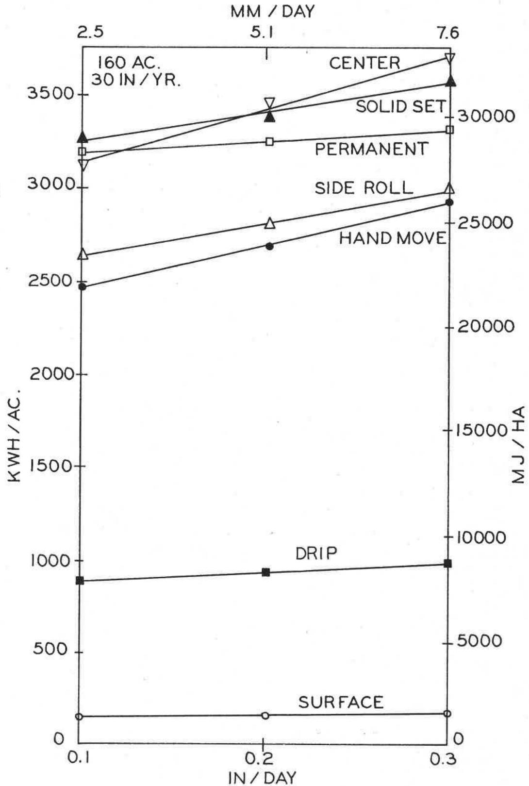
Figure 10. Plot of total seasonal energy as a function of consumptive use rate for a 30 inch (762 mm) seasonal application on a 160 acre (64.8 ha.) field.
