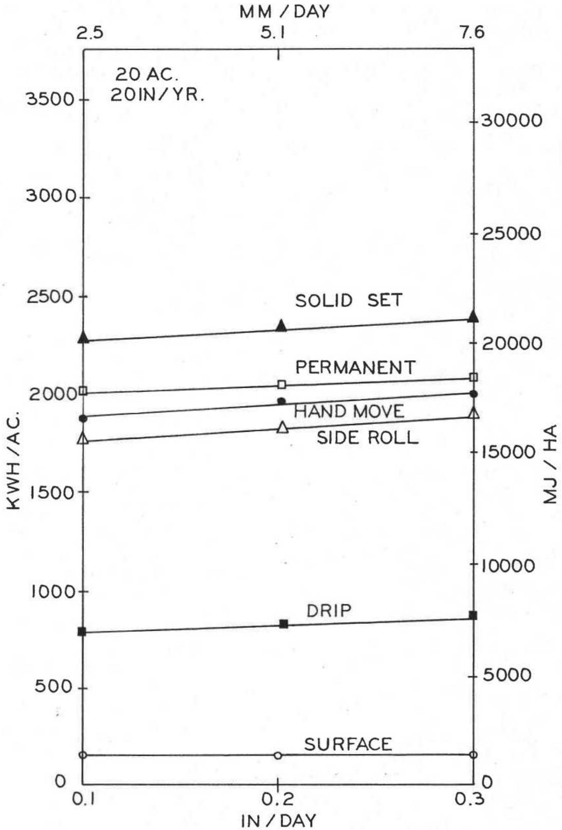
Figure 3. Plot of total seasonal energy as a function of consumptive use rate for a 20 inch (508 mm) seasonal application on a 20 acre (8.1 ha.) field.
