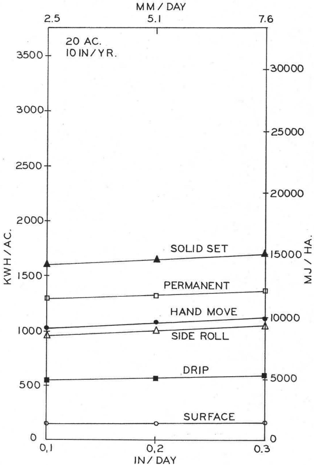
Figure 2. Plot of total seasonal energy as a function of consumptive use rate for a 10 inch (254 mm) seasonal application on a 20 acre (8.1 ha.) field.
