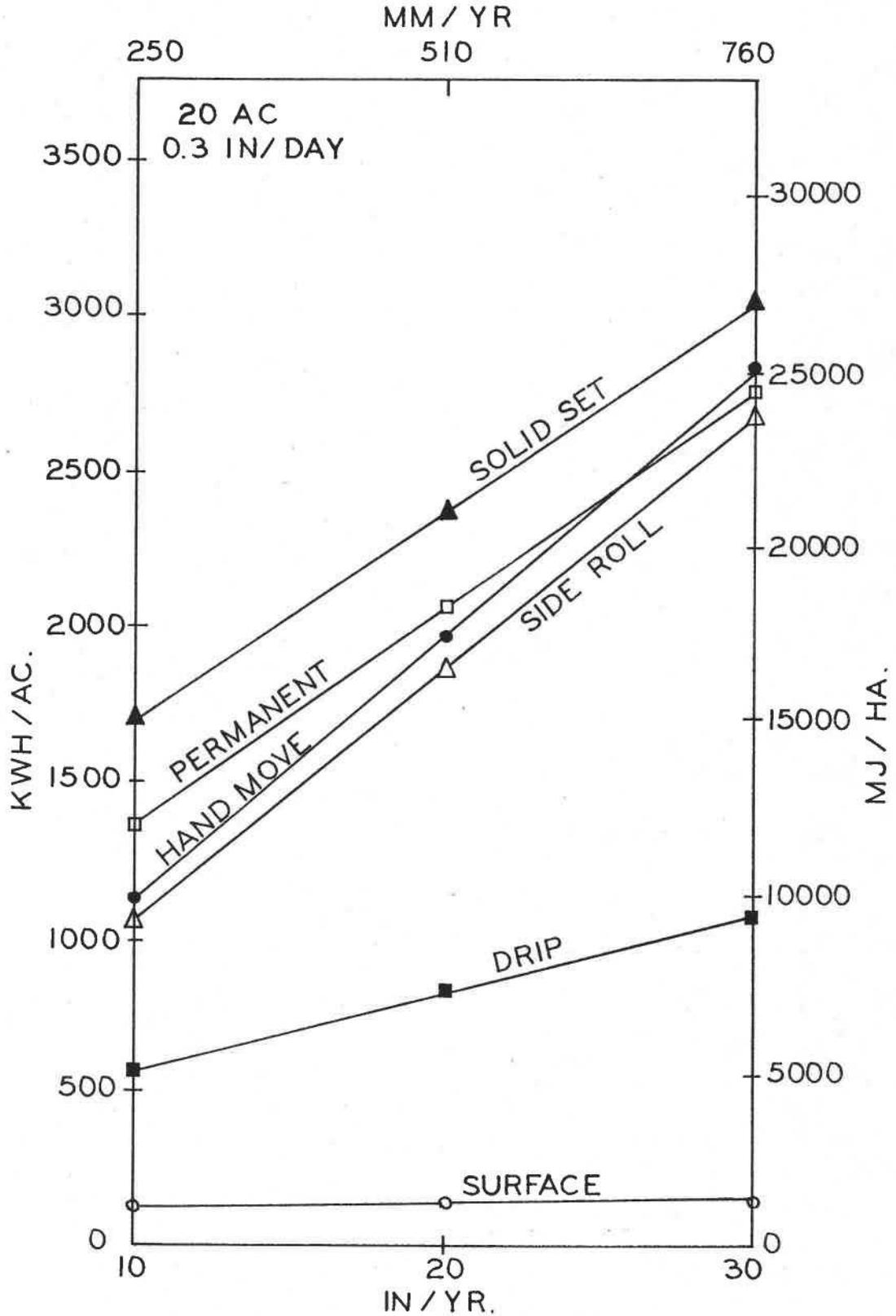
Figure 13. Plot of total seasonal energy as a function of seasonal application on a 20 acre (8.1 ha.) field with a consumptive use rate of 0.3 inch (7.6 mm) per day.
