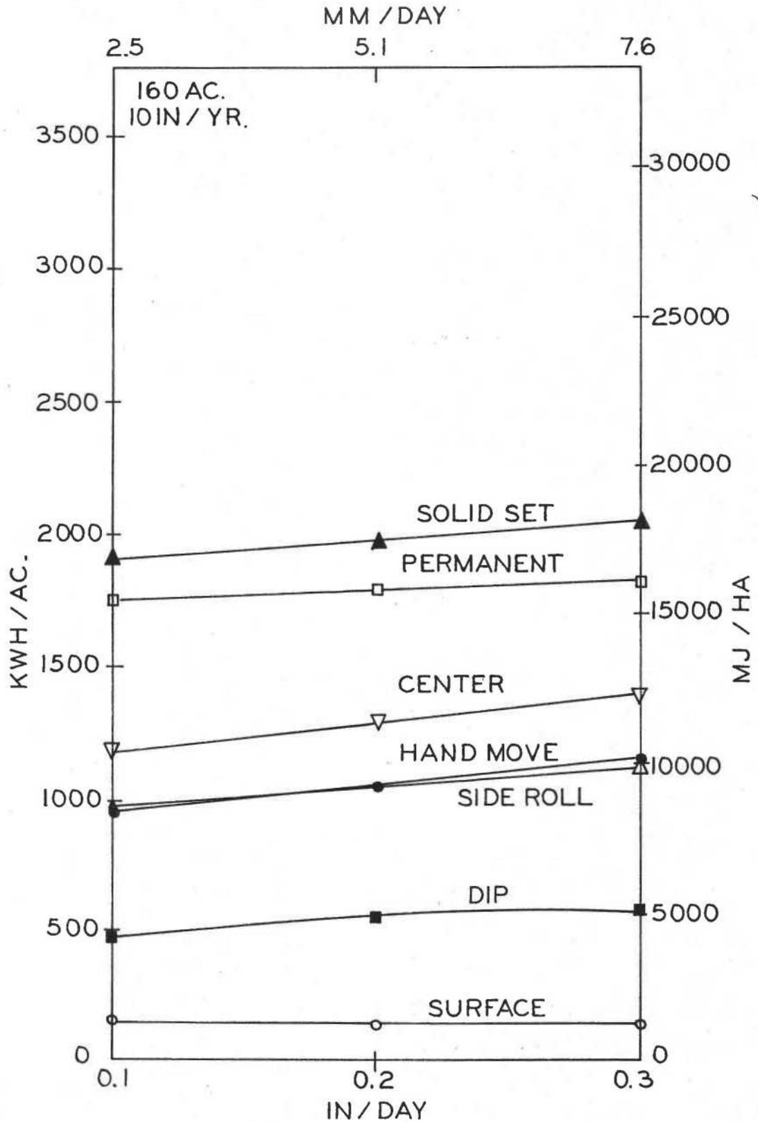
Figure 8. Plot of total seasonal energy as a function of consumptive use rate for a 10 inch (254 mm) seasonal application on a 160 acre (64.8 ha.) field.
