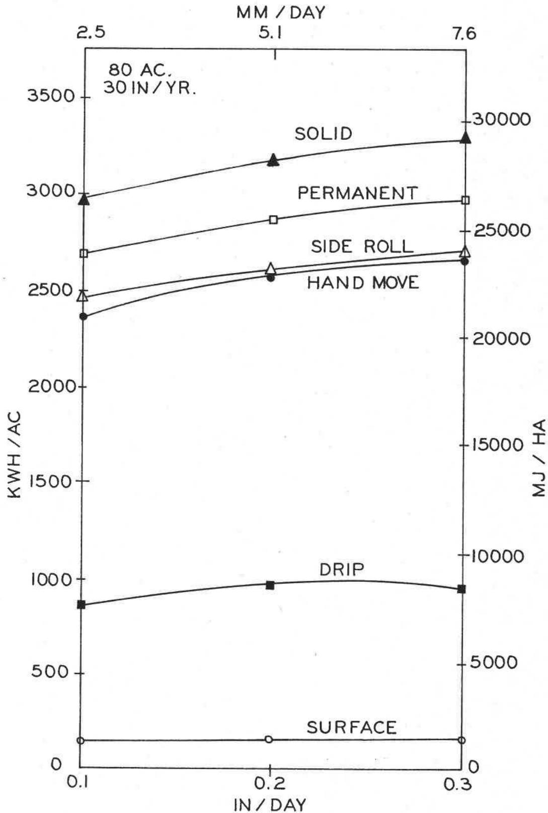
Figure 7. Plot of total seasonal energy as a function of consumptive use rate for a 30 inch (762 mm) seasonal application on a 80 acre (32.4 ha.) field.
