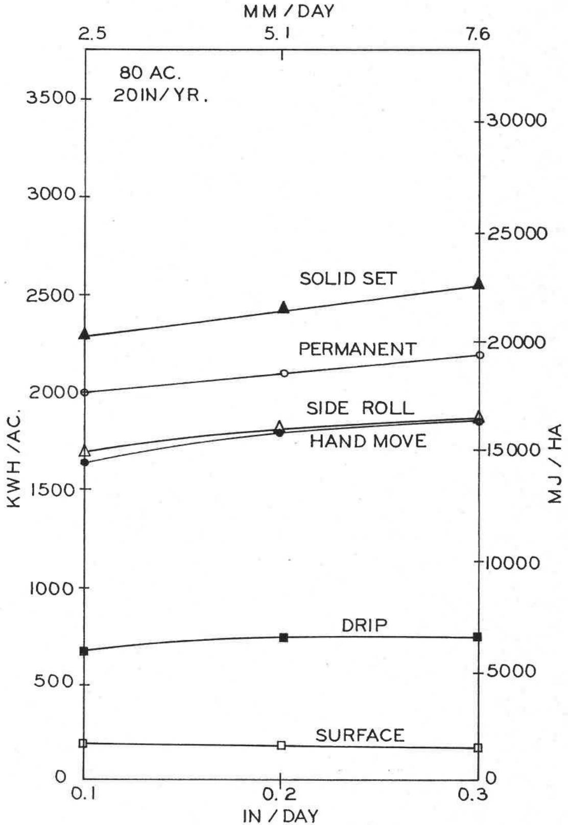
Figure 6. Plot of total seasonal energy as a function of consumptive use rate for a 20 inch (508 mm) seasonal application on a 80 acre (32.4 ha.) field.
