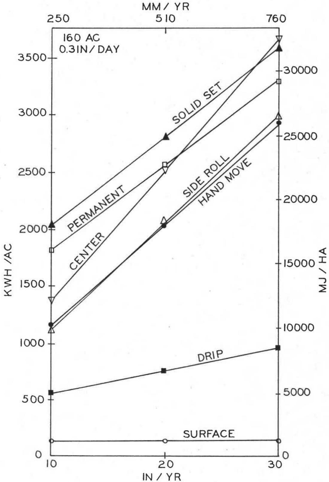
Figure 19. Plot of total seasonal energy as a function of seasonal application on a 160 acre (64.8 ha.) field with a consumptive use rate of 0.3 inch (7.6 mm) per day.
