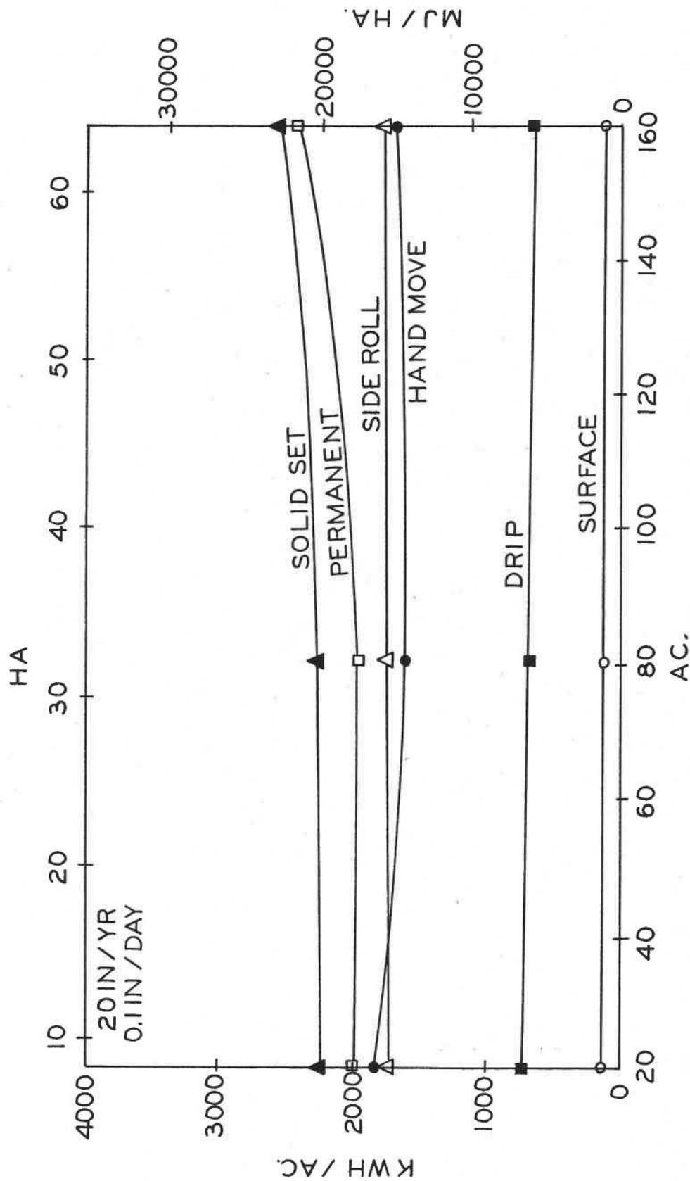
Figure 23. Plot of total seasonal energy as a function of area irrigated for a 20 inch (508 mm) seasonal application with a consumptive use rate of 0.1 inch (2.5 mm) per day.
