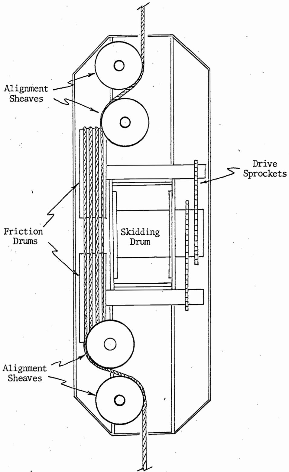
Figure 4. Endless Line Alignment Through the Carriage
