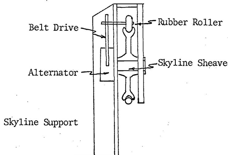
Figure 15. Alternator Drive Assembly
