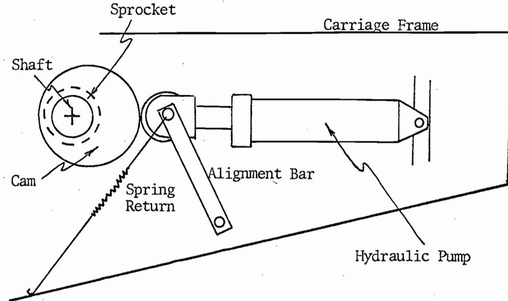
Figure 14. Hydraulic Pump Mechanism
