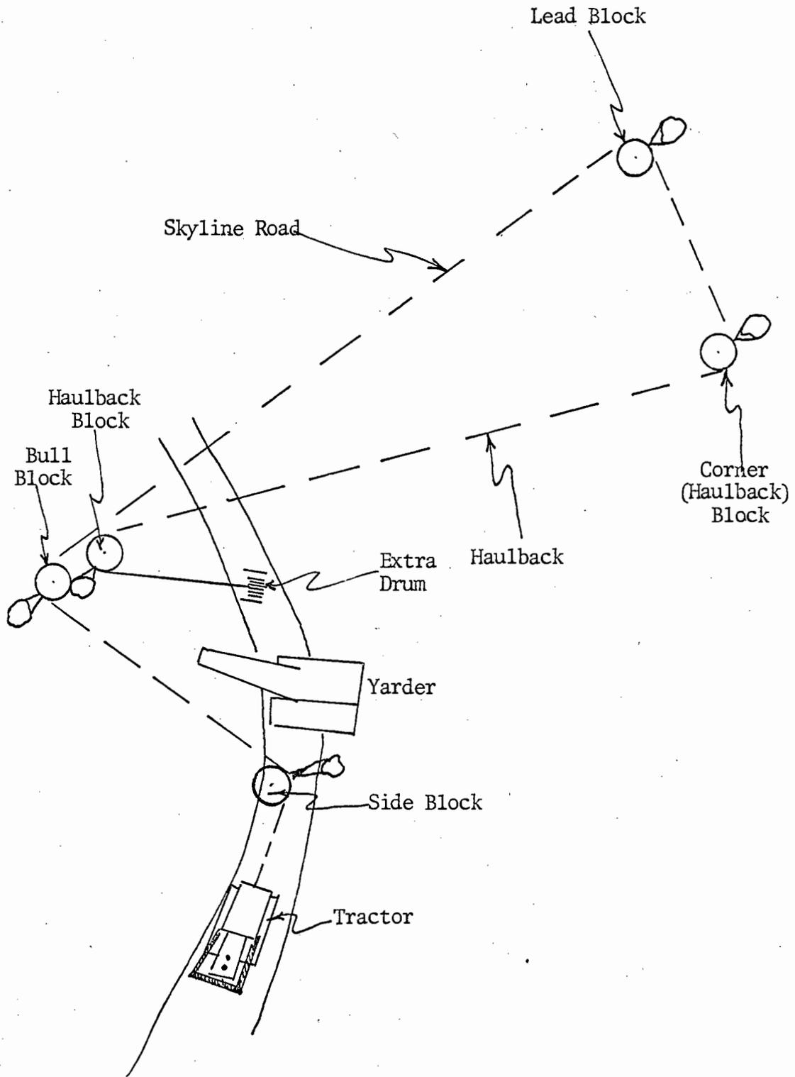
Figure 20. Continuous Line Layout
