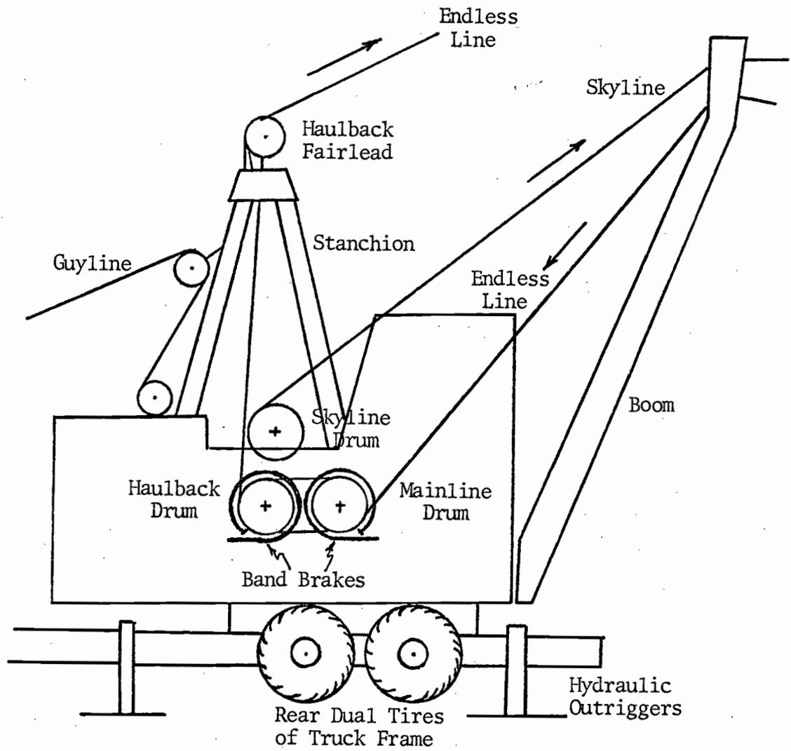
Figure 2. Schematic of Yarder
