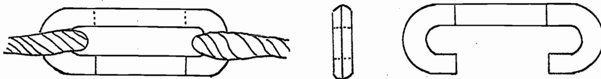
Figure 18. Endless Line Hooks (Couplings)
