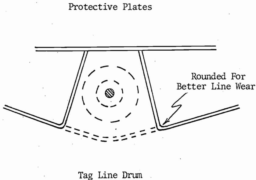
Figure 11. Cross Section of Tag Line Drum and
