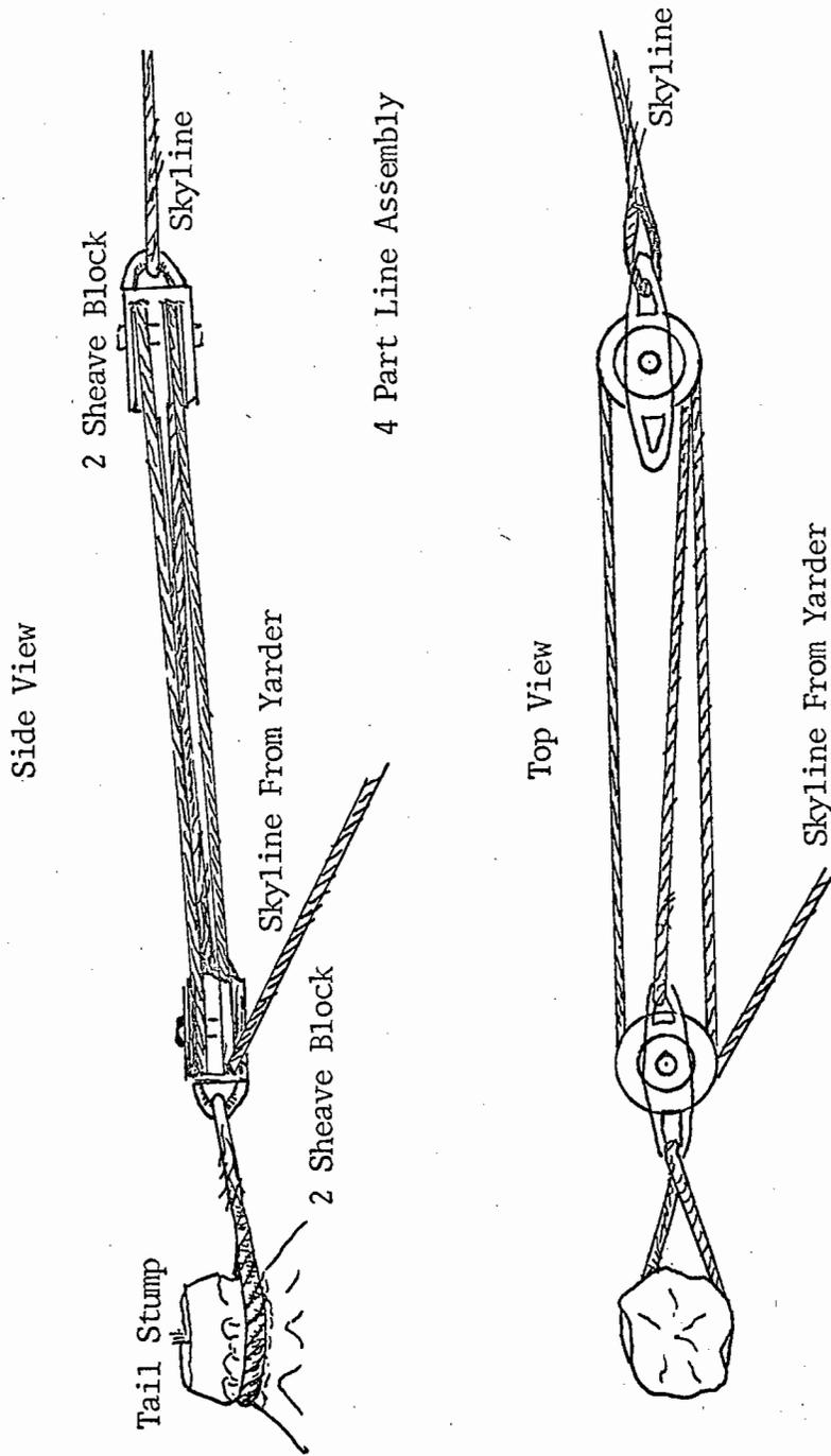
Figure 19. Skyline Head Stump Configuration
