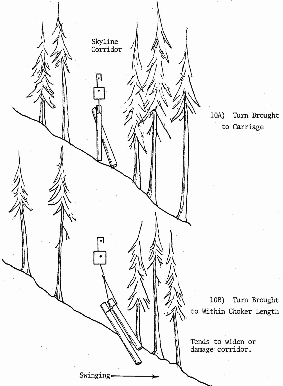
Figure 10. Bringing Logs Up to Carriage (Twito and Lyson, 1973)
