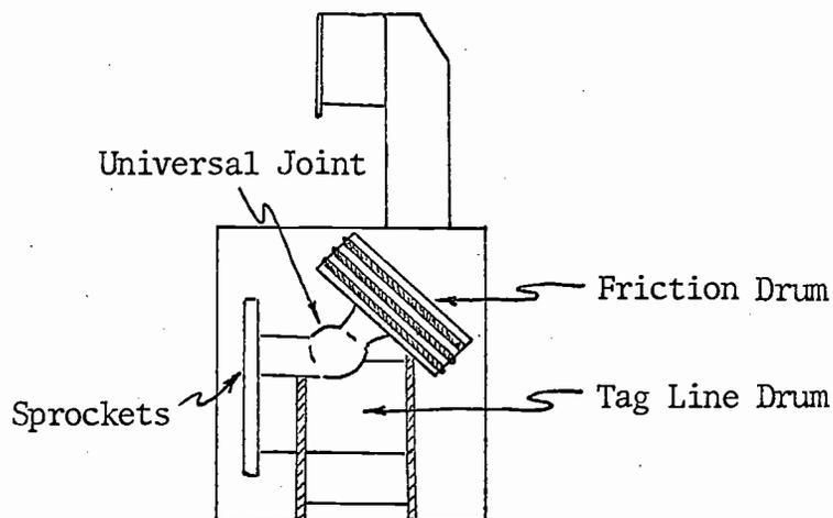
Figure 16. Slanted Friction Drums (End View)
