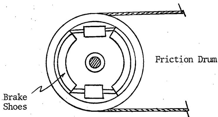
Figure 5. Friction Drum and Brake
