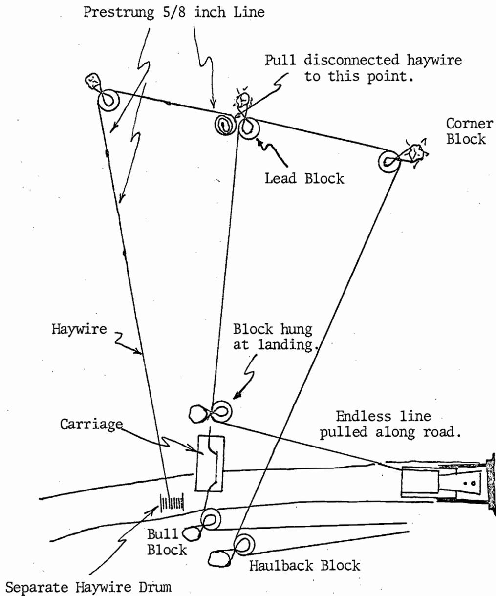
Figure 22. Line Changing (Endless Line)
