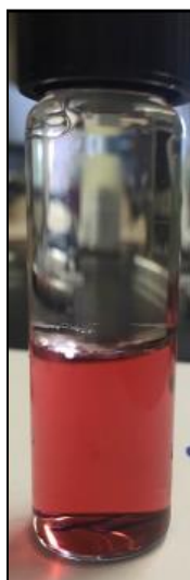
Fig S1. The shake flask method for octanol water partitioning performed using Au NPs. Particles were visually observed to partition to the aqueous phase.
