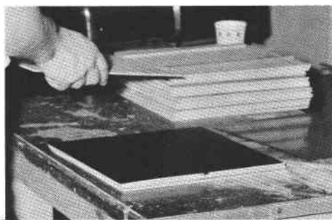
Figure 5. Reassembling veneers after applying glue.
