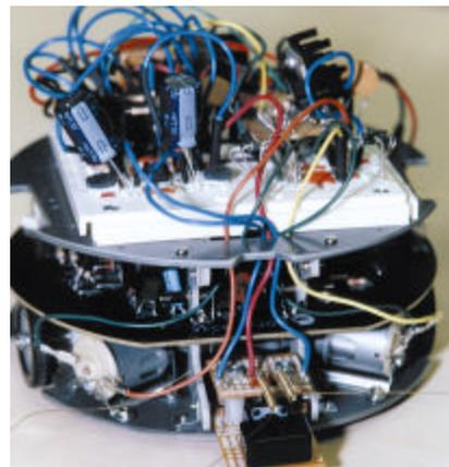
Fig. 2: Graymark robot with bread boarded "whiskers."
