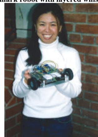
Fig. 4: TekBot robot platform with whiskers and add-on breadboard.
