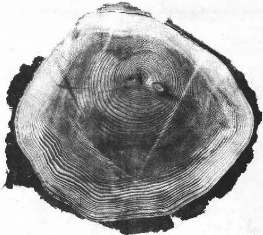
Figure 1.--Cross section of an 18-inch second-growth redwood log showing compression wood on the lower side. The wide rings with wide summerwood constitute the compression wood.
