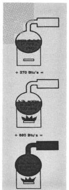
From the steam tables we learn that it takes 270 Btu's of heat to the raise the temperature of one pound of water from 70°F to 338°F at a pressure of 100 psig.
