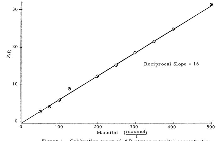
Figure 4. Calibration curve of  $\Delta R$  versus mannitol concentration.
