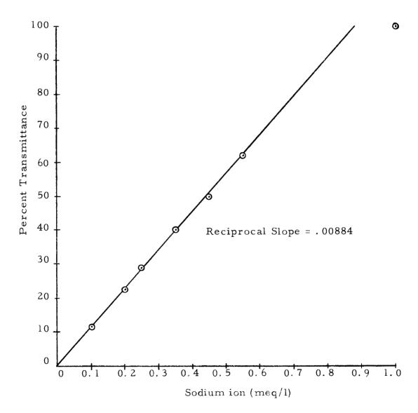
Figure 5. Calibration curve for percent transmission versus sodium ion concentration.
