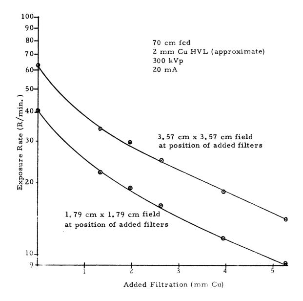
Figure 1. Half-value layer determination.
