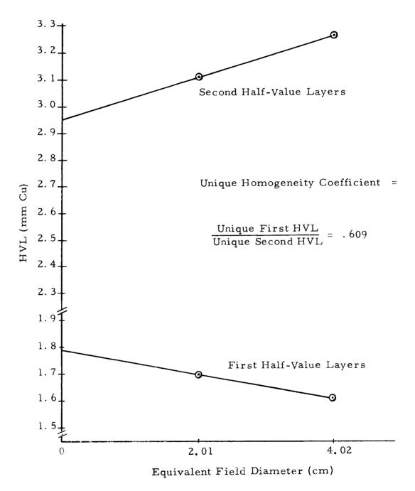
Figure 2. HVL (mm Cu) versus field diameter (cm).
