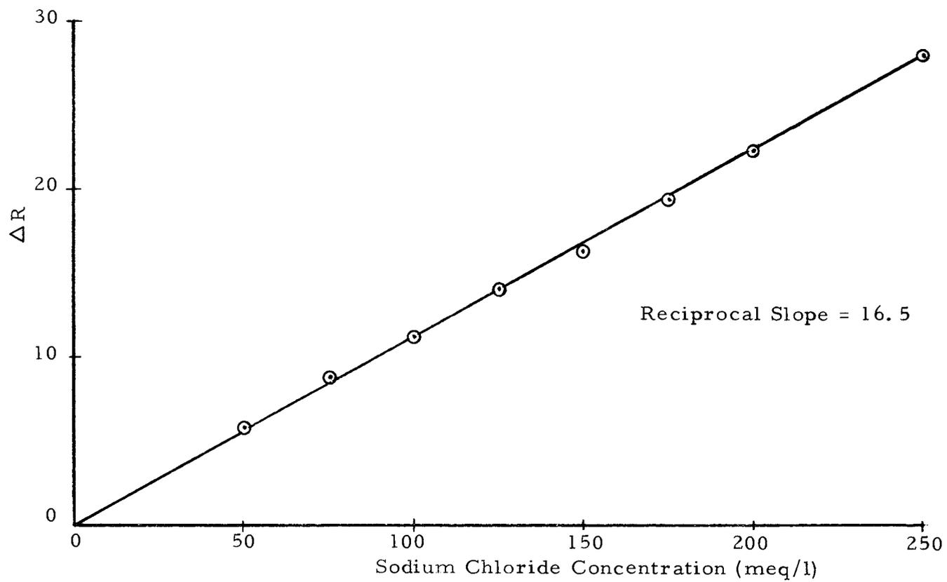
Figure 3. Calibration curve of  $\Delta R$  vs NaCl concentration.
