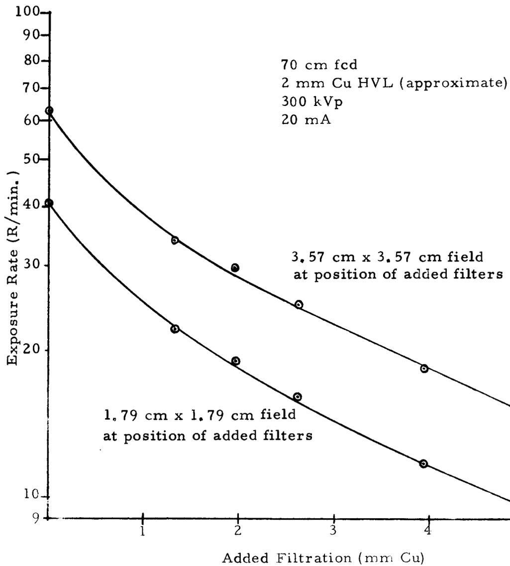
Figure 1. Half-value layer determination.
