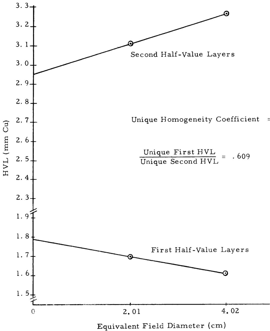
Figure 2. HVL (mm Cu) versus field diameter (cm).
