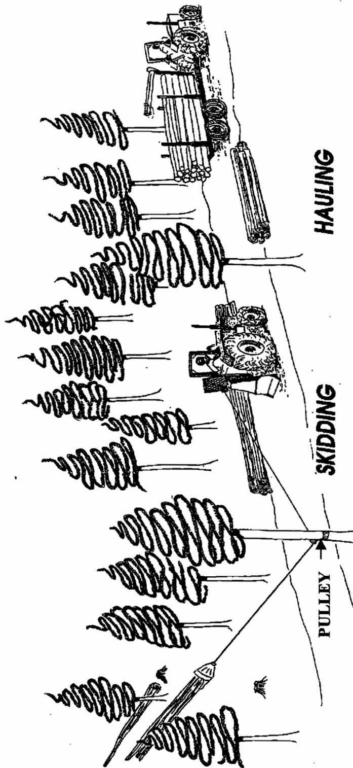
FIGURE 16. Using pulley increases the towing capacity of a farm tractor during skidding operation
