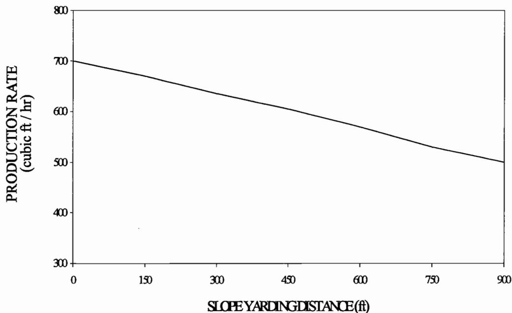
FIGURE 30. Yarding Production Rate by Slope Yarding Distance (Kellogg, 1986).
