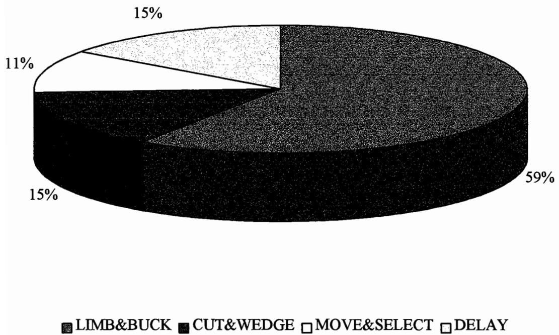
FIGURE 10. Felling Cycle Elements (Adapted from Kellogg, 1986).
