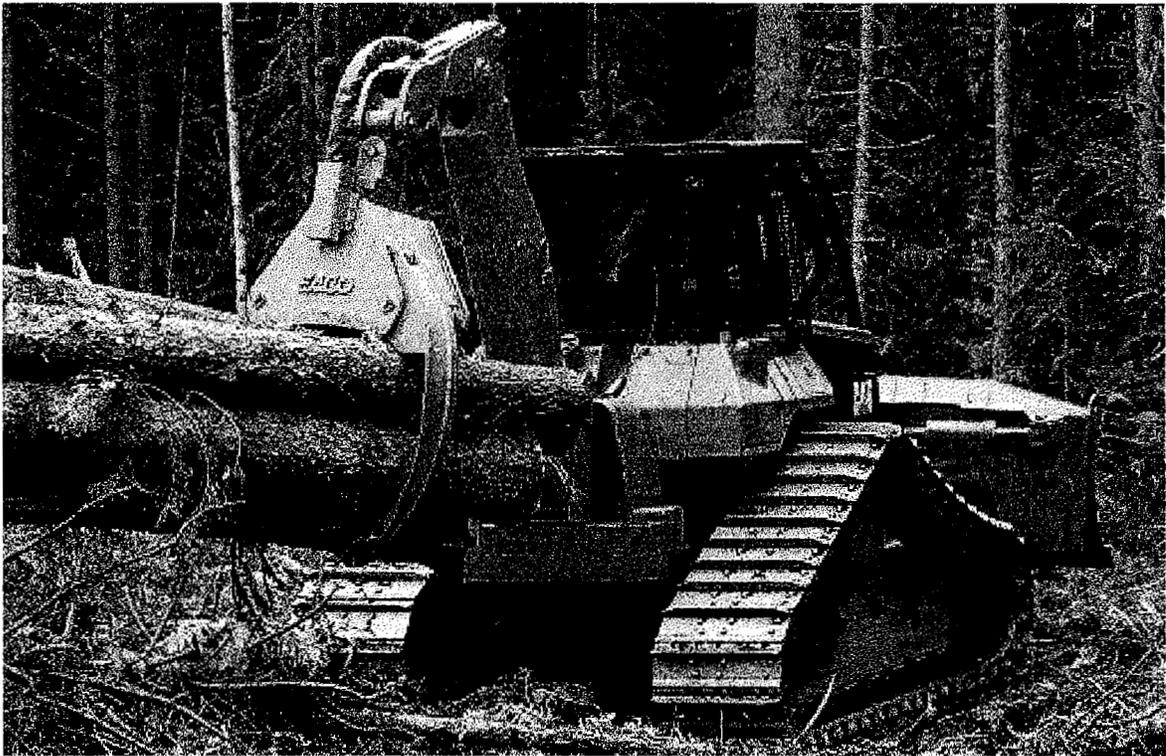
FIGURE 15. Crawler Tractor equipped with Grapple for Skidding and Blade for Light Road Construction.
