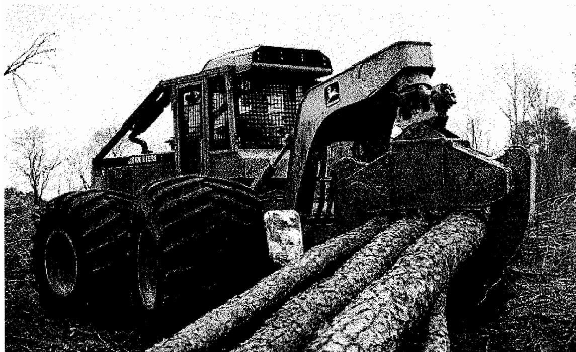
FIGURE 14. An example of the Rubber-tired grapple Skidder.
