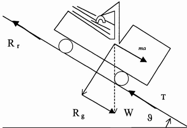
FIGURE 34. Forces acting on a forwarder, travelling downhill with load.
