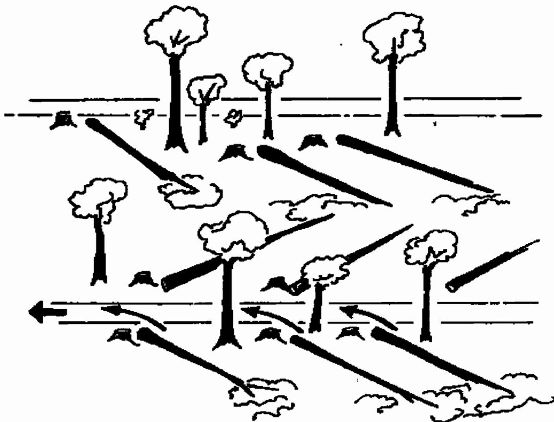
FIGURE 5. Felling in a Herringbone Pattern Away From a Skid Road
