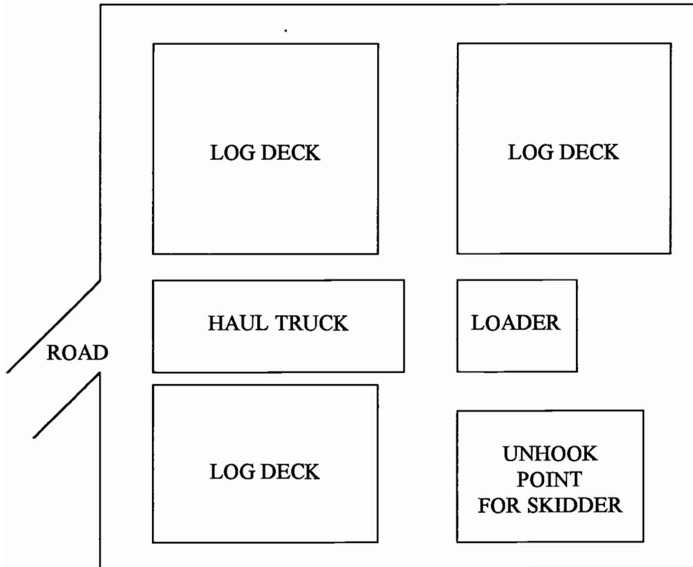
FIGURE 12. Landing Lay Out for Ground-Based Harvesting Systems.
