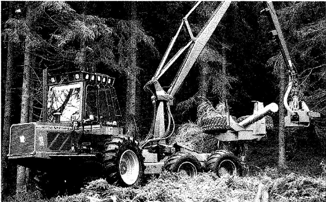
FIGURE 9. Double-grip Harvester Delimiting, and Bucking The Trees During Thinning Operation.
