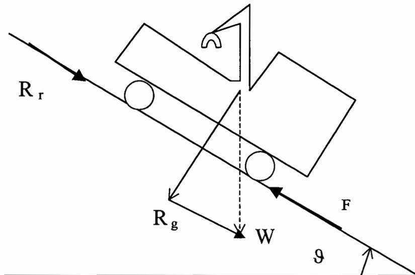
FIGURE 33. Forces acting on a forwarder, travelling uphill without load.
