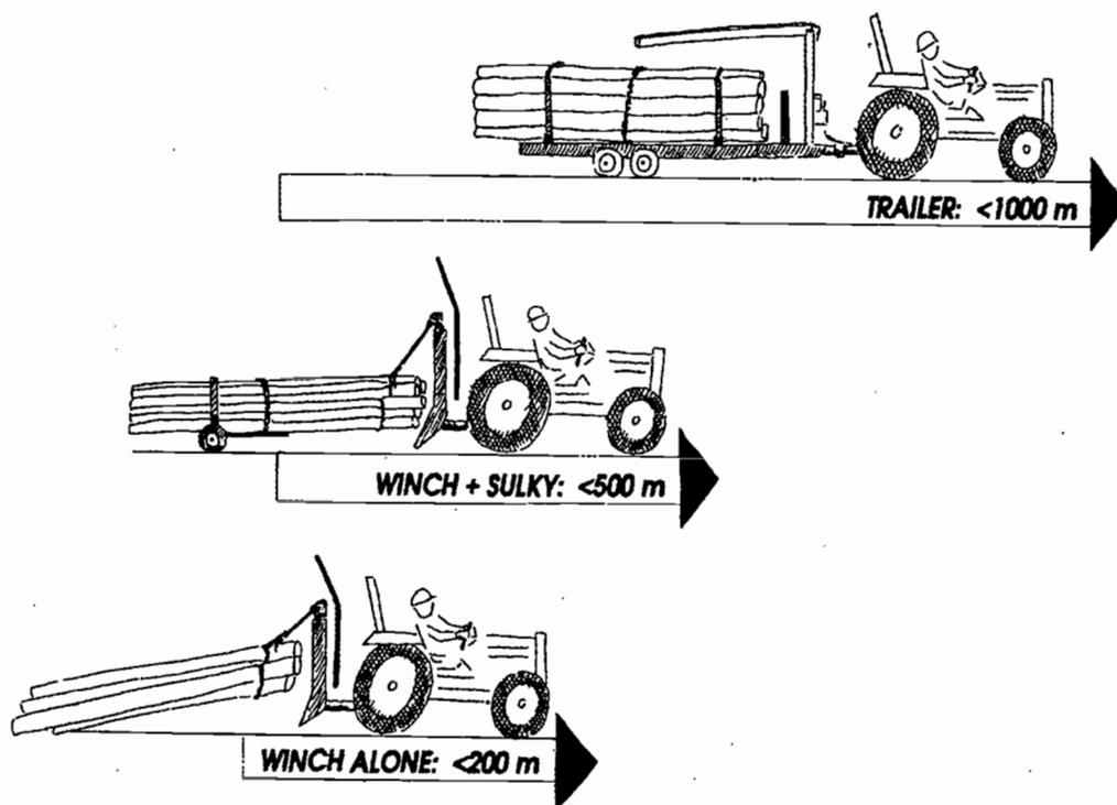
FIGURE 17. Hauling Distance for Skidding with Farm Tractor (Cadorette 1995).
