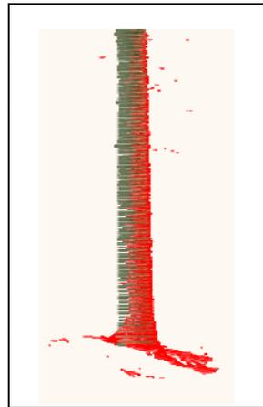
Figure 1.3.5 Stem profile generated from TLS diameter measurements (Bienert et al. 2006)
