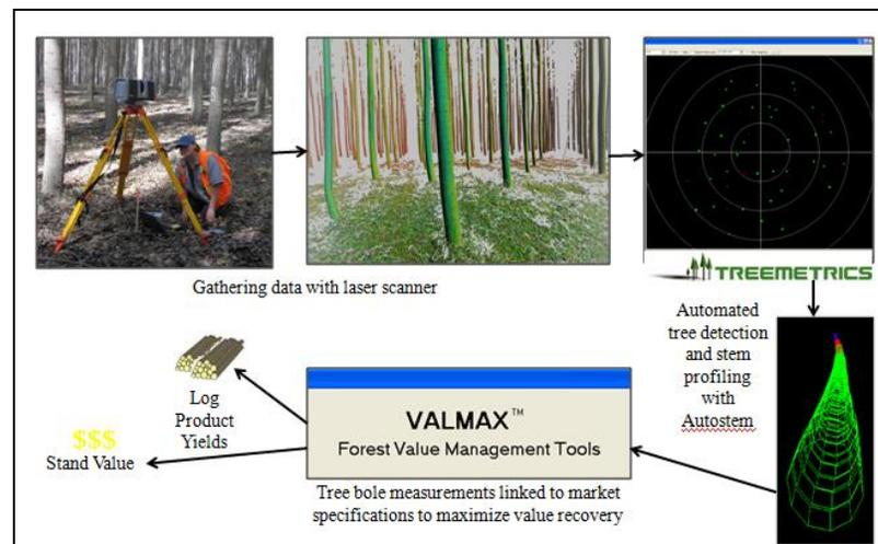
Figure 1.5.2 Process of turning TLS data gathered in the forest (upper left) into TLSOB results by processing plot data into detailed stem profiles (right) and using VALMAX optimization software (bottom center) to generate optimal log product yields and stand values (bottom right)
