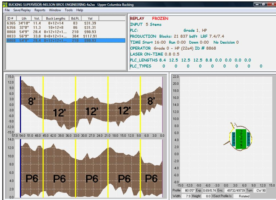
Figure 1.5.1 Log specifications (upper left), bucking lengths (lower left) and boards to be cut (lower right) output on the Nelson Brothers Engineering display screen
