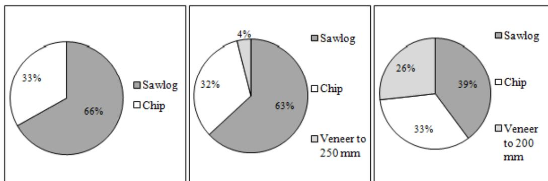
Figure 4.3.1.2 Optimal TLSOB product allocation for Stand M-7
