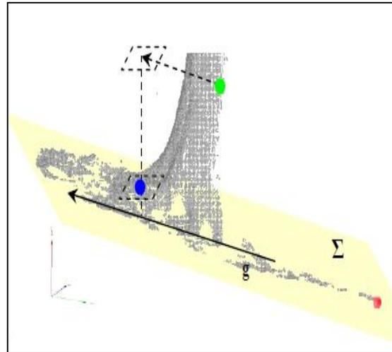
Figure 1.3.4 Calculation of height to DBH based on DTM surface ( $\Sigma$ ) and ground slope angle ( $g$ ) (Bienert et al. 2006)
