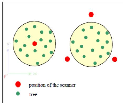
Figure 1.3.2 Image of scanner setup (Bienert et al. 2006)
