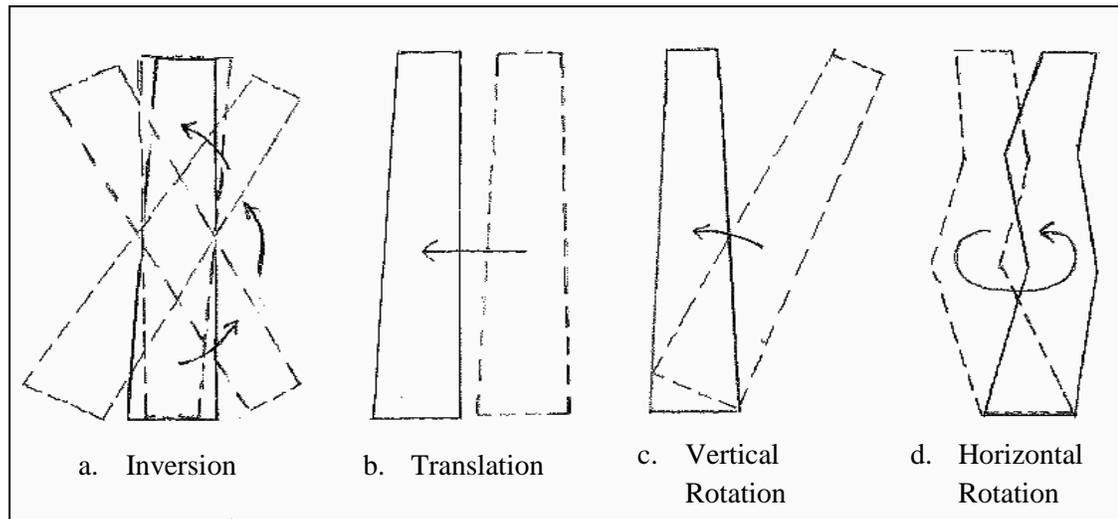
Figure 3.2.1.1 Methods used to invert, translate and rotate the TLS centerline and translate and rotate the NBE centerline
