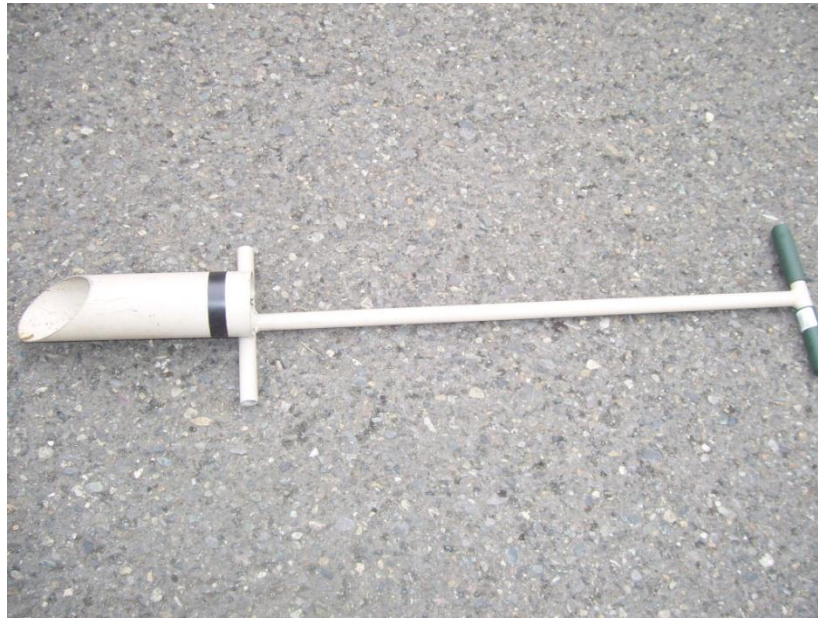
Figure 5, Bulb planter used for collecting core soil samples. (Marked at 15 cm with electrical tape.)
