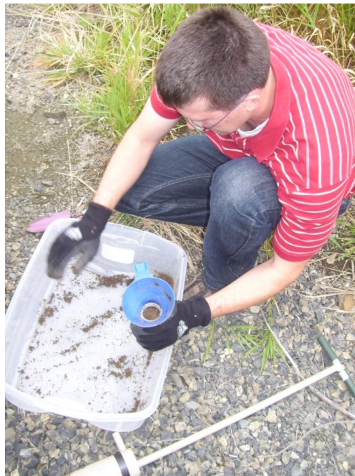
Figure 6, Collecting soil using a collection tray. Tray used to break down compacted samples and transfer to a 500 mL bottle using a funnel.
