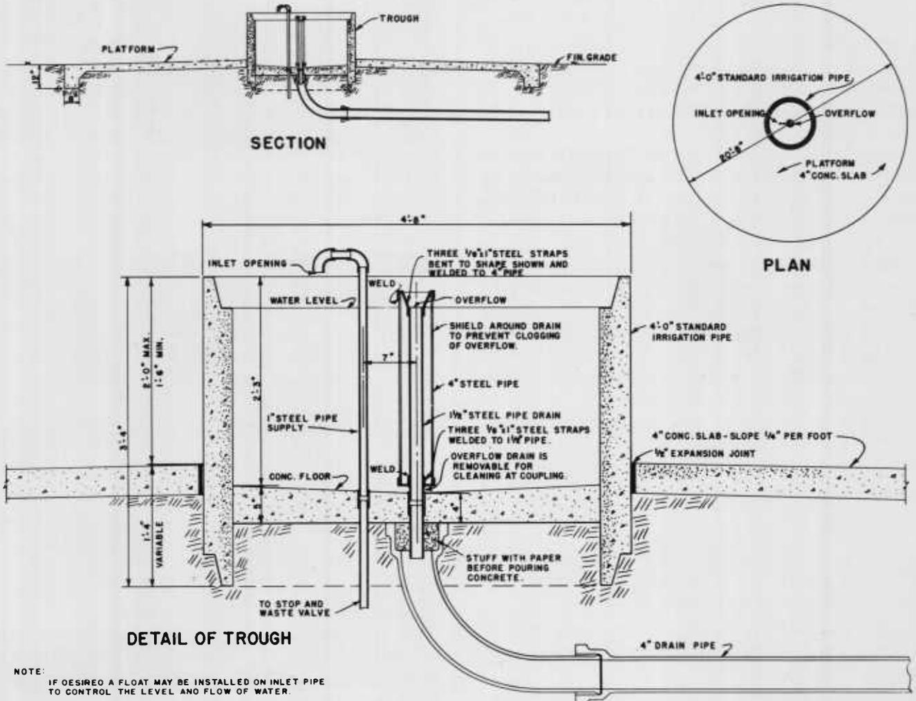
Figure 15. A good design for a stock watering tank.
