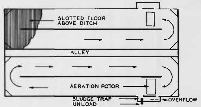
Figure 12. Schematic diagram of a typical oxidation ditch for a swine installation below a slotted floor.
