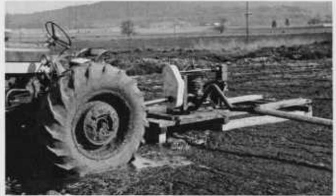
Figure 4. High-pressure liquid manure pump operated by tractor, PTO. Liquid is pumped to a large-capacity revolving sprinkler for final distribution on fields. This open pit received material from the feeding and milking areas. The crusted layer complicates proper agitation prior to pumping into pipe line. Also, the crusted top is a potential area for fly breeding if not handled properly.
