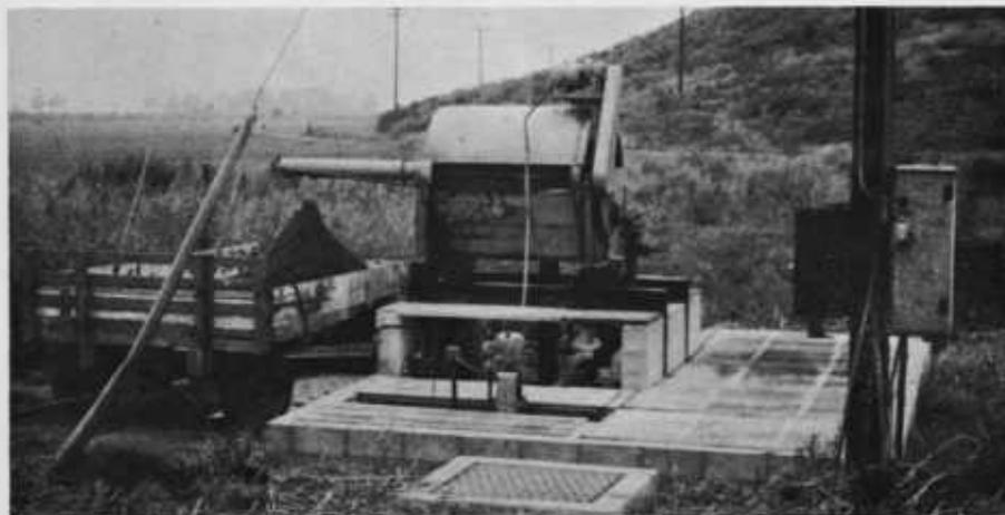
Figure 10. Removing water from manure with a mechanical screen.
