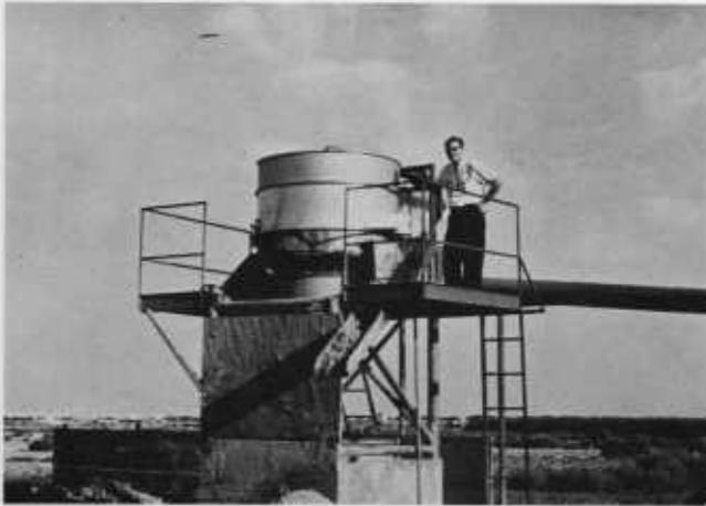
Figure 11. Removing water from manure with another special type of separator.
