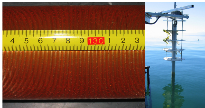
Figure 1. Close-up view of a section of the fiber wrapped sensor tube before painting (left) and sensor tube with radiation shield installed in the water (right).
