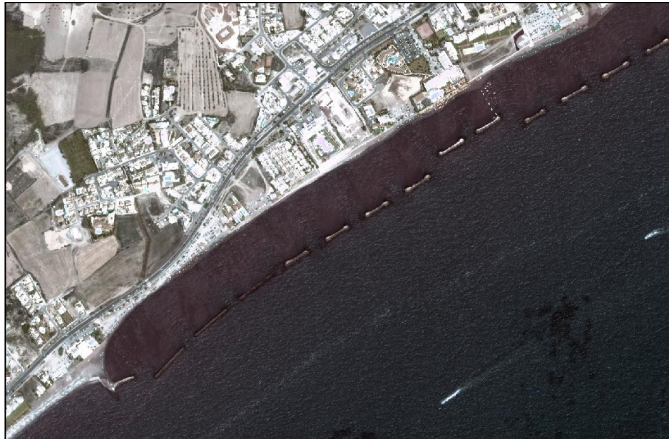
Figure 1-22 Coastal engineering works in northeast Lemesos for the purpose of sand capture.
