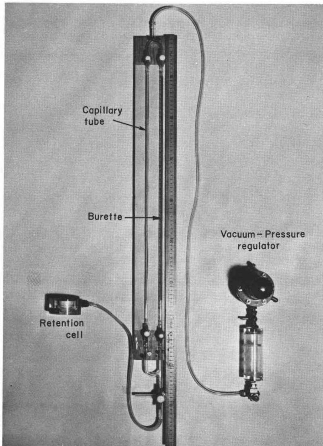
Exhibit 1. Apparatus for obtaining retention data.
