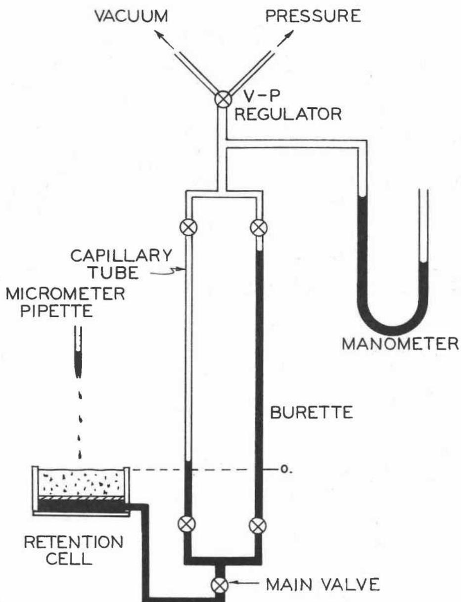
Figure 2. Schematic of the apparatus for obtaining the retention data.
