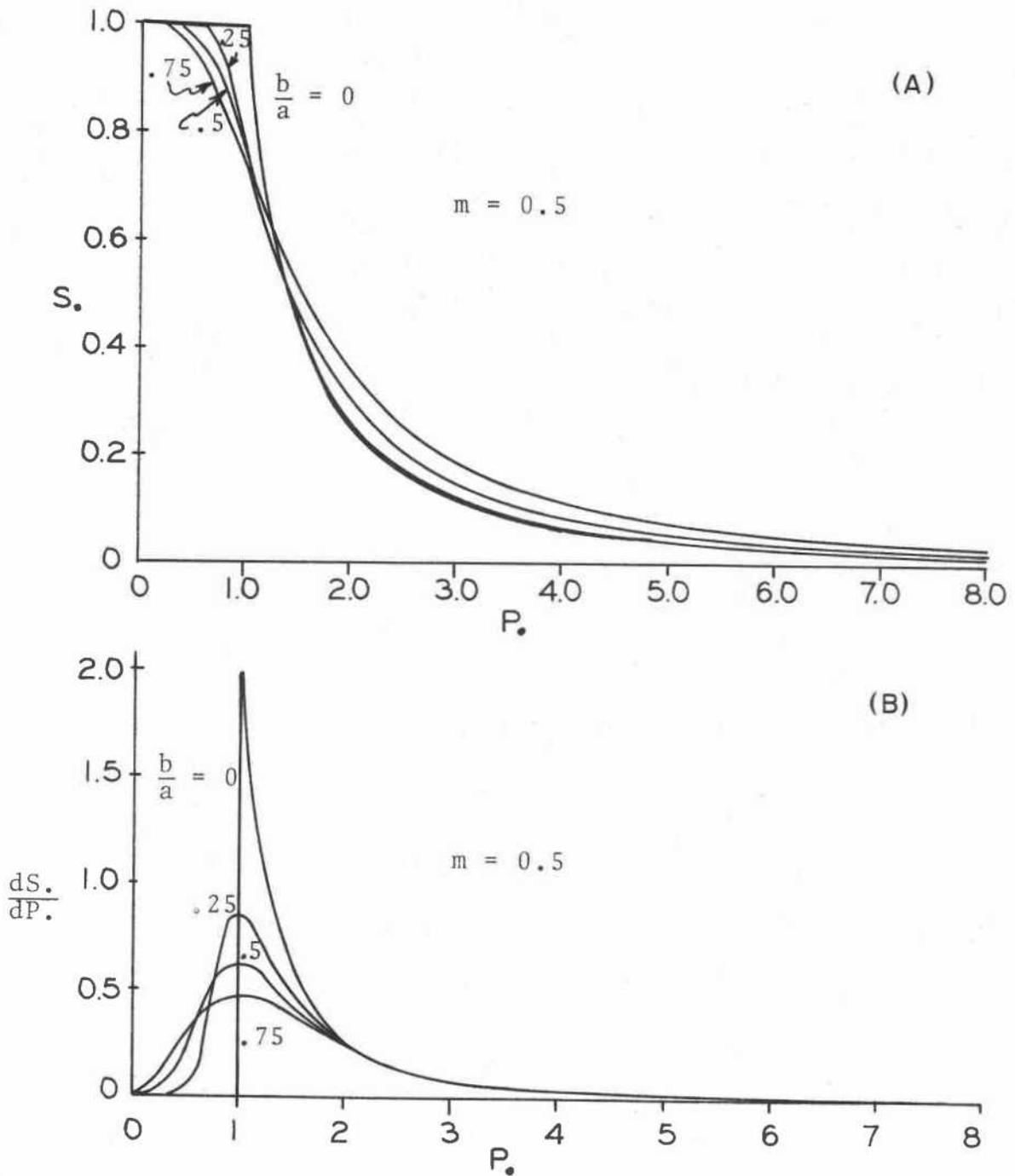
Figure 11. Theoretical curves of scaled saturation and scaled frequency of pore sizes as functions of scaled capillary pressure for hypothetical media having various values of  $b/a$  and  $m = 0.5$ .
