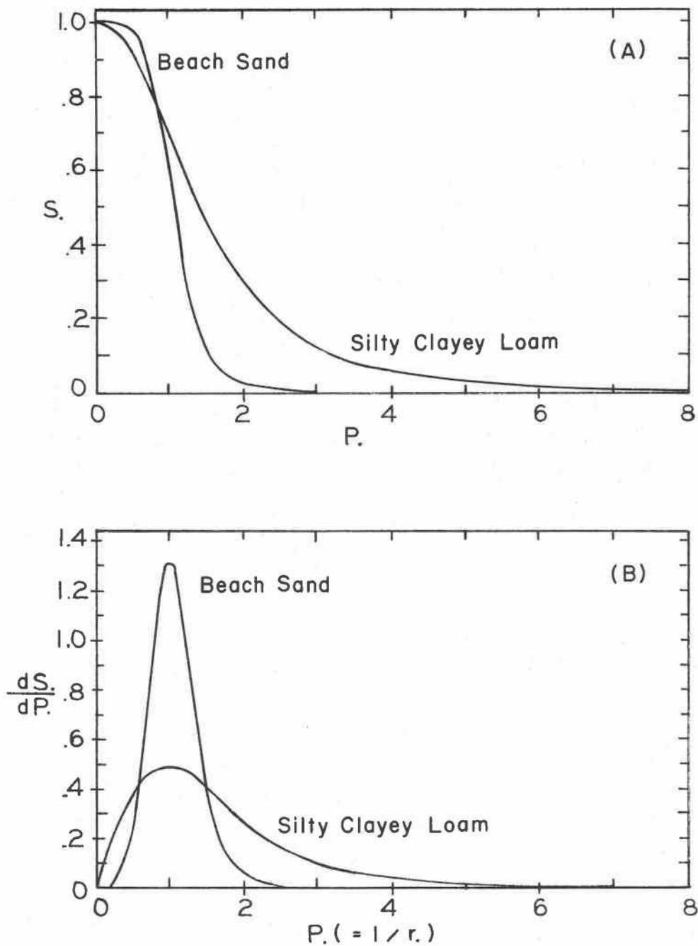
Figure 8. Scaled saturation and scaled frequency of pore sizes as functions of scaled capillary pressure for two media with widely different pore-size distributions.
