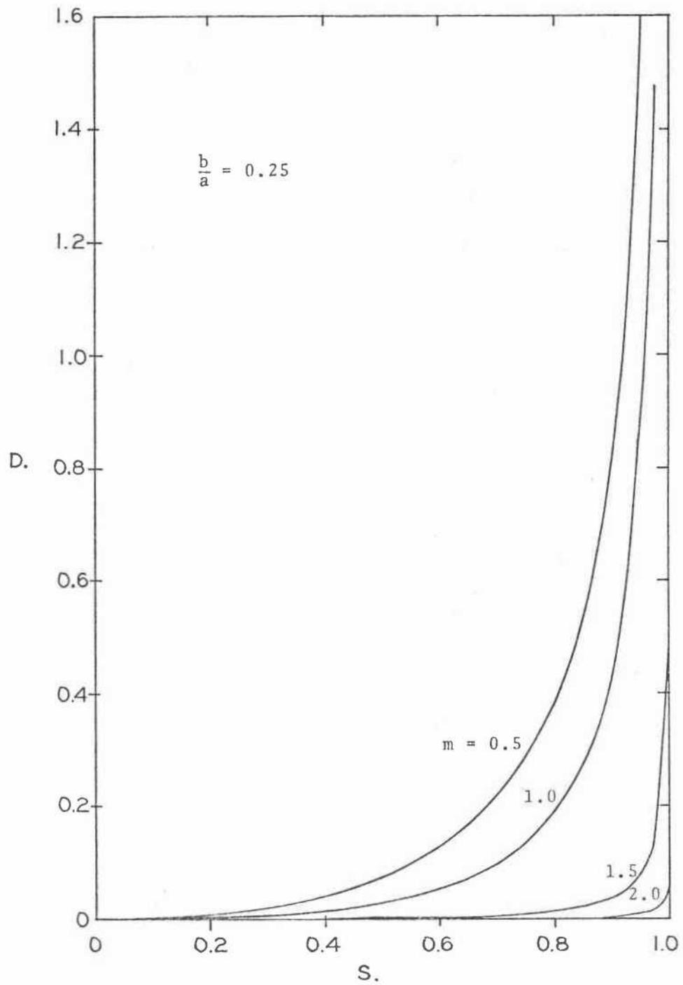
Figure 15. Theoretical scaled diffusivity as a function of scaled saturation for various values of  $m$  and for  $b/a = 0.25$ .
