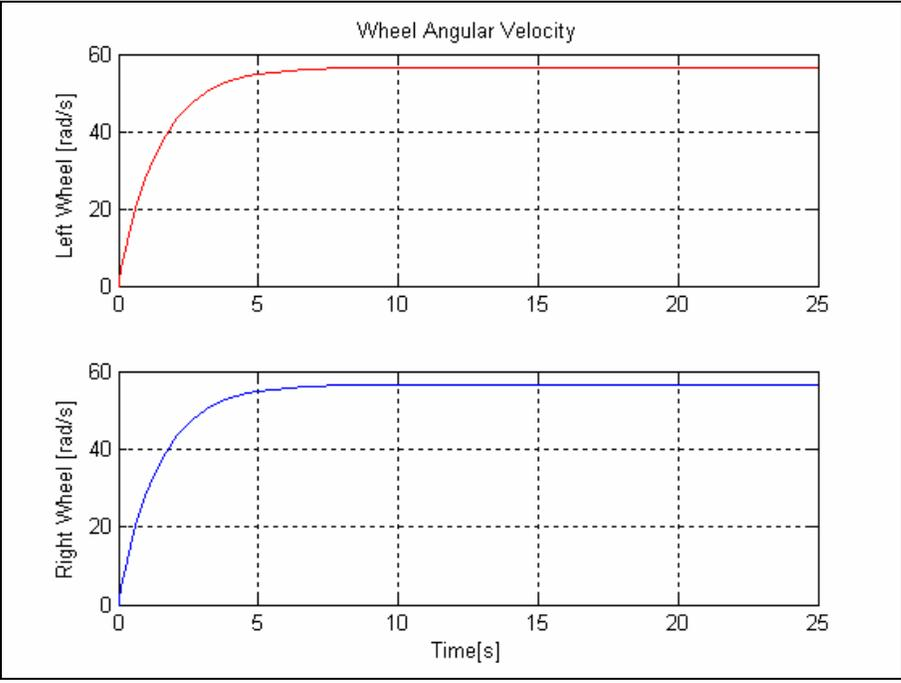
**Figure 12b: Wheel speeds for an uncontrolled slip during a turning maneuver ( $\Phi = 100$  to left)**
