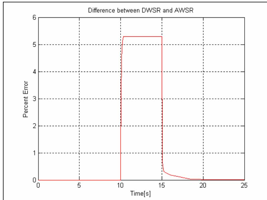
**Figure 10l: DWSR v. AWSR for a controlled straight line travel with slip (State weighting of 100).**
