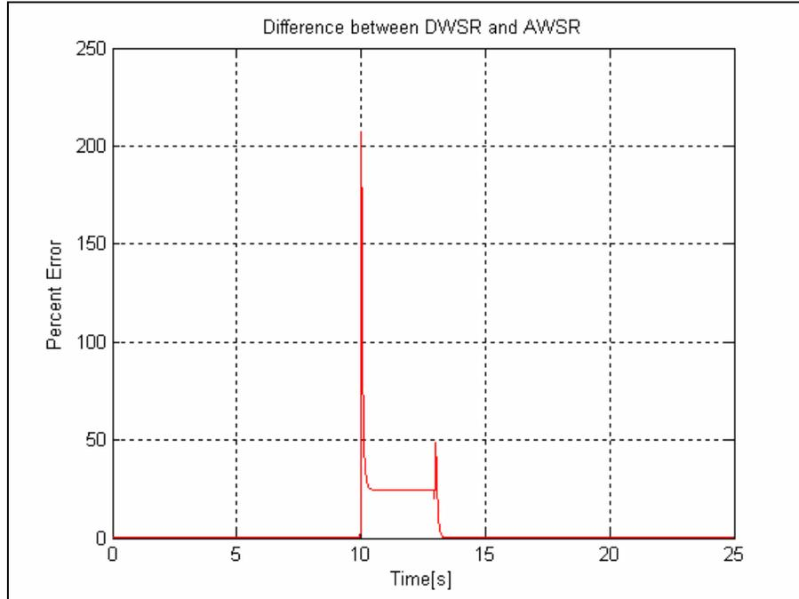
**Figure 12f: DWSR v. AWSR during a controlled slip during a turning maneuver ( $\Phi = 100^\circ$ )**
