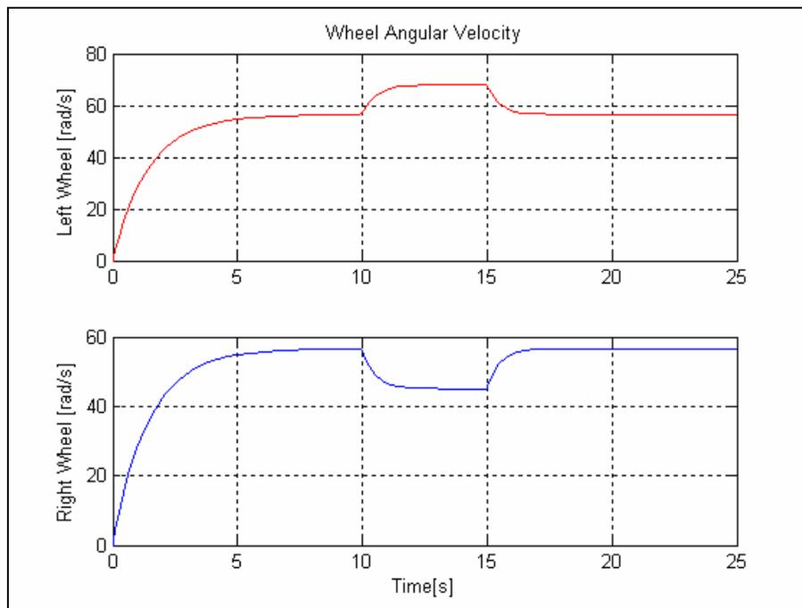
**Figure 10g: Wheel speeds for a controlled straight line travel with slip (State weighting of unity).**
