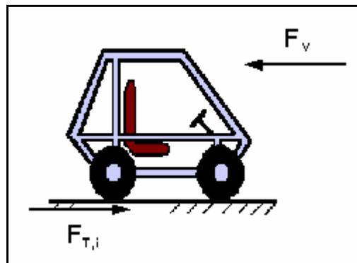
**Figure 2: Free-body diagram of the vehicle.**
