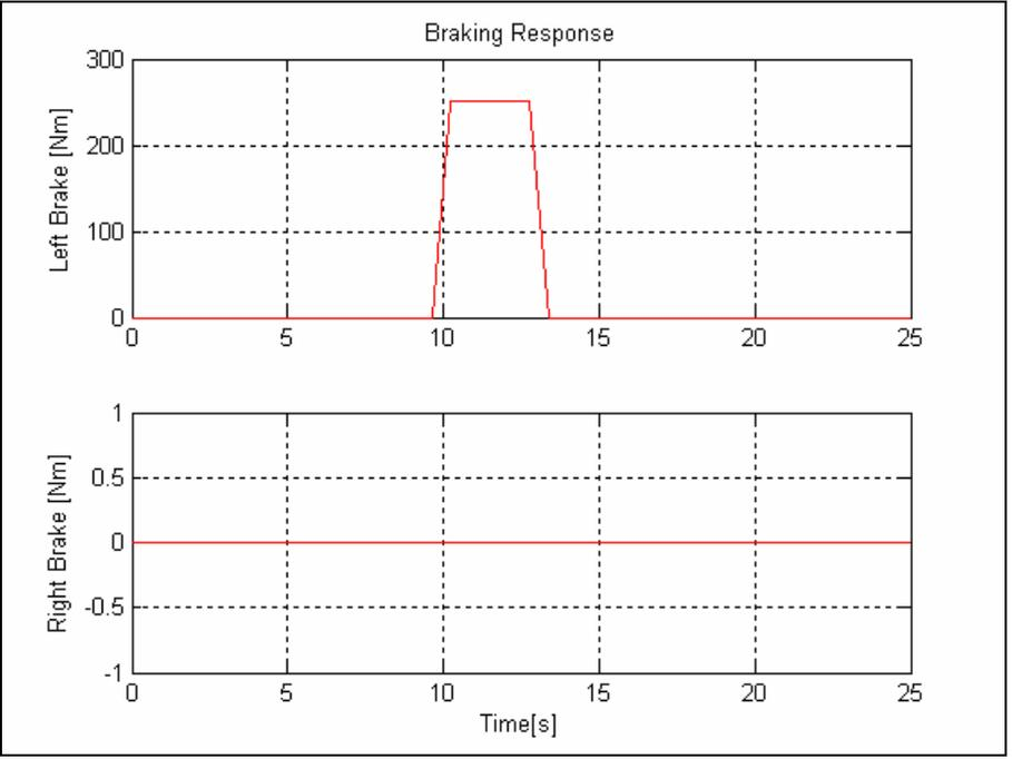
**Figure 12e: Braking response during a controlled slip during a turning maneuver ( $\Phi = 100^\circ$ ).**
