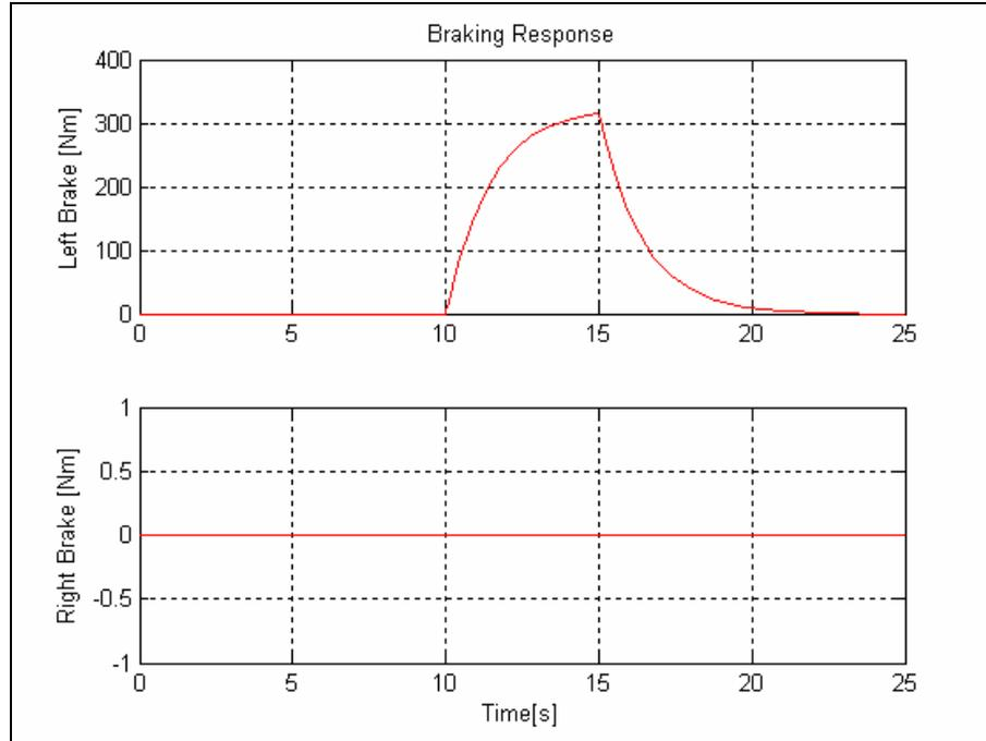
**Figure 10k: Braking response for a controlled straight line travel with slip (State weighting of 100).**
