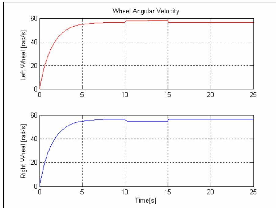
**Figure 10j: Wheel speeds for a controlled straight line travel with slip (State weighting of 100).**
