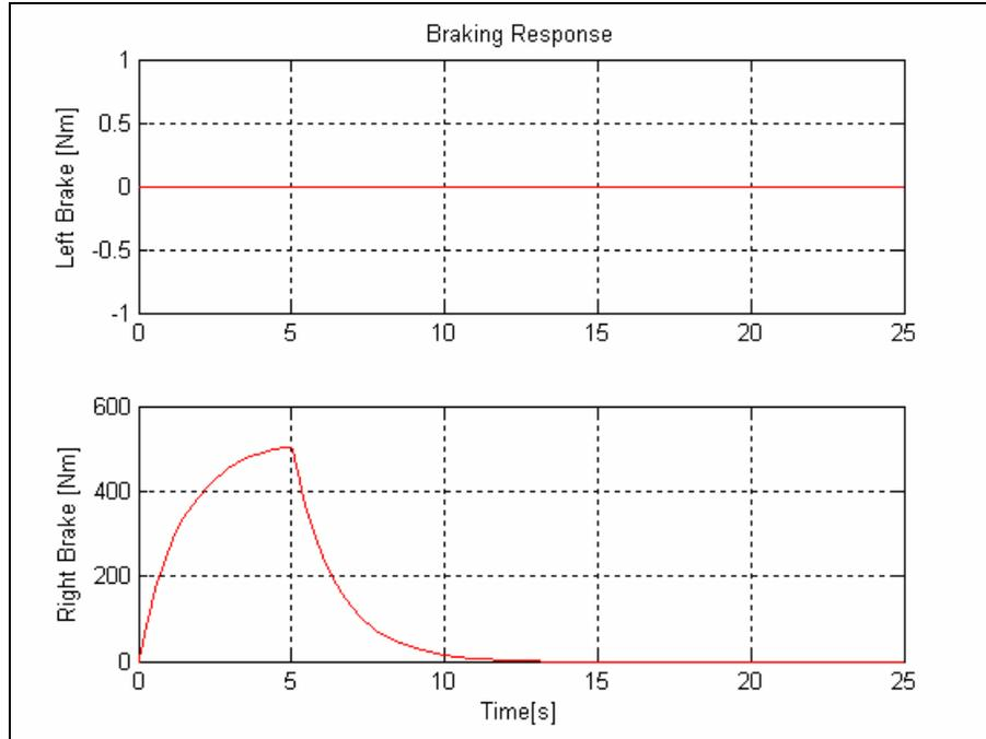
**Figure 11e: Braking response for a controlled straight line acceleration with slip occurring at the start.**
