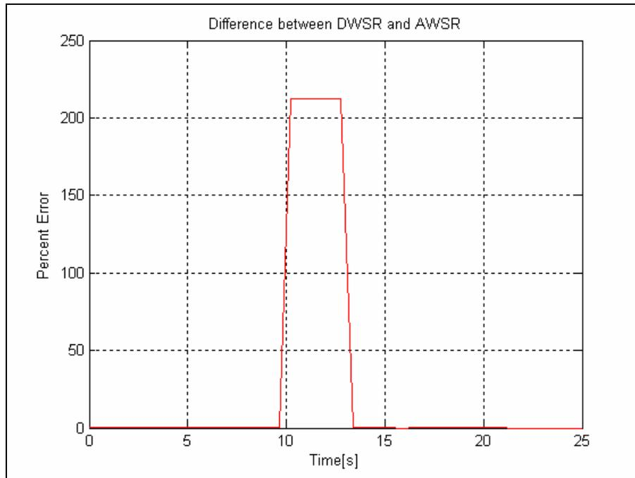
**Figure 12c: DWSR v. AWSR for an uncontrolled slip during situation ( $\Phi = 100^\circ$ ).**
