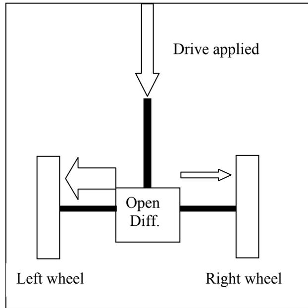
**Figure 15a: Drive torque distribution to the wheels during slip.**
