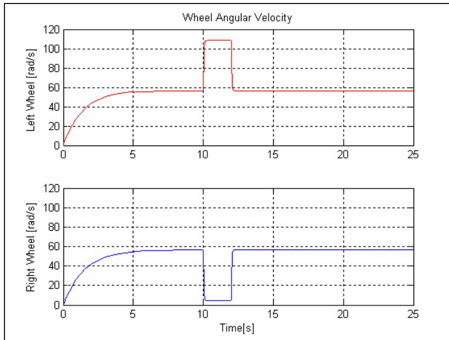
**Figure 13d: Wheel speeds during the controlled slip situations during initial acceleration and during a turning maneuver of  $\Phi = 245^\circ$  issued at  $t=10$  seconds and ending at  $t=15$  seconds.**
