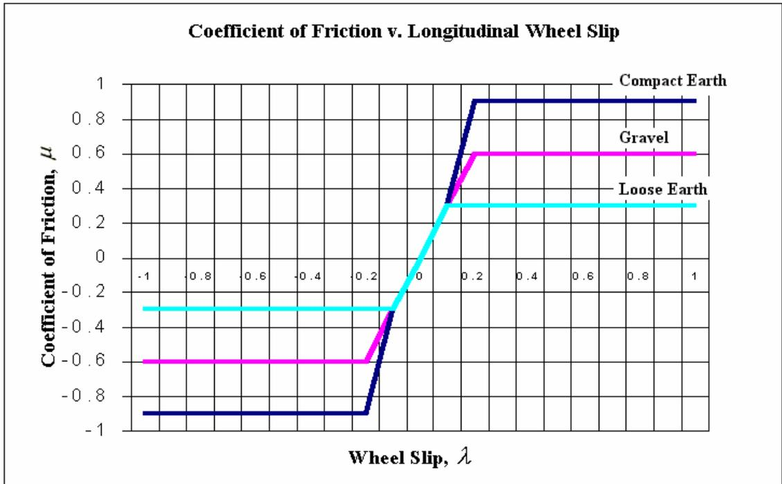
Figure 4: Simplified Pacejka model showing correlation between coefficient of friction and longitudinal wheel slip.
