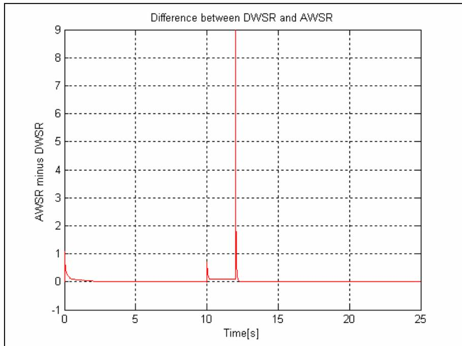
**Figure 13f: DWSR v. AWSR during a controlled slip situation during initial acceleration and during a turning maneuver of  $\Phi = 245^\circ$  issued at  $t=10$  seconds and ending at  $t=15$  seconds.**
