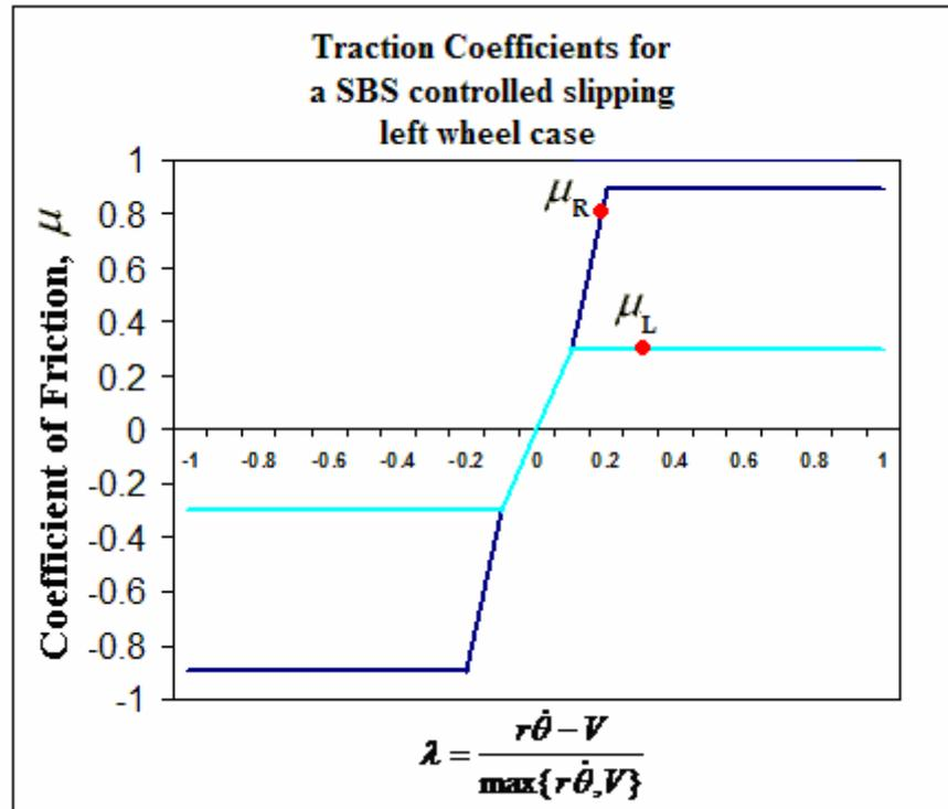
Figure 16b : Traction coefficient for the left and right wheel during a SBS controlled slipping left wheel.
