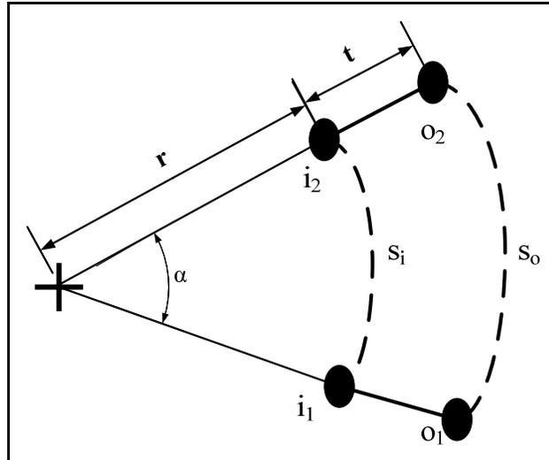
**Figure 1: Vehicle turning geometry used in DWSR derivation.**
