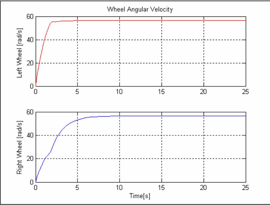
**Figure 13b: Wheel speeds for uncontrolled slip during initial acceleration and during a turning maneuver of  $\Phi = 245^\circ$  issued at  $t=10$  seconds and ending at  $t =15$  seconds.**
