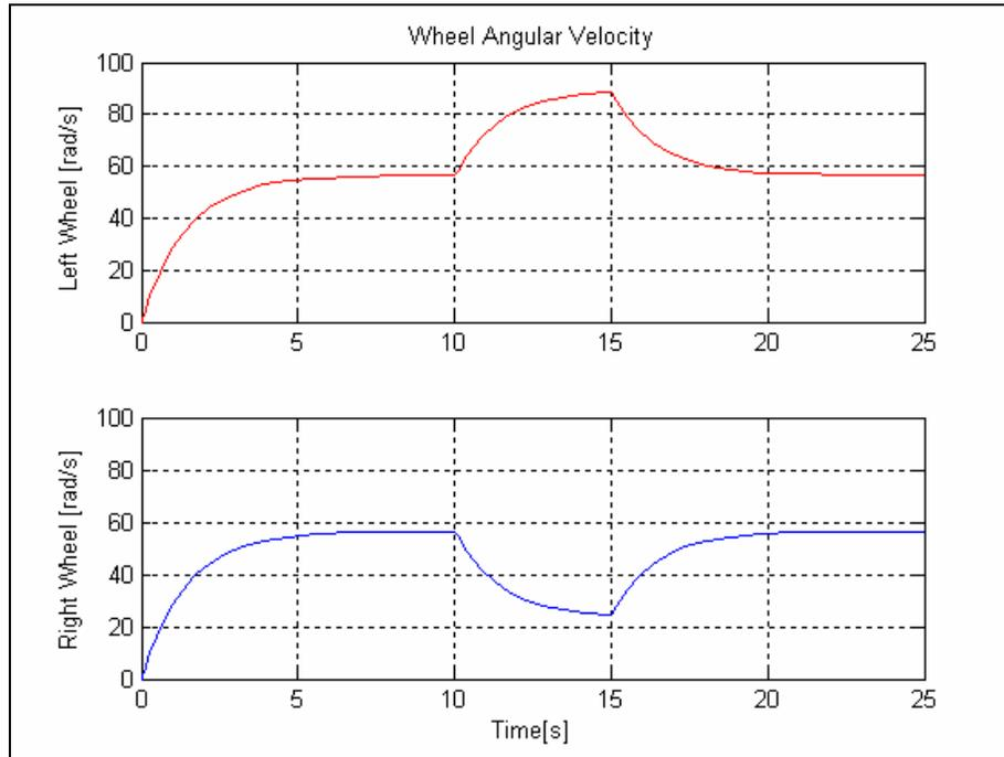
**Figure 10d: Straight travel with slipping of the left wheel.**
