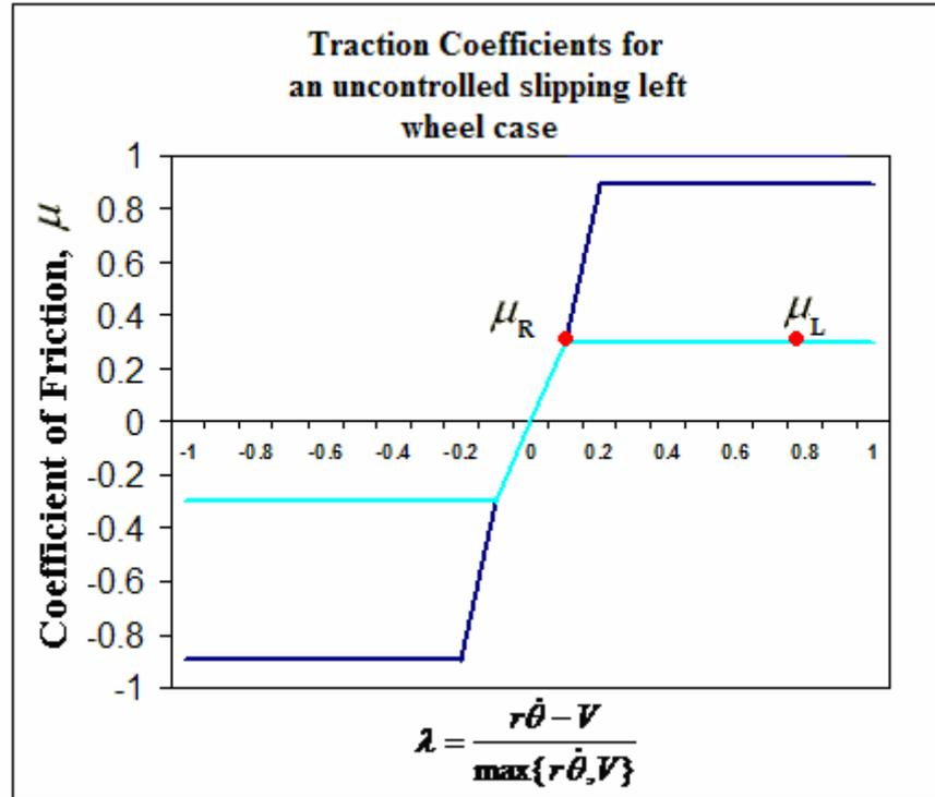
Figure 15b : Traction coefficient for the left and right wheel during an uncontrolled slipping left wheel.
