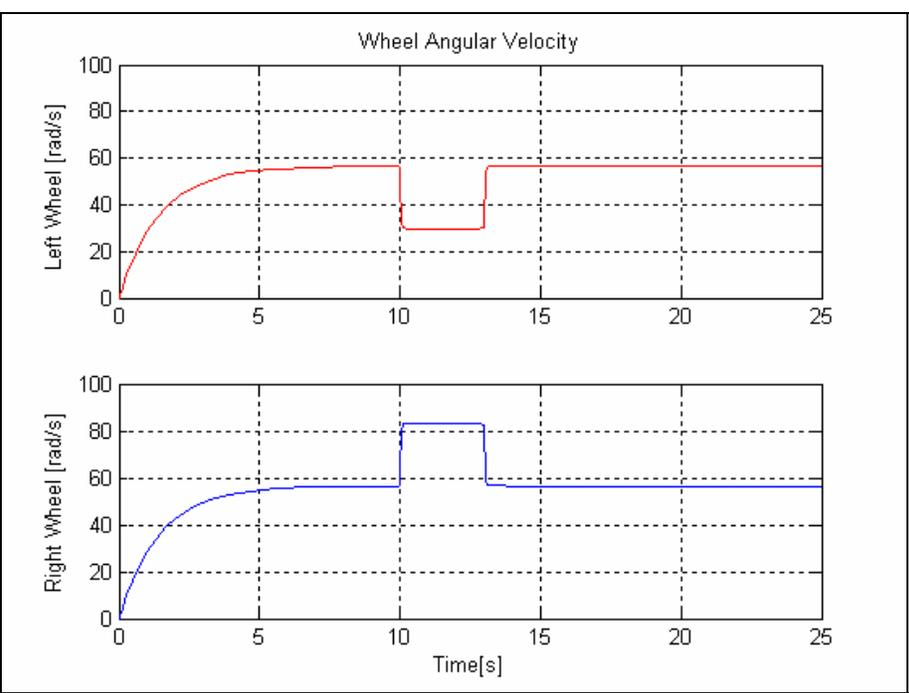
**Figure 12d: Wheel speeds during a controlled slip during a turning maneuver ( $\Phi = 100^\circ$ ).**
