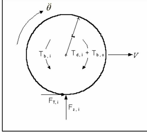
Figure 3: Free-body diagram of a quarter model of the vehicle wheels.
