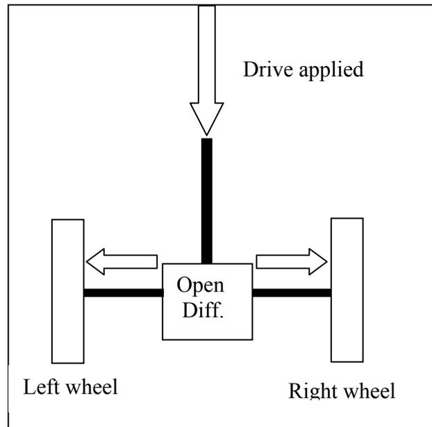
**Figure 14a: Drive torque distribution to the wheels with no slip.**
