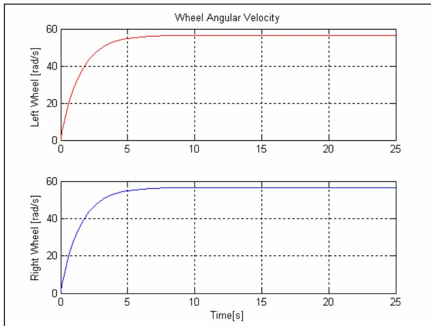
**Figure 11a: Straight line acceleration with no-slip at initial take off.**
