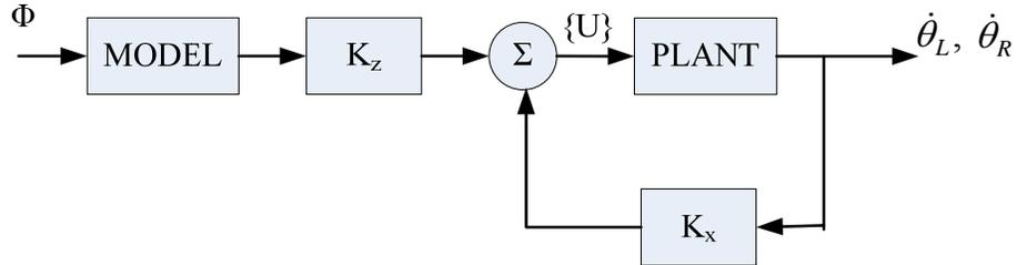
**Figure 7 : Control Loop of SBS**
