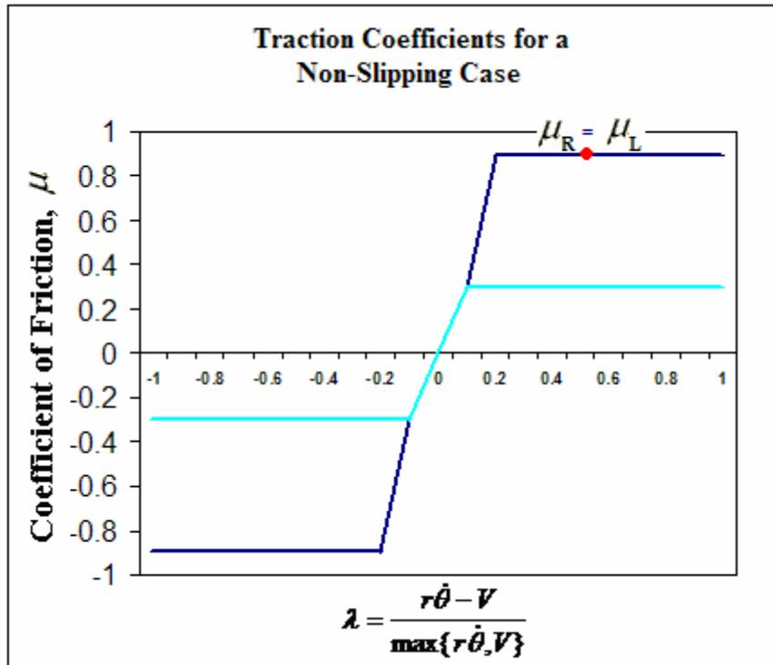
Figure 14b : Traction coefficient for the left and right wheel with no slip.
