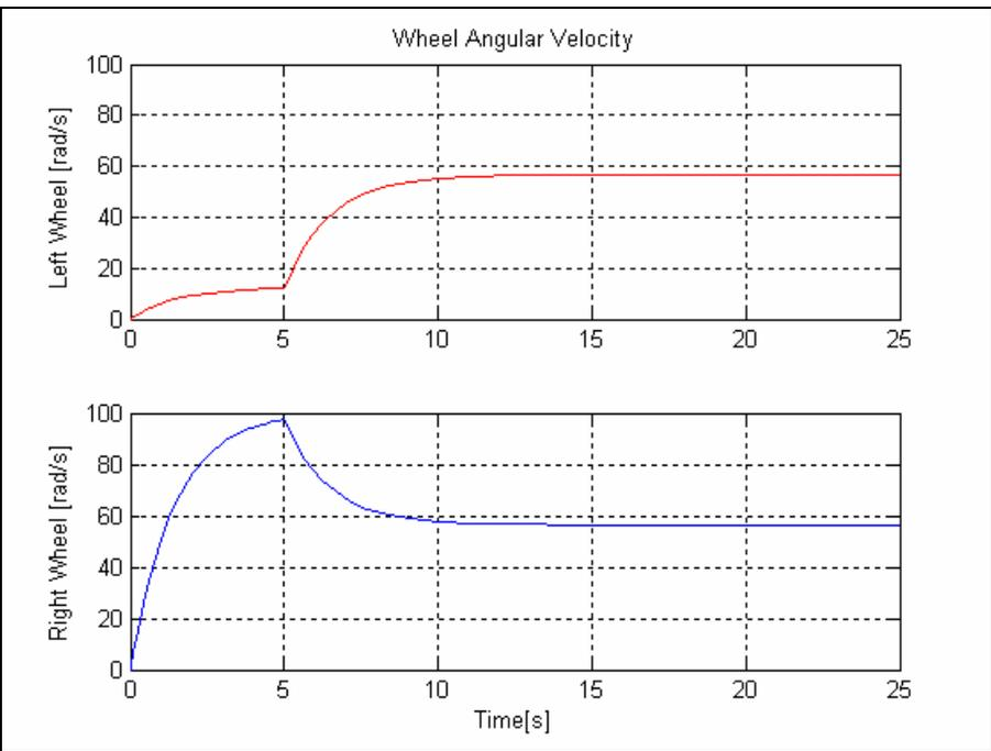
**Figure 11b: Straight line acceleration with the right wheel slipping at start.**
