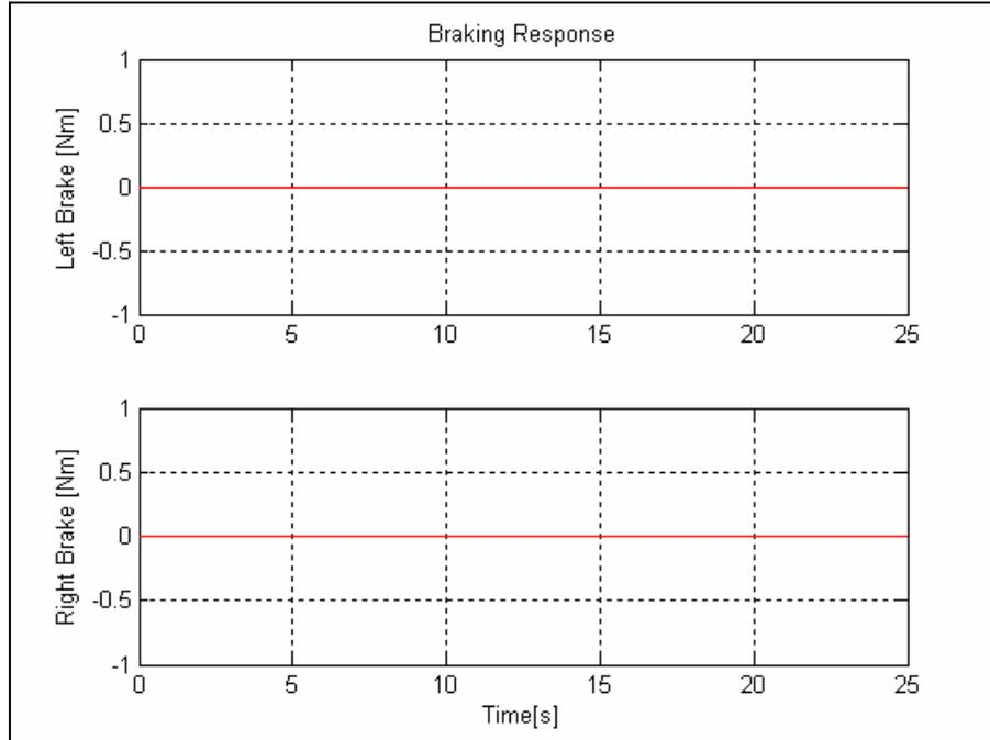
**Figure 10b: Brake response for straight travel with no slipping.**
