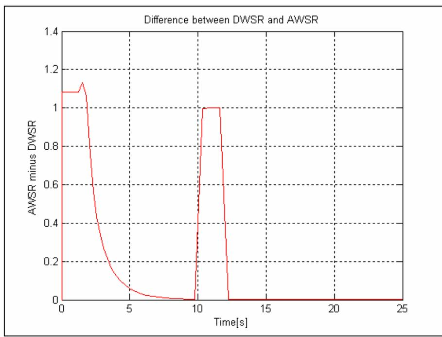
**Figure 13c: DWSR v. AWSR for an uncontrolled slip during initial acceleration and during a turning maneuver of  $\Phi = 245^\circ$  issued at  $t=10$  seconds and ending at  $t =15$  seconds.**
