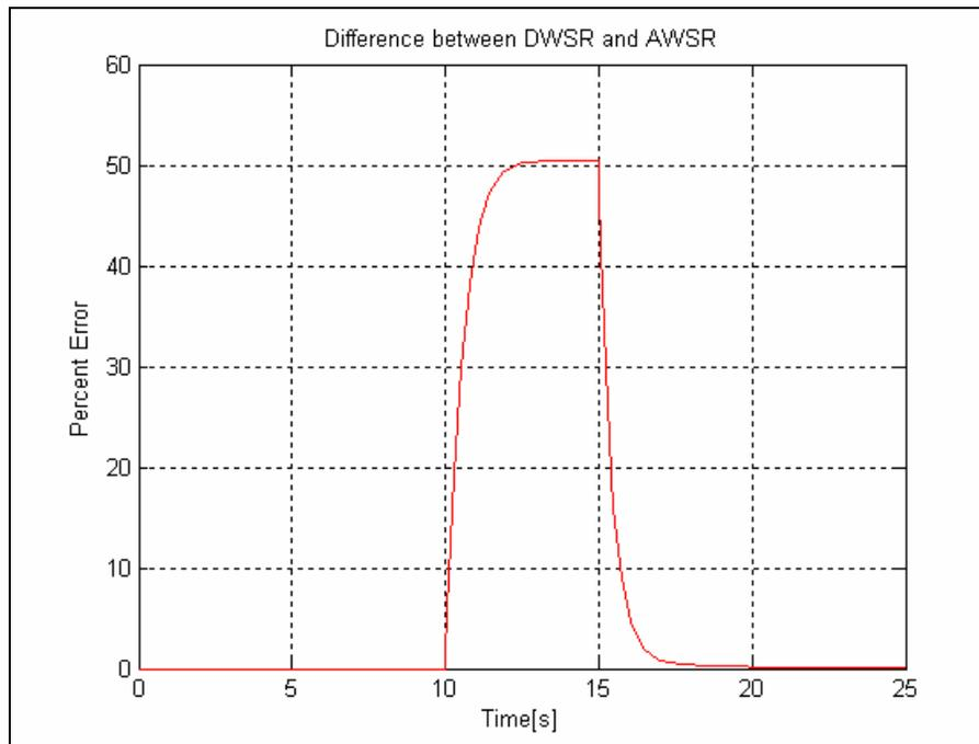
**Figure 10i: DWSR v. AWSR for a controlled straight travel with slip (State weighting of unity).**
