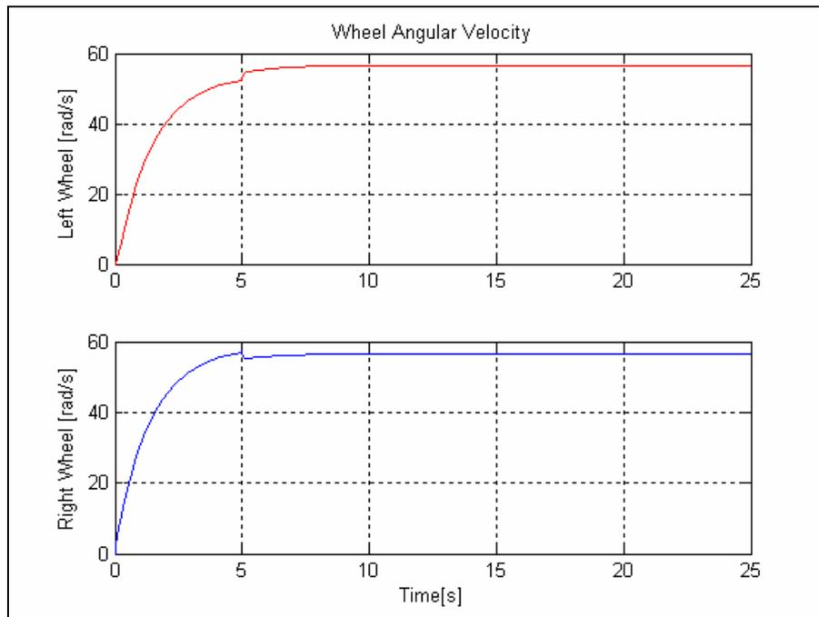
**Figure 11d: Wheel speeds for a controlled straight line acceleration with slip at start.**
