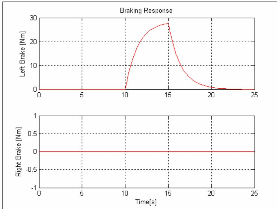
**Figure 10h: Braking response for a controlled straight travel with slip (State weighting of unity).**
