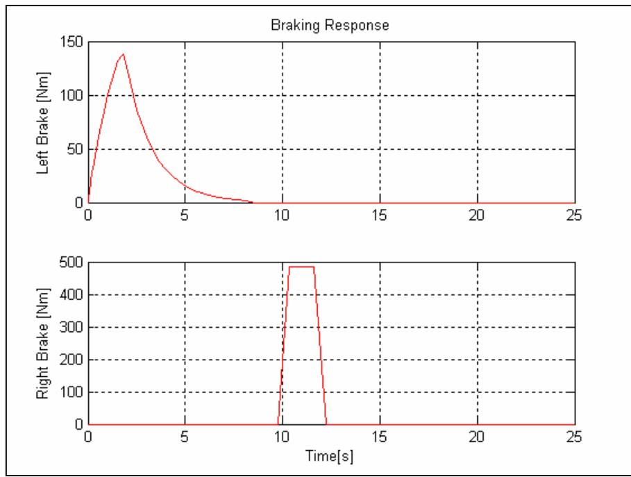
**Figure 13e: Braking response during a controlled slip situation during initial acceleration and during a turning maneuver of  $\Phi = 245^\circ$  issued at  $t=10$  seconds and ending at  $t=15$  seconds.**
