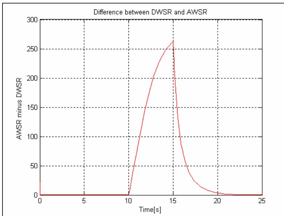
**Figure 10f: Difference between DWSR and AWSR for an uncontrolled straight travel with slip.**
