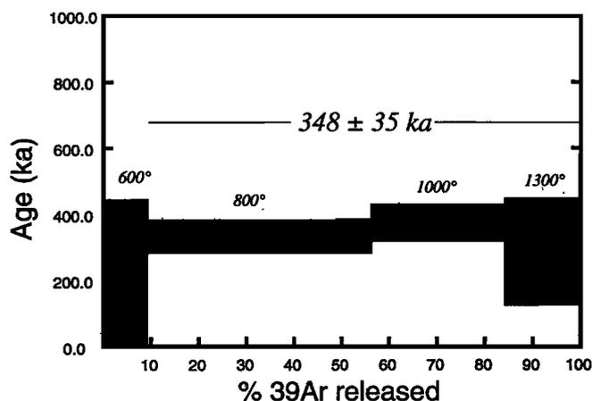
Figure 1. Age spectrum for incremental heating of submarine basalt PH117-2 from the East Pacific Rise ( $9^\circ 30' \text{N}$  to  $11^\circ 20' \text{N}$ ). Largely atmospheric Ar outgassed at low and high temperatures, while higher proportions of radiogenic  $^{40}\text{Ar}$  were released at  $800 \pm 200^\circ\text{C}$ .
