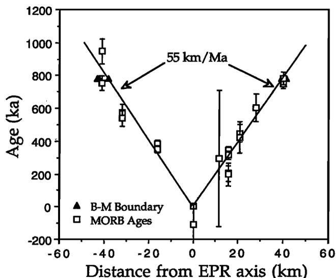
Figure 2. Radiometric ages measured by  $^{40}\text{Ar}$ - $^{39}\text{Ar}$  incremental heating experiments plotted against distance from the East Pacific Rise. In general, sample ages are concordant with those expected from location and the spreading rate, or interpolation between the Brunhes-Matuyama boundary and the spreading axis.
