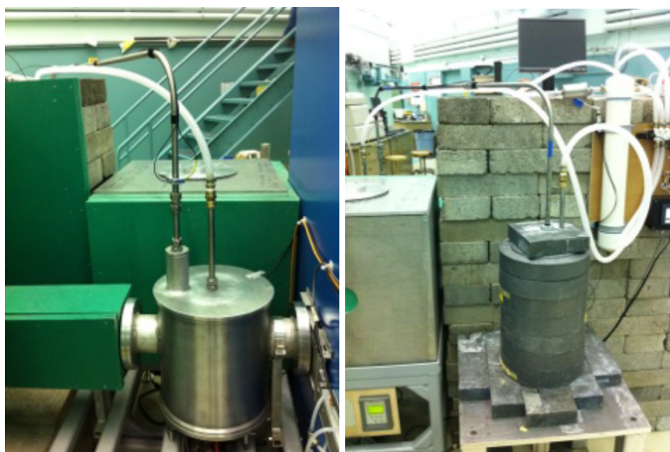
Figure 16: Photographs of the pneumatic transfer system and detector [64].
