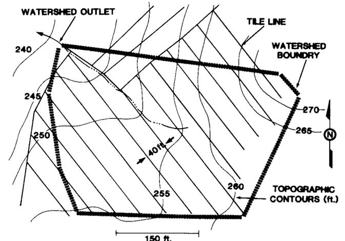
Fig. 3. Perforated plastic drain tube was installed at forty foot spacing covering a 2.3 acre sub-watershed.
