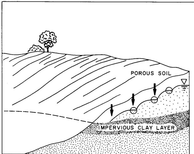
Fig. 1b. A more rapid lowering of the water table can prevent saturation induced runoff.
