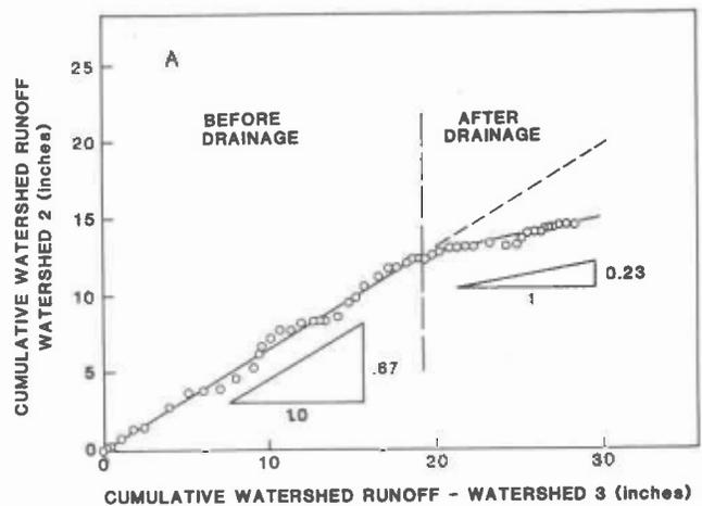
Fig. 5a. Relative water runoff was reduced 65% by drain installation.
