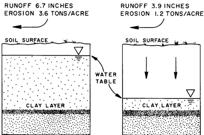
Fig. 2. Measurements in Polk county have demonstrated enhanced runoff and erosion associated with high (near the soil surface) perched water tables.
