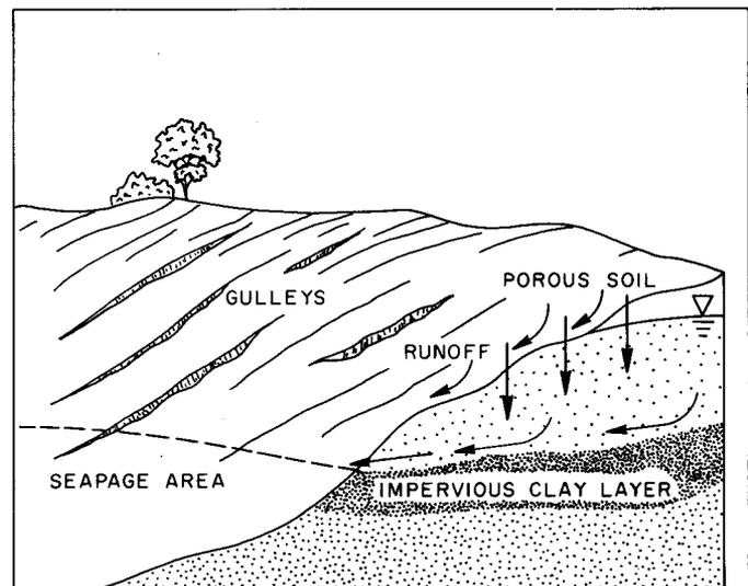
Fig. 1a. When infiltrating water reaches a relatively impervious layer, the temporary water table may rise to the soil surface. Then runoff occurs even when there is no concurrent rainfall.
