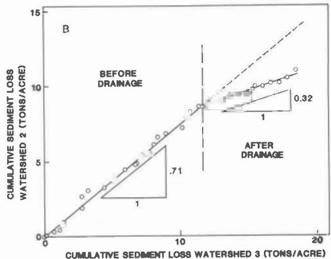
Fig. 5b. Relative erosion was reduced 50% by drain installation.
