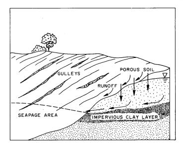
Fig. la. When infiltrating water reaches a relatively impervious layer, the temporary water table may rise to the soil surface. Then runoff occurs even when there is no concurrent rainfall.
