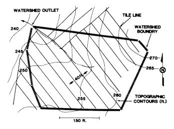
Fig. 3. Perforated plastic drain tube was installed at forty foot spacing covering a 2.3 acre sub-watershed.
