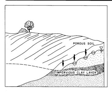
Fig. 1b. A more rapid lowering of the water table can prevent saturation induced runoff.
