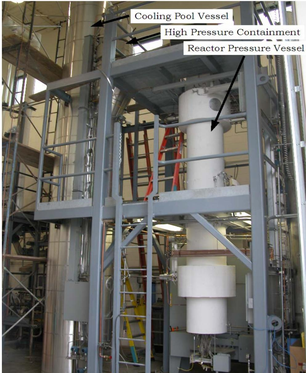
Figure 3.0-1: First level view of the MASLWR Test Facility.
