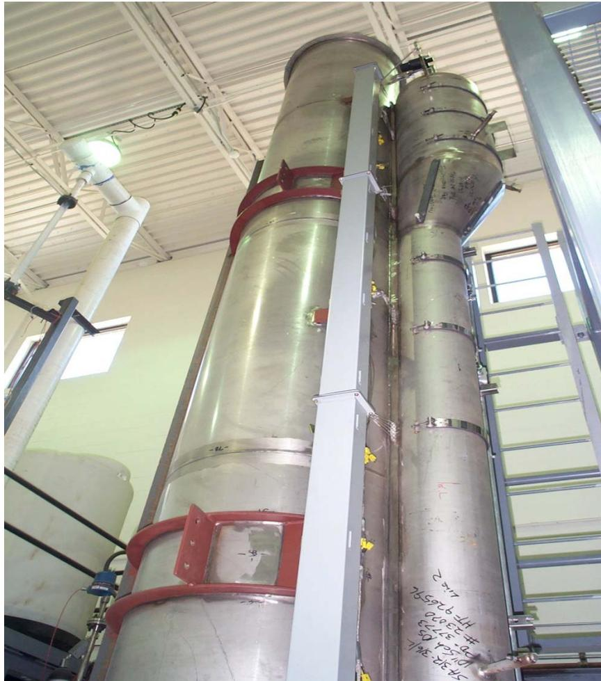
Figure 3.2-1: OSU MASLWR Test Facility Containment and Cooling Pool Vessels without insulation.
