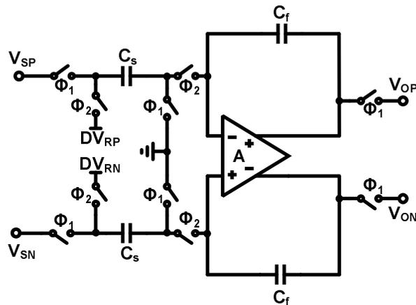
Figure 2.4: Integrator with shared input and DAC capacitor
