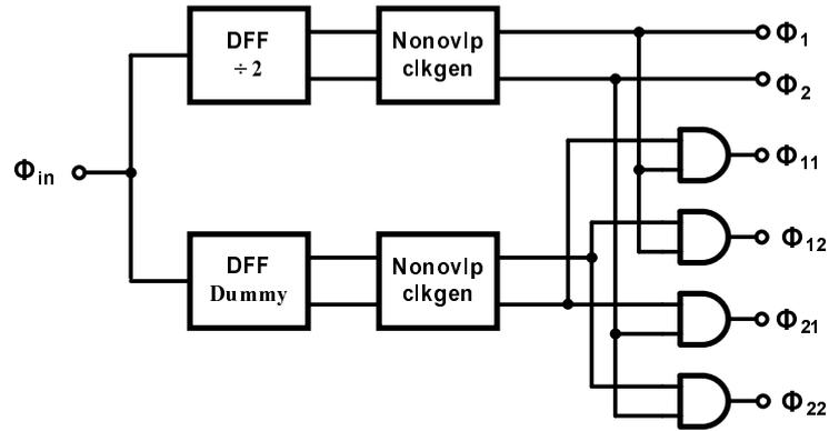
Figure 4.16: Four phase clock generator
