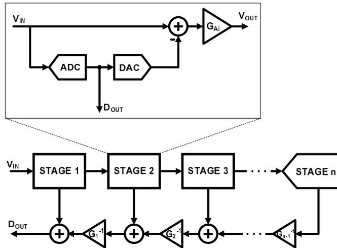
Figure 2.7: Pipelined ADC
