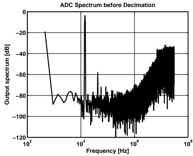
Figure 6.11: Output spectrum of modulator at 1.1V
