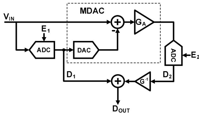
Figure 2.6: Two-step ADC
