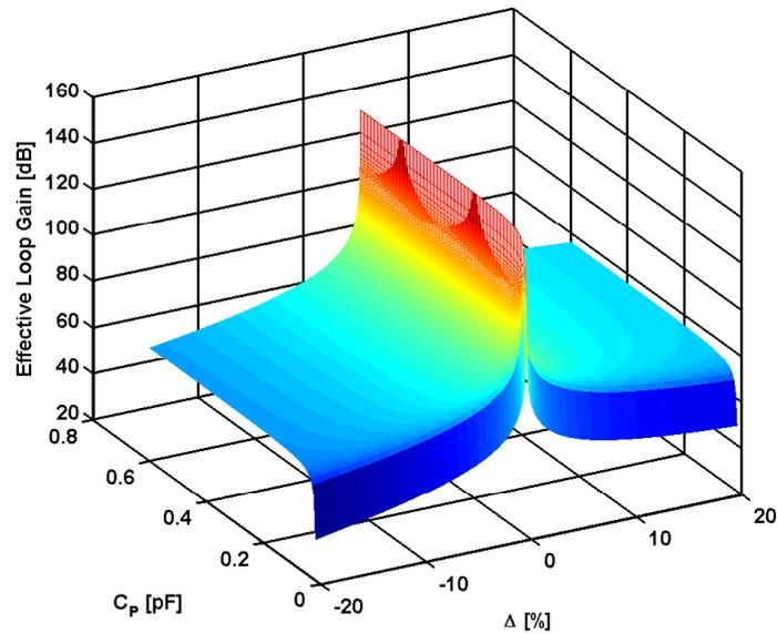
Figure 4.5: Effect of  $C_P$  on Accuracy
