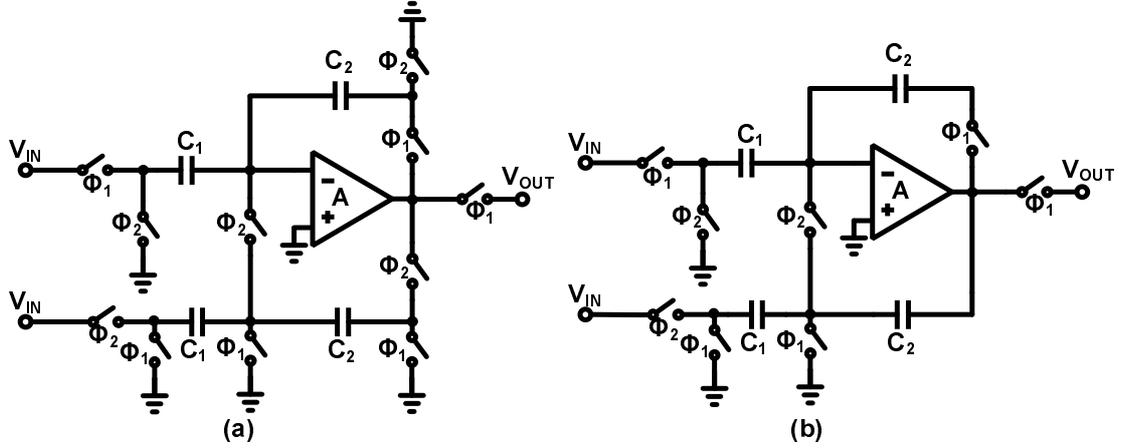
Figure 3.6: Larson CDS (a)gain stage and (b)integrator
