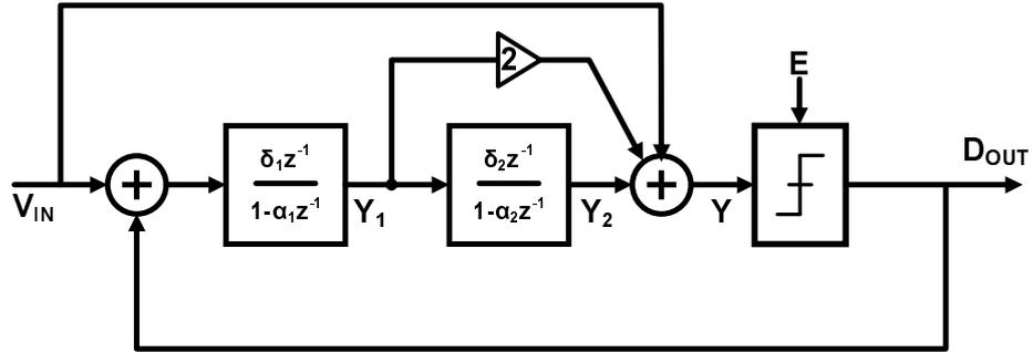
Figure 2.9: Delta-sigma ADC
