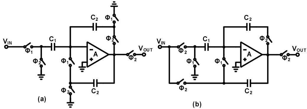
Figure 3.5: Haug CDS (a)gain stage and (b)integrator
