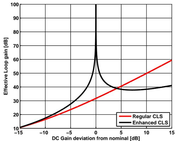
Figure 4.4: Sensitivity of loop gain to DC gain variation
