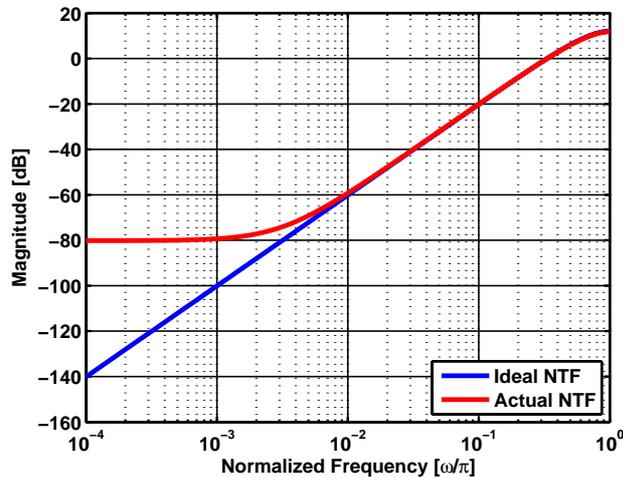
Figure 2.10: Effect of amplifier gain on noise shaping
