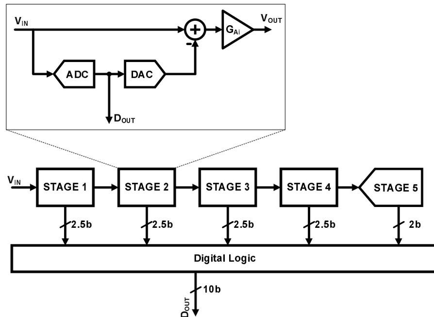
Figure 4.7: Pipelined ADC block diagram
