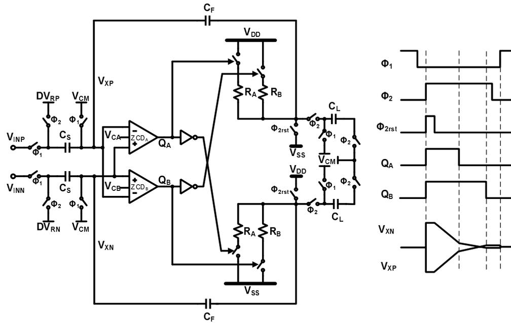
Figure 6.6: Zero-crossing-based integrator
