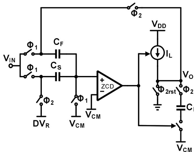
Figure 6.1: Comparator-based MDAC
