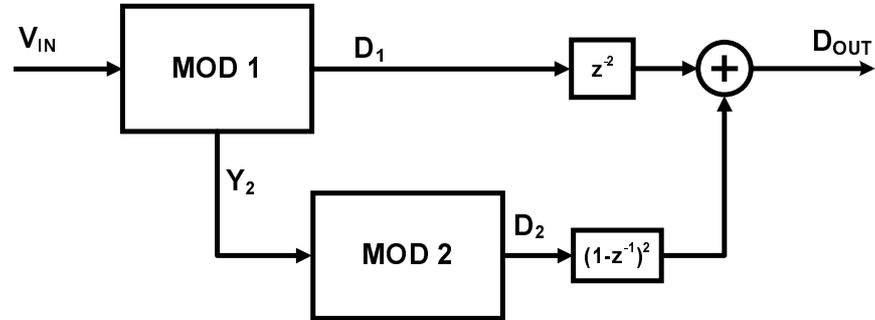
Figure 2.11: Two-stage MASH ADC
