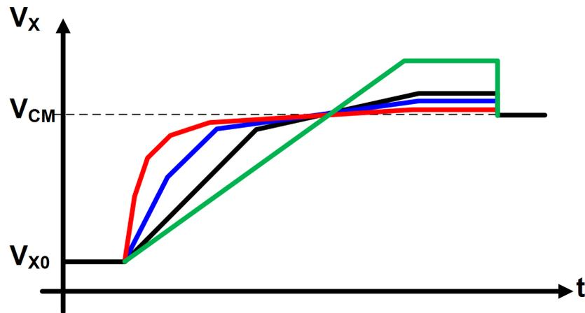
Figure 6.4: Multi-rate charging scheme
