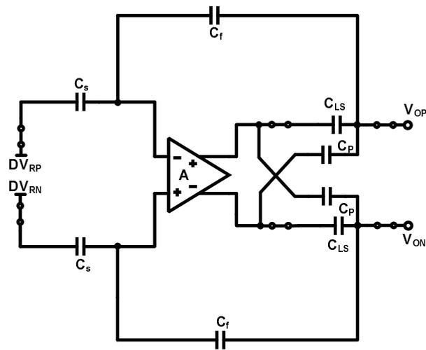
Figure 4.3: Cross-Coupled CLS MDAC - Level Shifting
