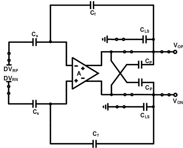
Figure 4.2: Cross-Coupled CLS MDAC - Estimation
