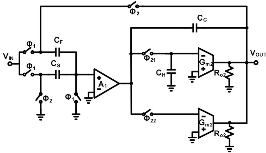
Figure 3.4: Replica gain enhanced gain stage
