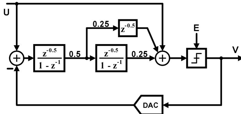
Figure 6.7: 2nd order feedforward  $\Delta\Sigma$  modulator
