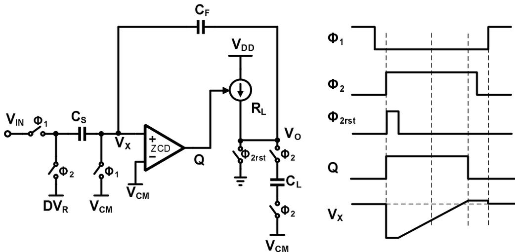
Figure 6.3: Zero-crossing-based Integrator
