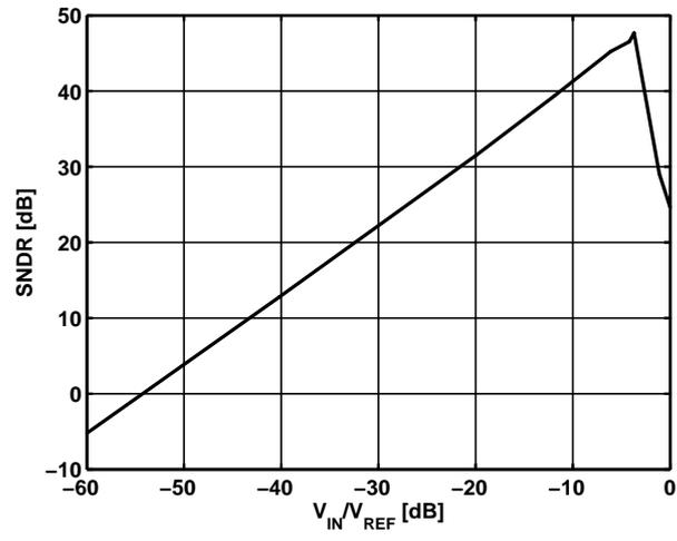
Figure 6.13: SNR vs input level at 1.1V
