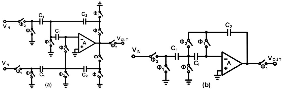
Figure 3.7: Nagaraj CDS (a)gain stage and (b)integrator
