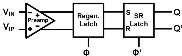
Figure 6.9: Zero-crossing detector circuit
