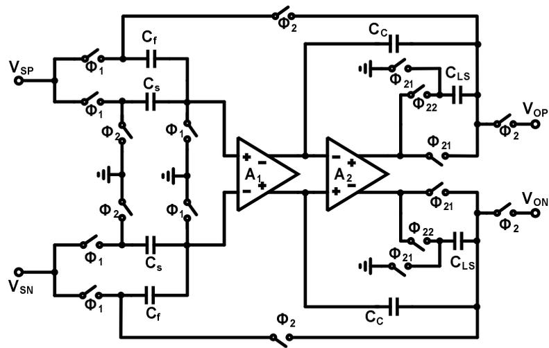
Figure 3.10: CLS MDAC with two-stage amplifier
