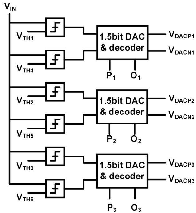
Figure 4.12: 7 level quantizer
