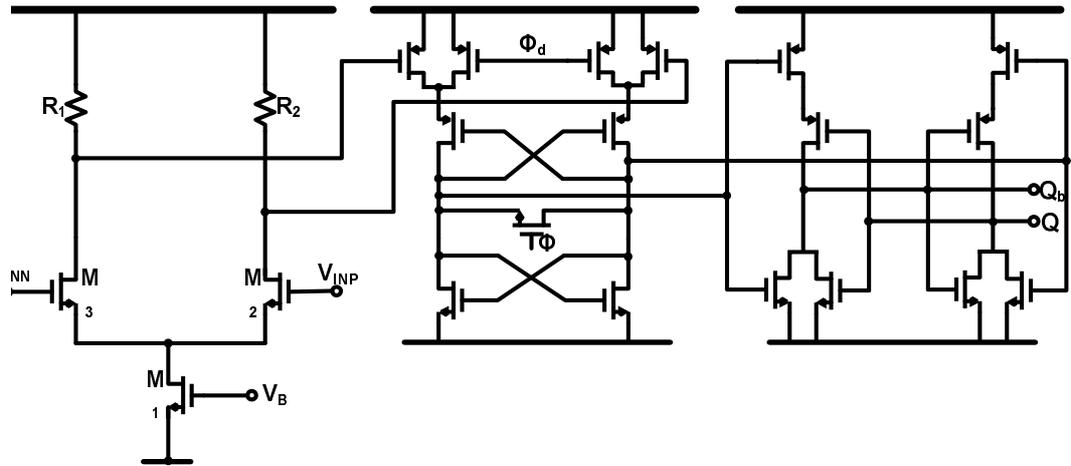
Figure 4.15: Comparator schematics
