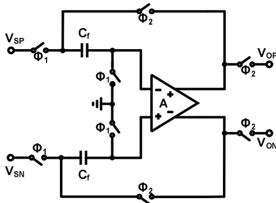
Figure 2.2: Flip-around sample-and-hold
