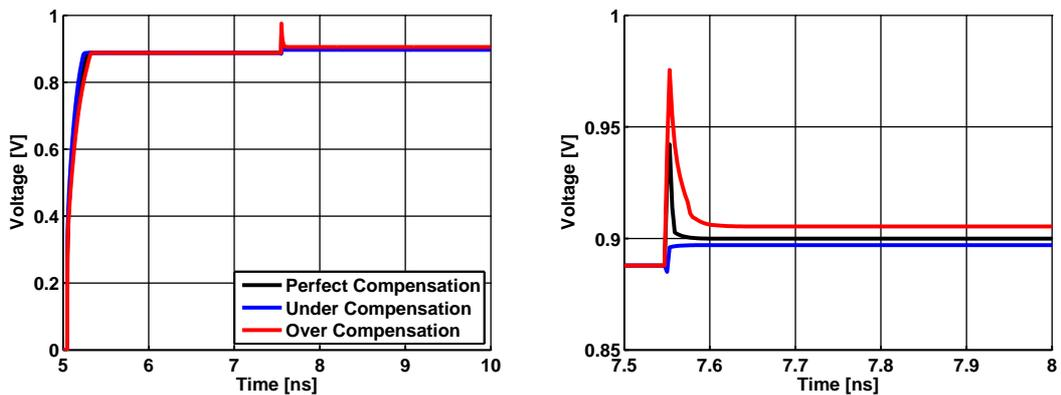
Figure 4.6: Settling response of CLS MDAC
