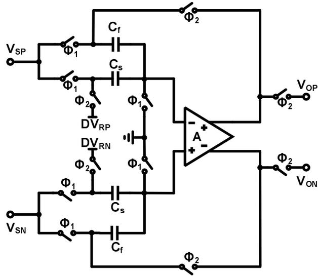
Figure 2.3: Flip-around multiplying digital-to-analog converter
