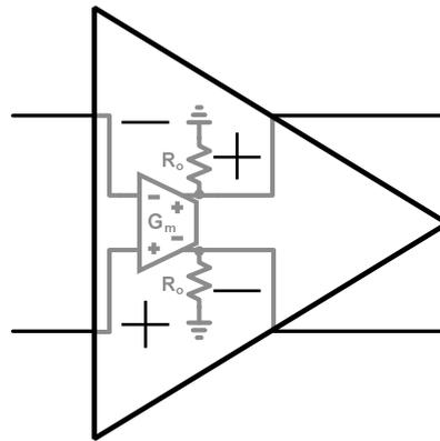
Figure 2.1: Representation of operational transconductance amplifier
