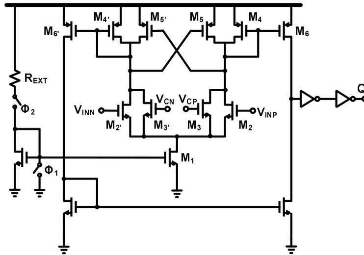
Figure 6.8: Zero-crossing detector
