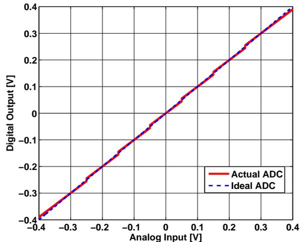
Figure 2.8: Effect of gain error in pipelined ADC linearity
