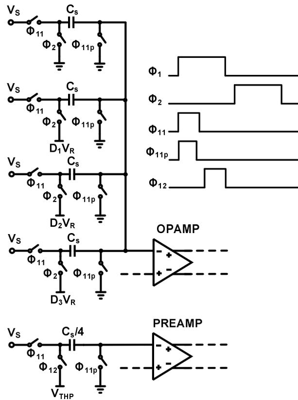
Figure 4.8: SAH-less sampling configuration
