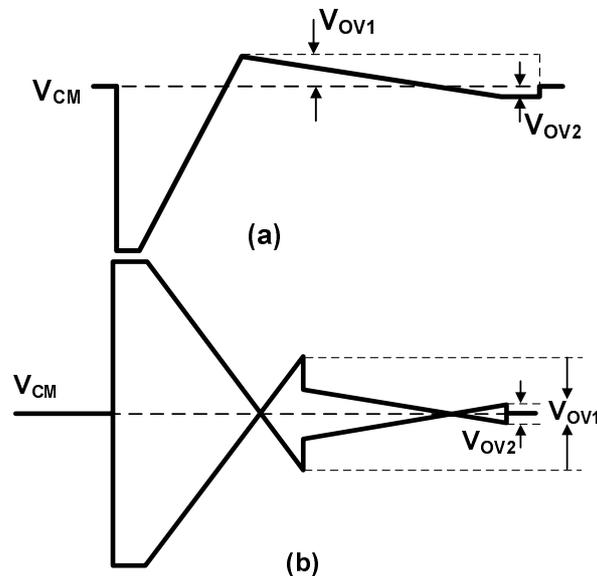
Figure 6.2: Effect of Coarse-fine on overshoot
