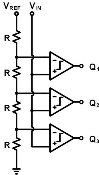
Figure 2.5: 2-bit flash ADC
