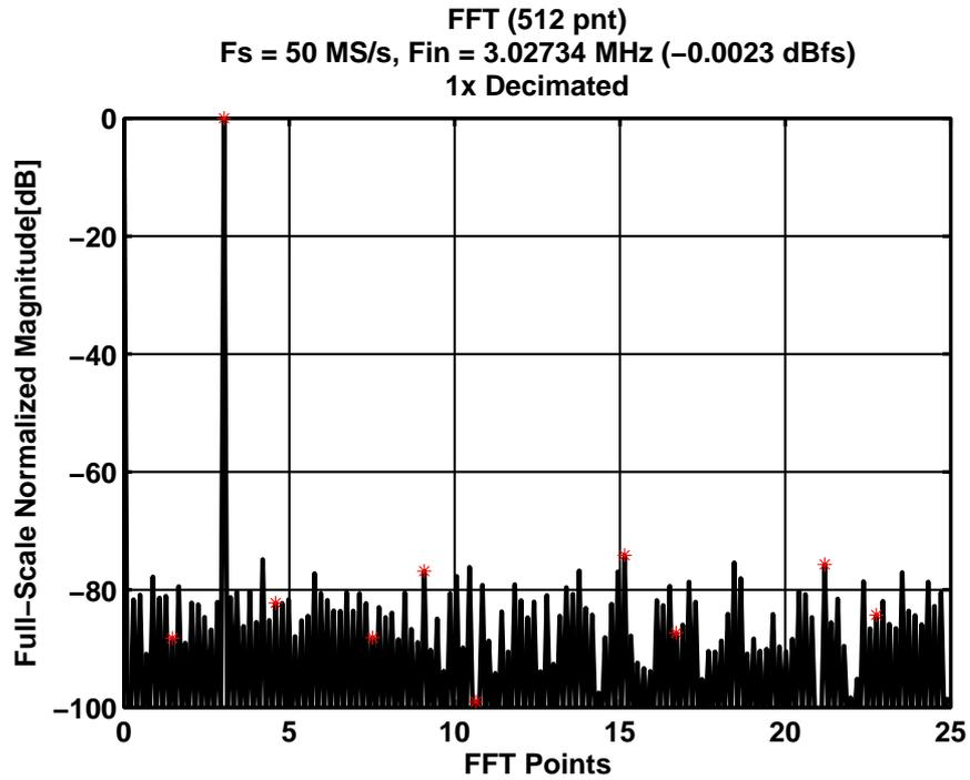
Figure 4.20: ADC output spectrum
