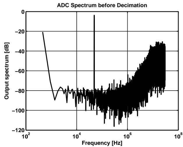
Figure 6.12: Output spectrum of modulator at 1.2V
