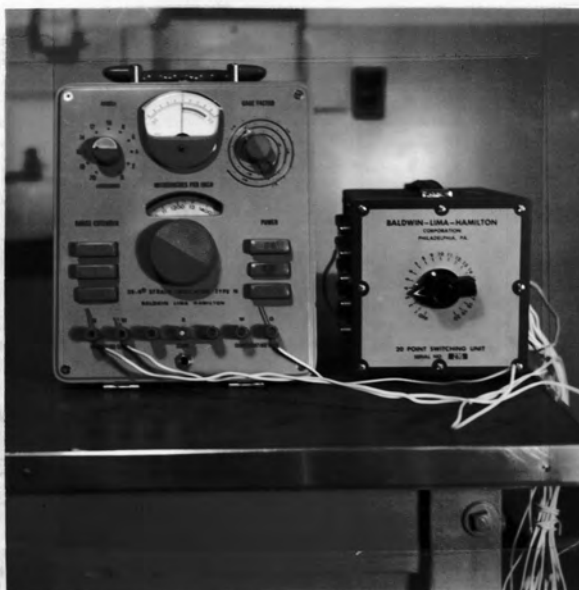
Plate 7. Strain Indicator and Switching Unit
