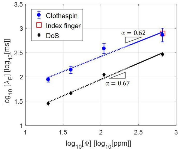
**Figure 5.** Extensional relaxation time,  $\lambda_E$ , plotted against PEO concentration,  $\Phi$ , on a log-log scale for the smartphone method with a clothespin (blue circles) and the ODES-DOS method (black diamonds). The slope,  $\alpha$ , for the smartphone analysis was similar to that of the ODES-DOS analysis. Error bars represent standard deviation with  $n=10$ . One point is shown for the finger method (red square) to show the similarity of results to the clothespin method.
