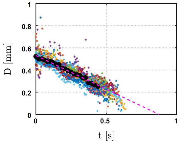
**Figure 7.** Diameter decay of Newtonian 4870 mPa·s silicone oil. Black points represent an average decay profile from 15 trials. Dashed line is the linear fit of the data used to represent Equation (4).
