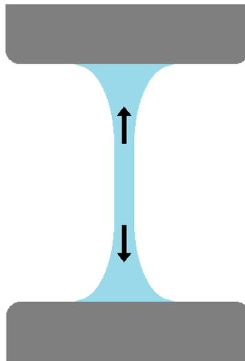
**Figure 1.** Schematic of capillary forces within a liquid bridge moving fluid to the bulk regions on each of the plates used to pull the fluid apart such as is done in a CaBER.
