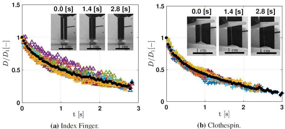
**Figure 3.** Profiles for diameter decay with time and the average of ten trials (black dots) for the finger method (a) and the clothespin method (b). Both methods show similar profiles but the noise, or variation, in the finger method is much greater.
