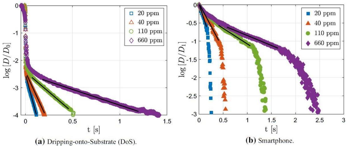
**Figure 4.** Log of diameter decay plotted at various concentrations of PEO according to Equation (2) for the ODES-DOS (a) and the smartphone (b). Data shown are averages of 10 trials for each fluid. Black lines show a linear fit for the exponential decay regime. Both methods are sensitive to small changes in polymer concentration.
