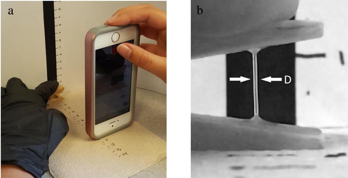
**Figure 2.** Experimental setup for filament thinning analysis using an iPhone SE. The phone is rested upside-down on the table to allow for close proximity of the camera lens to the sample (a). The high-speed camera is used to capture video of the liquid bridge decaying with time (b).
