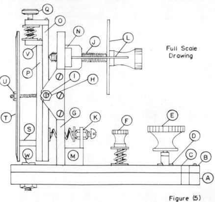
use of a lock nut to hold them in position in H. The set screw J is used to tilt the holder about the Z axis against the pressure produced by spring K. The scale on the head L is divided into fifty divisions, the pitch of the thread being one millimeter. The supports at M and N were made respectively of three-eighths and half inch square stock.
