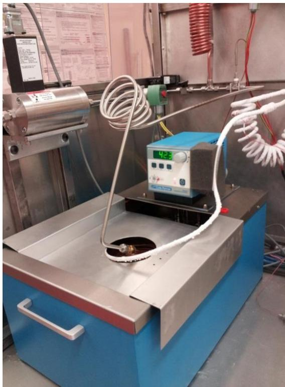
*Figure 18. Heater bath connected prior to the mass flow meter*
