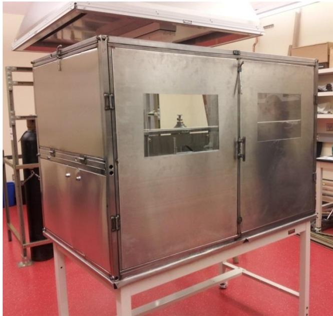
*Figure 12. Sheet metal shroud enclosing the test facility. The facility is located under the hood shown in the picture.*
