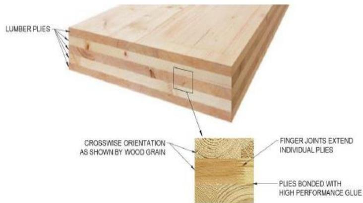
Figure 2. 1 Schematic of CLT panel (Kordziel, 2018)
