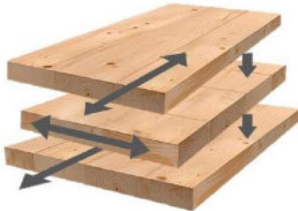
Figure 4. 1 Schematic of CLT layers (Mallo and Espinoza, 2014)
