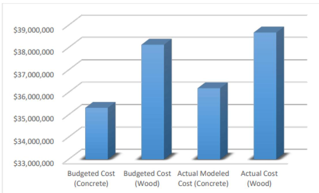
Figure 4. 2 Budgeted and actual construction cost of concrete and mass timber
