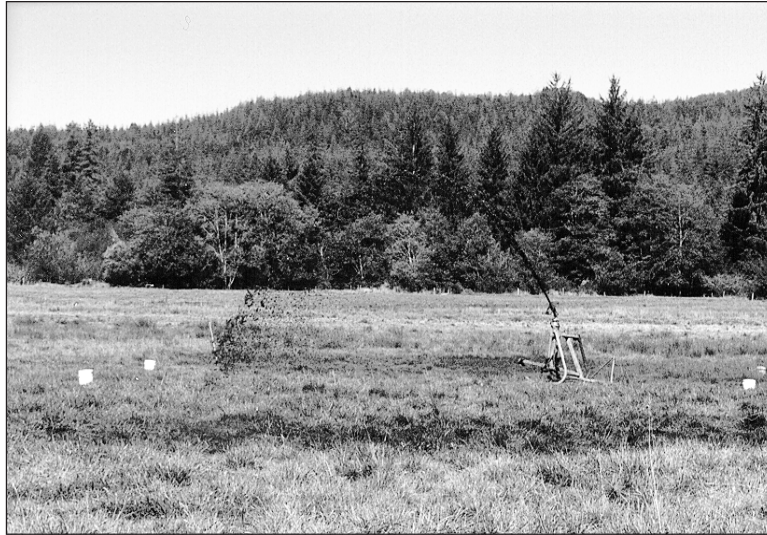
Figure 1. Place several straight-sided, flat-bottom buckets in the area where the gun is to apply liquid.
