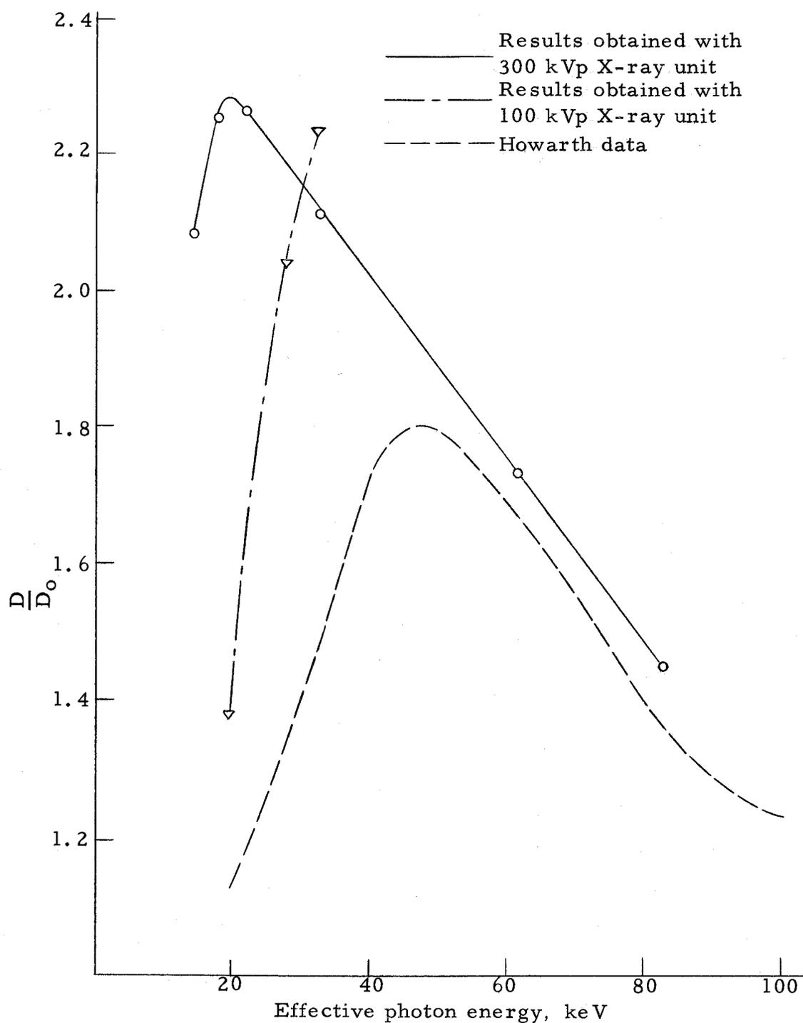
Figure 16. Increased X-ray dose in a 13.2 micron soft tissue layer located adjacent to a plane, semi-infinite slab of bone, as a function of effective X-ray energy. Comparison of results obtained with both the 100 kVp and 300 kVp X-ray units with theoretical data of Howarth (1965).
