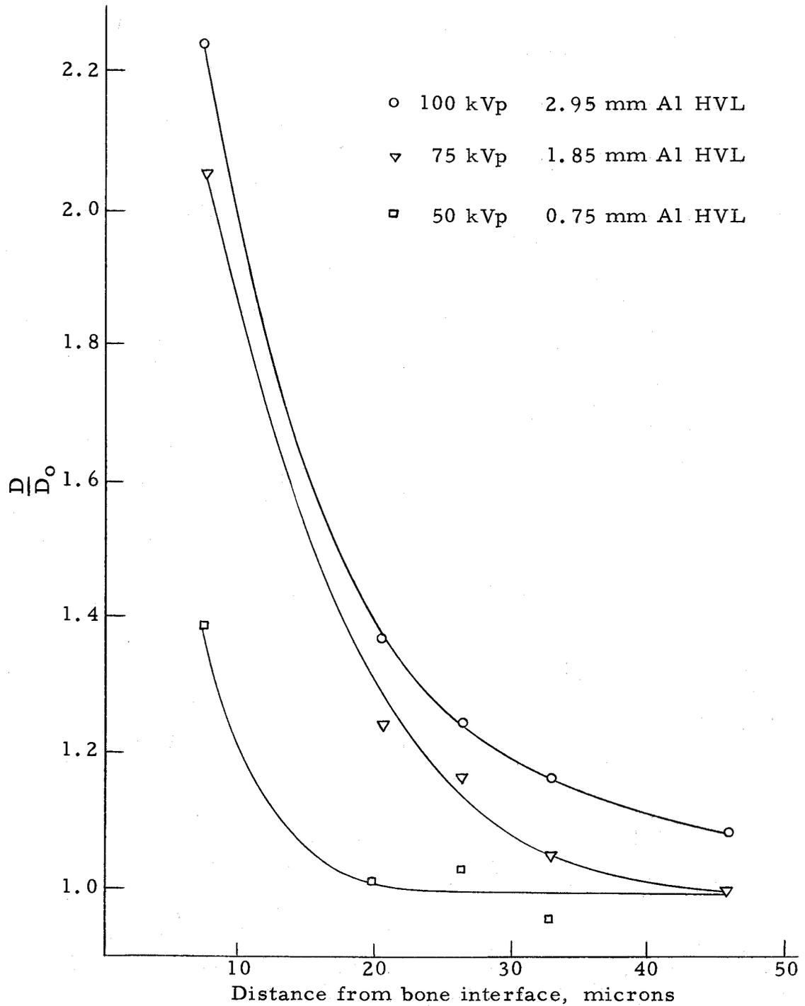
Figure 12. Increased X-ray doses in soft tissue adjacent to plane, semi-infinite slabs of bone--100 kVp X-ray unit.
