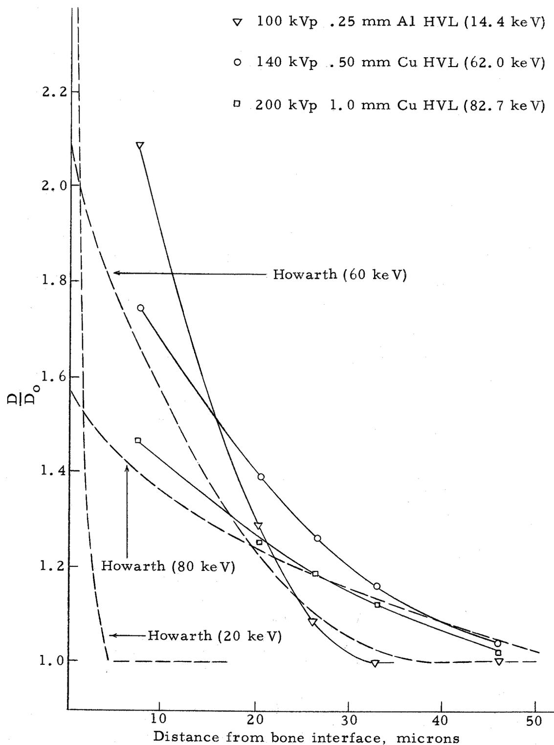
Figure 14. Increased X-ray doses in soft tissue adjacent to plane, semi-infinite slabs of bone. Comparison of results obtained with 300 kVp X-ray unit, solid curves, with Howarth (1965) data, dotted curves.
