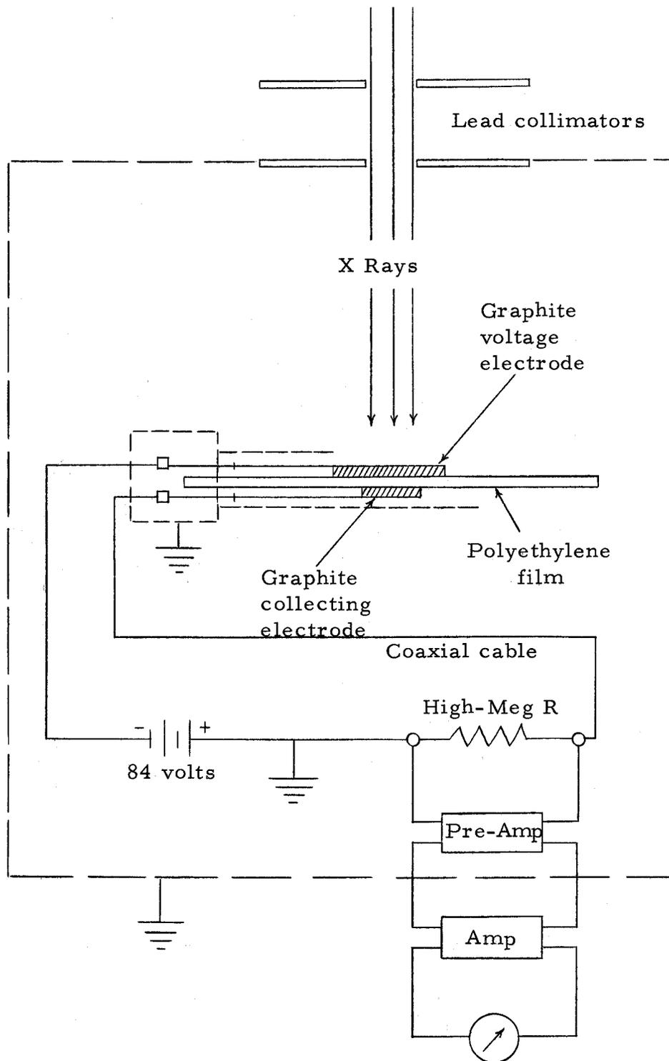
Figure 2. Diagram of circuit used to measure the radiation induced conductivity of polyethylene. Guard circuits are denoted by dotted lines.
