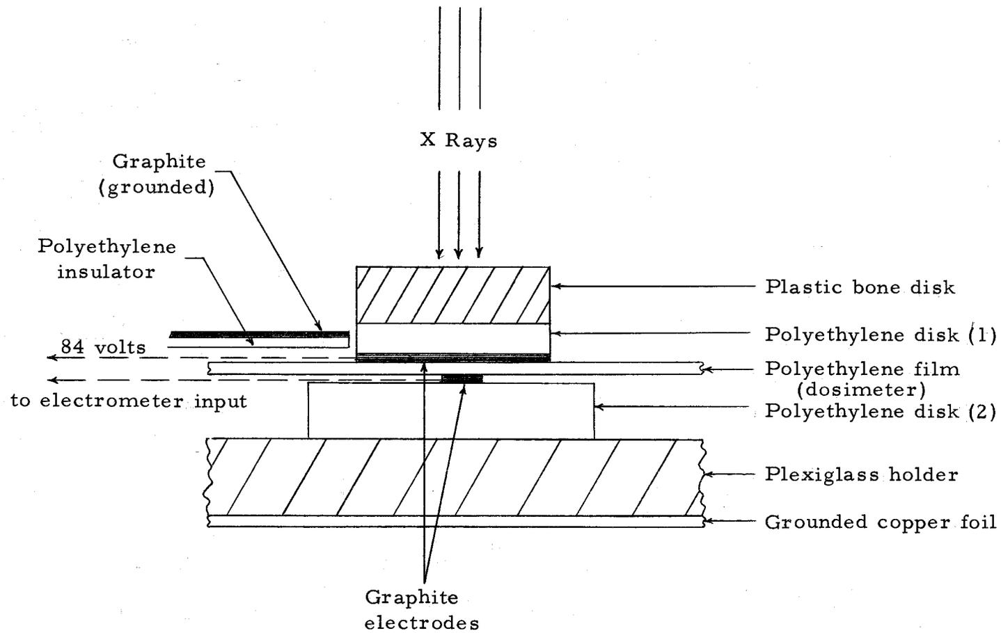
Figure 7. Apparatus used to simulate plane bone-soft tissue interfaces. Guard electrodes are also shown.
