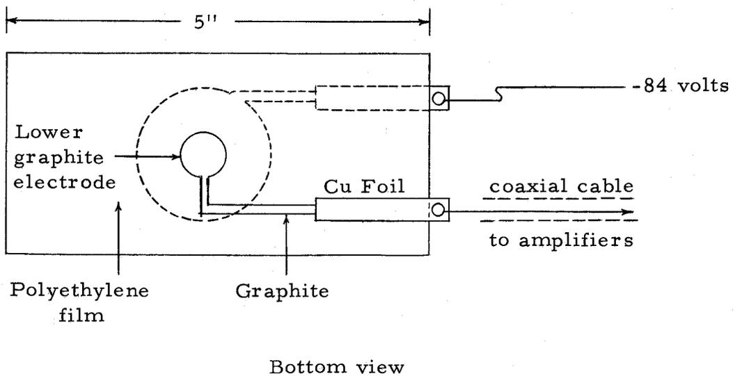
Figure 1. Diagram of polyethylene-film dosimeter showing film, electrodes, and lead-in strips.
