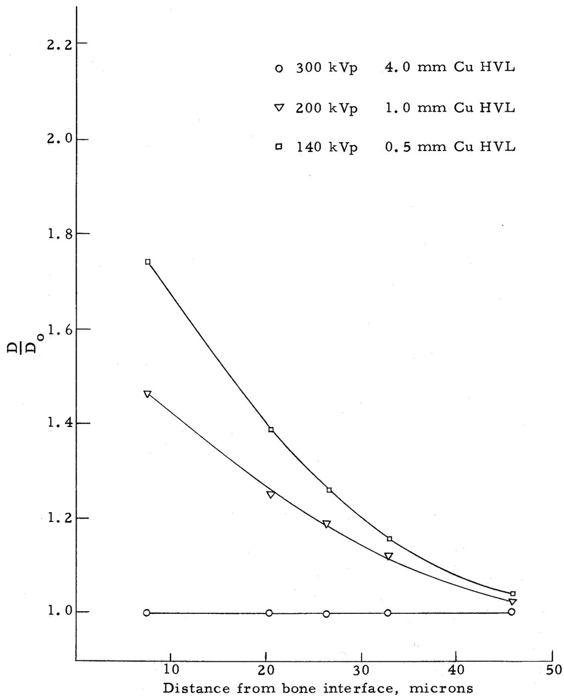
Figure 10. Increased X-ray doses in soft tissue adjacent to plane, semi-infinite slabs of bone--300 kVp X-ray unit.
