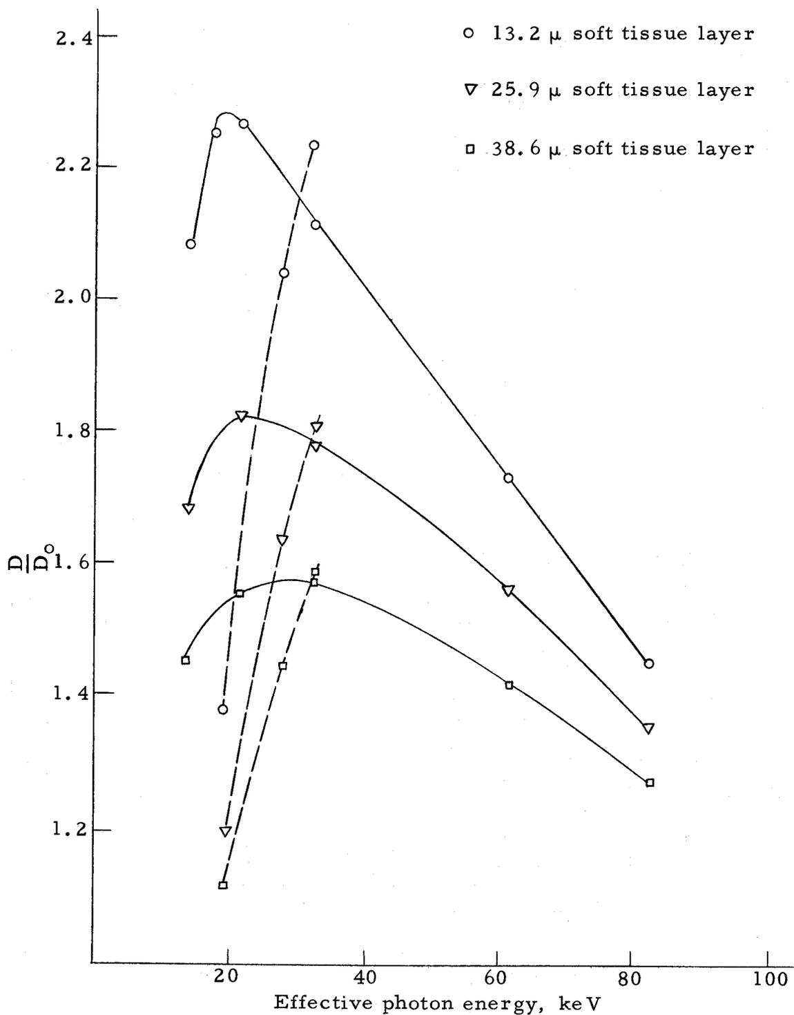
Figure 13. Increased X-ray doses in soft tissue layers of finite dimensions located adjacent to plane, semi-infinite slabs of bone shown as a function of effective photon energy--100 kVp X-ray unit, dotted curves; and 300 kVp X-ray unit, solid curves.
