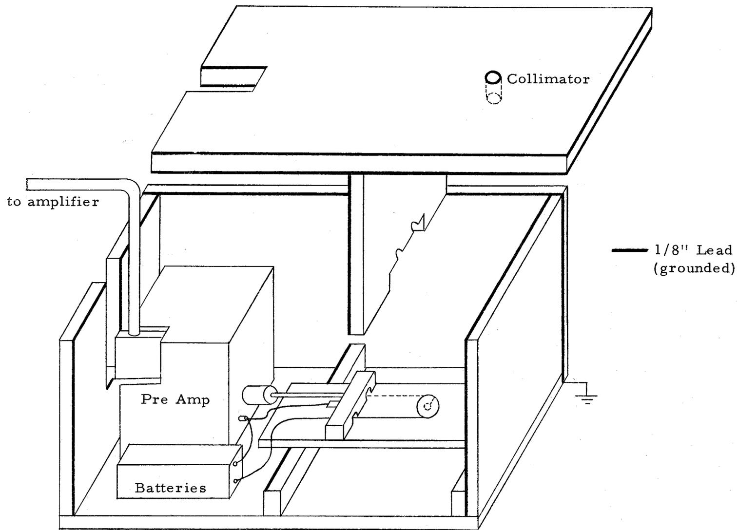
Figure 4. Complete apparatus shown housed in lead shielded Faraday cage.
