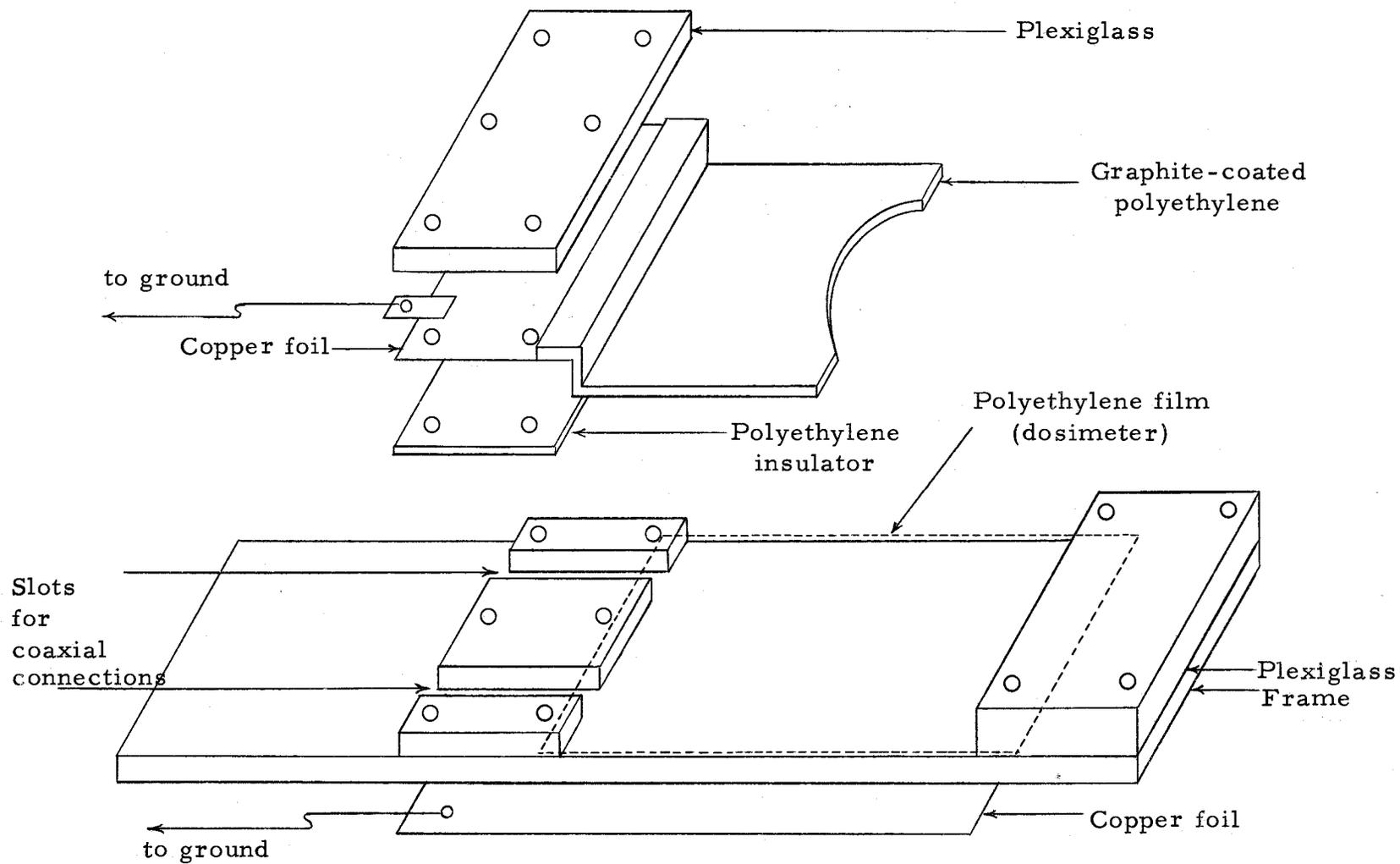
Figure 3. Apparatus for holding polyethylene-film dosimeter. Guard electrodes are shown.
