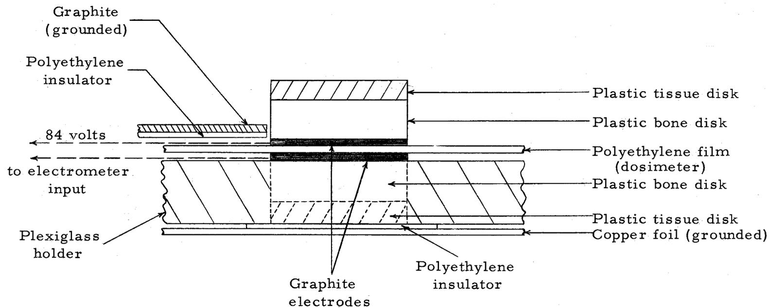
Figure 9. Apparatus used to simulate a parallel-slab soft tissue cavity in bone. Guard electrodes are also shown.
