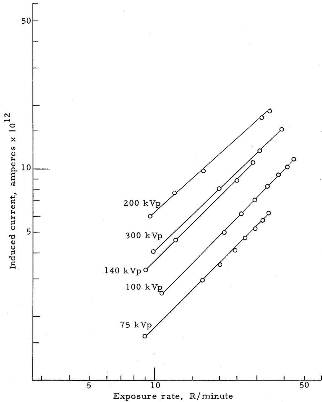
Figure 6. Induced current in polyethylene as a function of X-ray exposure and X-ray energy.
