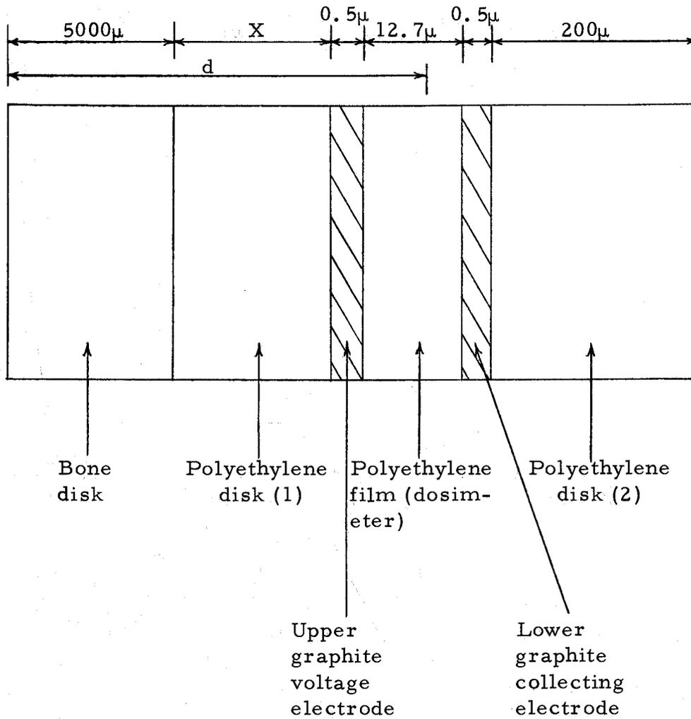
Figure 8. Diagram showing dimensions of the components of the simulated plane bone-soft tissue interface.
