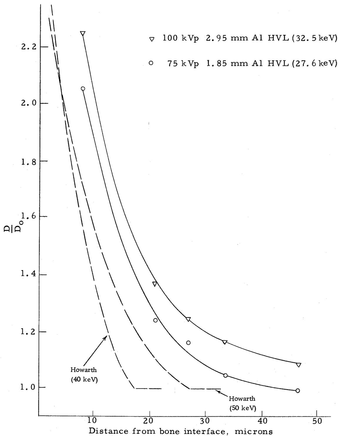
Figure 15. Increased X-ray doses in soft tissue adjacent to plane, semi-infinite slabs of bone. Comparison of results obtained with 100 kVp X-ray unit, solid curves, with Howarth (1965) data, dotted curves.
