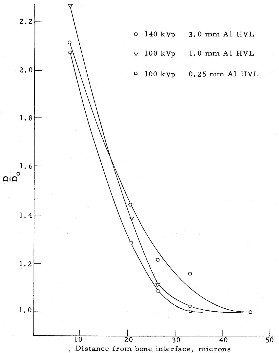
Figure 11. Increased X-ray doses in soft tissue adjacent to plane, semi-infinite slabs of bone--300 kVp X-ray unit.
