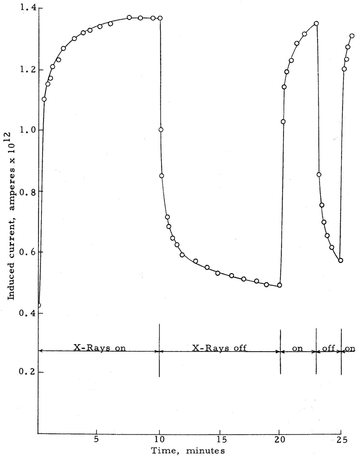
Figure 5. Relationship between induced current in polyethylene and time during which X rays are off and on. Exposure rate of 10 Roentgen/min.
