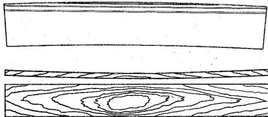
Fig. 4. Warp From Crooked Log
