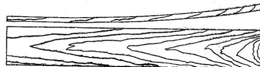
Fig. 6 Bow in Board Sawn Parallel to Pith
