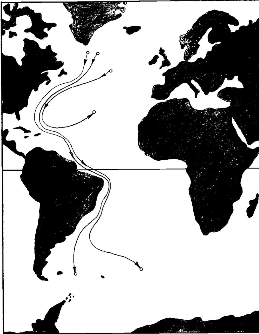
Figure 7. A possible interpretation of total transports in Atlantic bottom layer. Areas of sinking and upwelling are indicated by little circles. Net transport across the equator is 16 Sv. (From Stommel)
