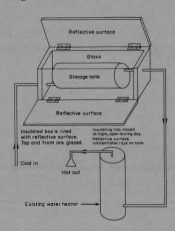
The cold water supplied to the tank is pre-heated by the sun (collection) where it remains (storage) until hot water is drawn from a household faucet (control). The pre-heated water moves to a conventional water heater where it is heated to the required temperature. The collection area of a "bread box" system is small when compared to more conventional solar heated water systems. The solar energy contribution to water heating is normally under 40 percent for most "breadbox" systems.
