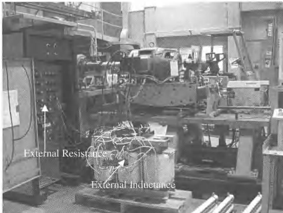
*Fig. 3.33: Configuration of External Impedance into the Rotor Circuit*
