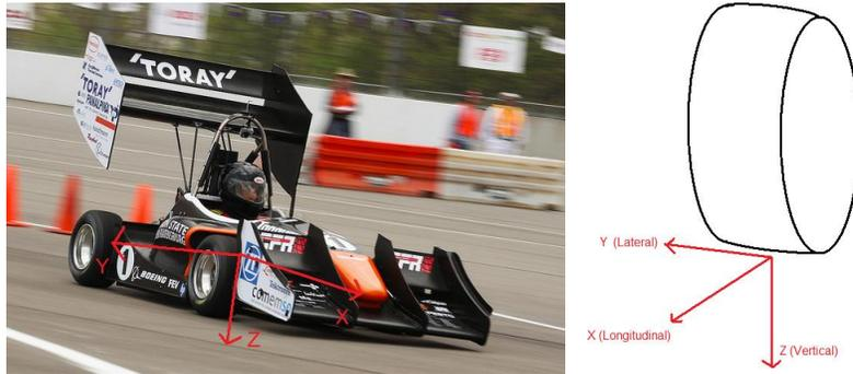
FIGURE 1.3: Vehicle and tire axis systems. Photo credit: Robert Story
