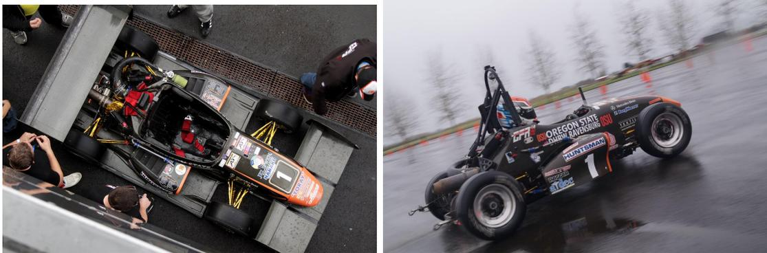
FIGURE 2.6: GFR11c with and without aerodynamic elements, At left at FS Austria 2011, at right during Round 1 damper testing. The gold color on suspension links is heat shielding for the strain gauges on the links. Photo credit: Robert Story and Jay Swift
