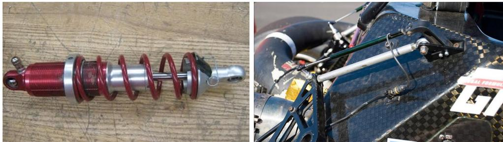
FIGURE 2.9: Penske 7800 damper on left, “Hardlink” installed for rigid damping setup on right. Photo credit: Author, Ankit Agarwal
