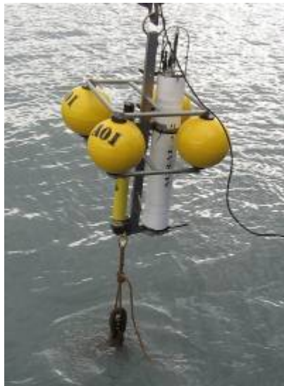
Figure 7. An OBH system, consisting of a hydrophone recording system and an acoustic release, with floats and anchor.
