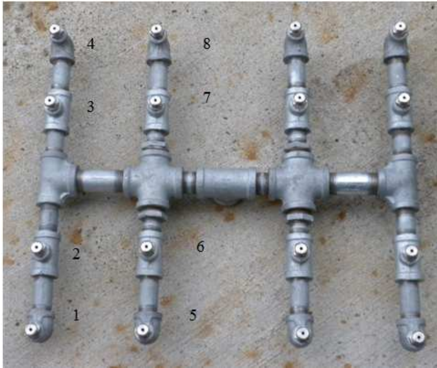
Figure 4: Complete piping network with the numbered nozzles corresponding to the beakers
