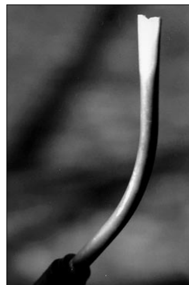
Figure 4.—A new tip can be constructed using a \frac{3}{8} -inch pipe nipple and coupler. Note the end of the nipple has been smashed flat, creating an opening of about \frac{3}{8} inch for the flame. This allows the gas to burn cool with no aeration. Remove the end of the weed burner and attach the new tip to the end of the torch.
