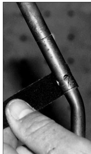
Figure 3.—Taping the tip excludes air and maintains a cooler flame.
