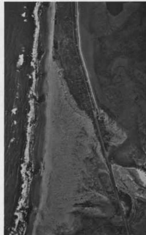
Figure 11.—In 1956 a dike was completed between Pitcher Point and Bayocean township. The map and aerial photo show where the breach occurred and illustrate how the dike has altered the natural erosion patterns. The arrow on the map shows the breach; see figure 10. Note how sand has built up seaward of the dike in the region where the breach happened. (The map is reproduced from chart C&GS 6112/NOS 18162.)
