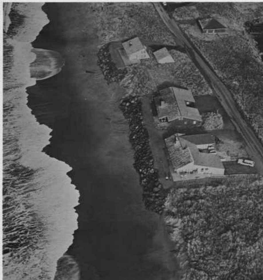
Figure 1.—European dune grass sown on Siletz Spit stabilizes the sand dunes. Nonetheless, the coastline changes. Homes on the spit are vulnerable to high tides and storm waves. Attempting to defeat natural processes that continually alter the coastline, homeowners have placed riprap—large rocks—along their seaward boundaries. The resultant slowing of erosion shows in the contrast between the prominence of the protected homesites and the receding dunes on the adjacent vacant land.
