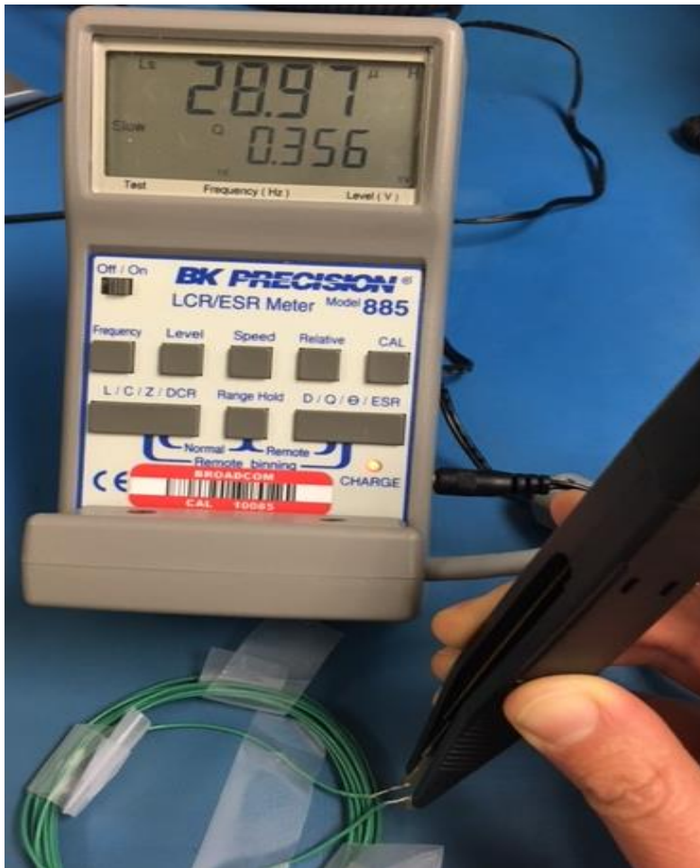
Figure 4-3: Measurement of the self-inductance of the coil with an LCR meter
