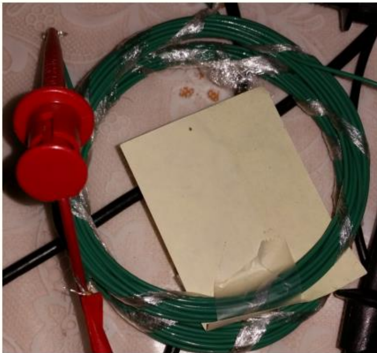
Figure 4-1 Hand-wrapped transmitter and receiver coils
