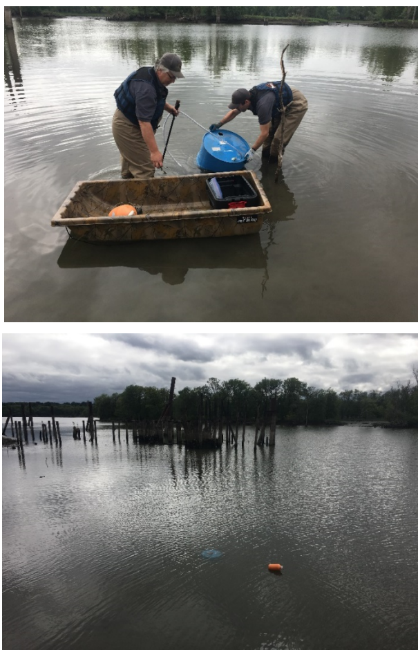
Figure 5.1. Deployment of half-barrel seepage meters at a creosote contaminated site in St. Helens, Oregon. When paired with passive sampling devices to measure concentrations of contaminants in the sediment porewater, the seepage meters can be used to determine the advective flux of contaminants.
