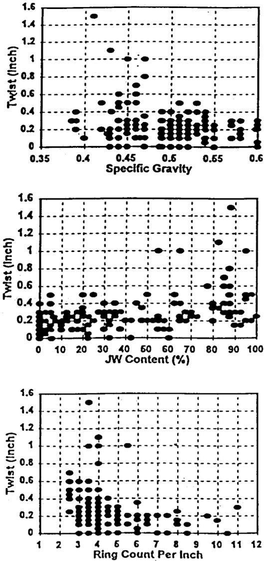
FIGURE 3. Twist as a function of wood growth properties. a) specific gravity, b) juvenile wood (JW) content, and c) ring count.
