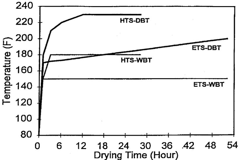
FIGURE 1. Kiln schedules used in the study. ETS: elevated temperature schedule; HTS: high-temperature schedule; DBT: dry bulb temperature; WBT: wet bulb temperature.
