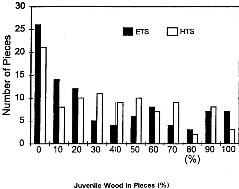
FIGURE 2. Distribution of juvenile wood content in the test lumber dried with elevated temperature schedule (ETS) and high-temperature schedule (HTS).
