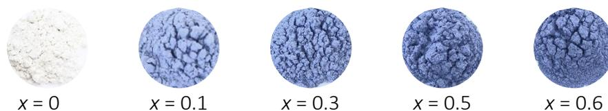
**Figure 3.4.** Color pictures of the synthesized  $\text{Sr}_2\text{Zn}_{1-x}\text{Ni}_x\text{Ge}_2\text{O}_7$  solid solution at different  $x$  values.
