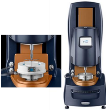
Figure 7. The DHR and zoomed in configuration with the double wall Couette [23].
