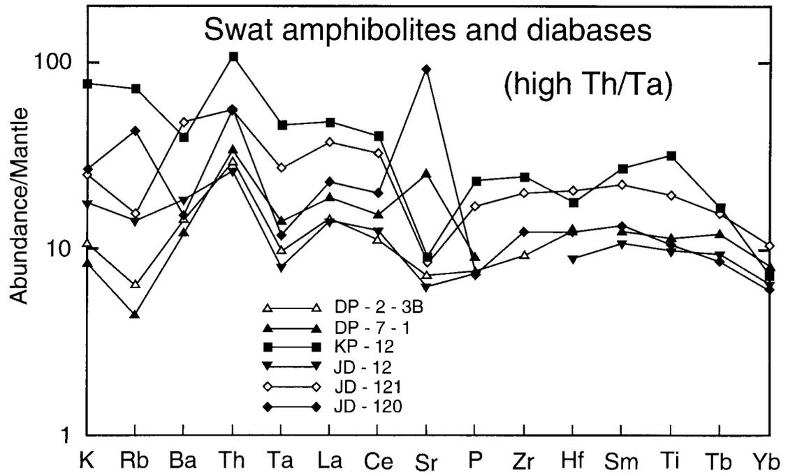
Figure II.6 - Multi-element plots of Swat and Peshawar basin amphibolites and diabases having high Th/Ta ratios, shown normalized to Earth mantle abundances (Taylor and McClennan, 1985).
