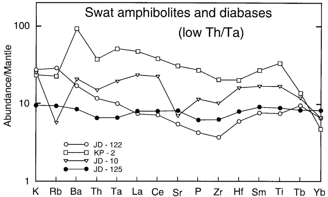
Figure II.5 - Multi-element plots of Swat and Peshawar basin amphibolites and diabases having low Th/Ta ratios, shown normalized to Earth mantle abundances (Taylor and McClelland, 1985).
