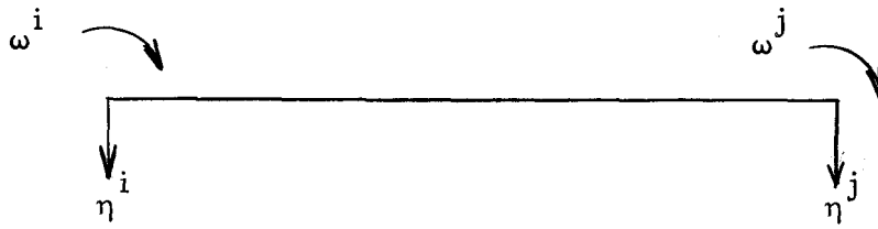
(a) Sign convention for member displacements. Directions as shown are considered positive.
